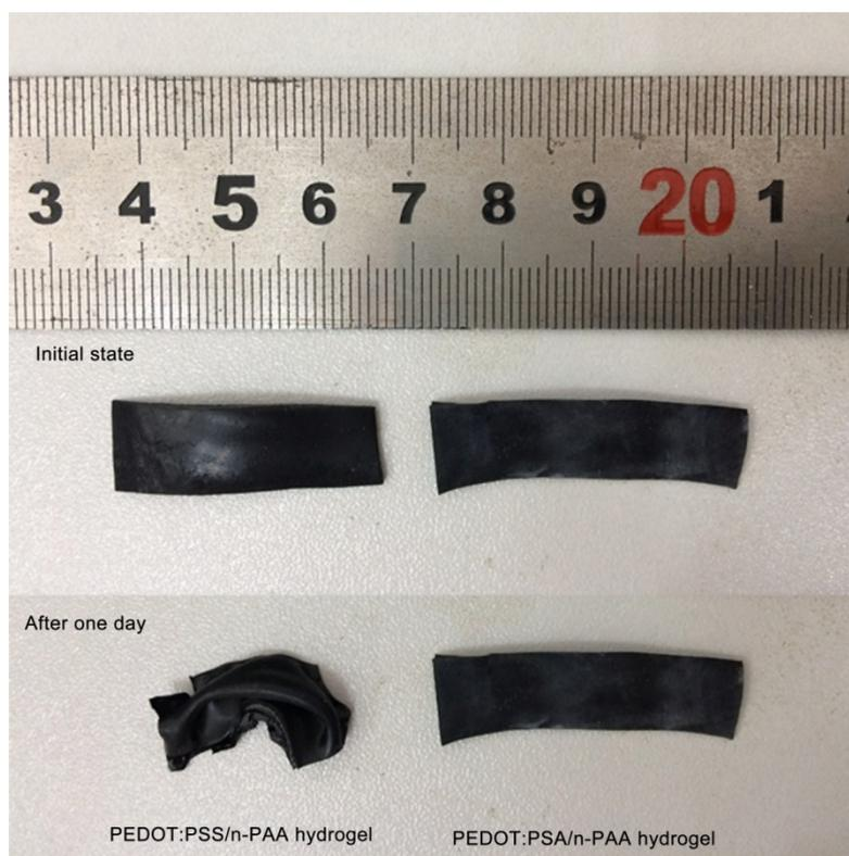
Fig. S7 Photographs of the PEDOT: PSS/n-PAA hydrogel and PEDOT: PSA/n-PAA hydrogel
