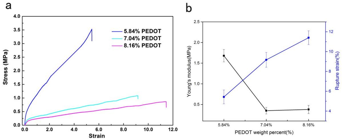
Fig.S4 Stretch-insensitive behavior of resistance for PEDOT: PSS/n-PAA hydrogels. a) Stress-strain curves for the PEDOT: PSS/n-PAA hydrogels for different weight ratios of PEDOT: PSS. b)
