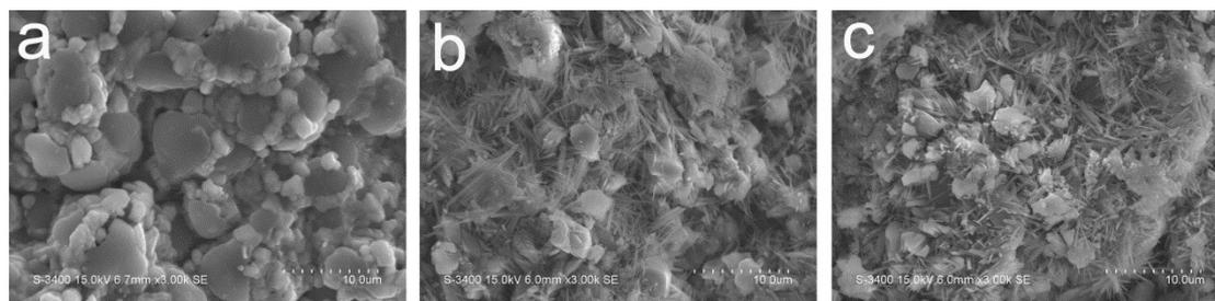
Fig.S3 SEM images of the PEDOT section of the PEDOT: PSS/n-PAA hydrogels include a) 5.84 wt% PEDOT, b) 7.04 wt% PEDOT, c) 8.16 wt% PEDOT, respectively.
