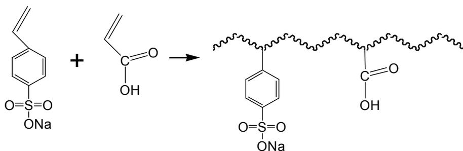
Fig. S2 Fabrication process of PSA copolymers
