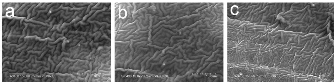
Fig.S5 SEM images of PEDOT: PSA/n-PAA hydrogels after tensile cycles. (a) 1th. (b) 500th. (c)
