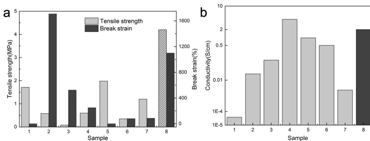
Fig.S1 Comparison of comprehensive properties of conducting hydrogels with other recently
