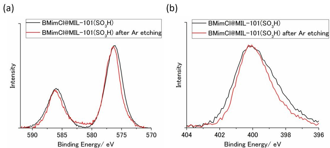
**Fig. S8.** XPS spectra of BMimCl@MIL-101(SO<sub>3</sub>H) before and after Ar ion-beam etching. Close-up peaks of (a) Cr 2p and (b) N 1s.
