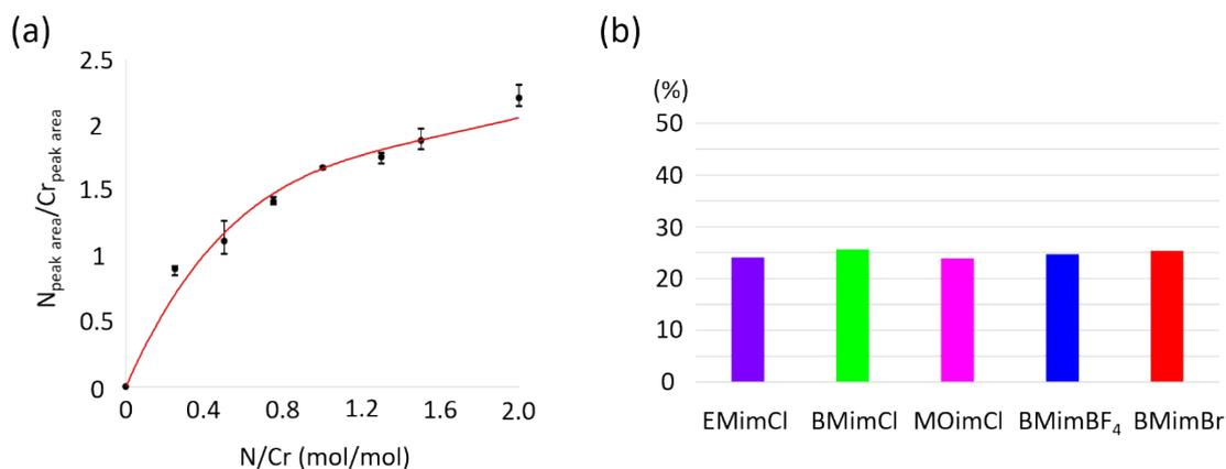
**Fig. S3.** (a) The calibration curve generated from XPS measurements with the standard samples obtained by controlled mixing of MIL-101 and BMimCl. The y axis corresponds to the peak area ratios ( $N/Cr$ ) obtained from XPS measurements. The x axis corresponds to the actual molar ratios in the samples. (b) Percentage of  $SO_3H$  groups in MIL-101( $SO_3H$ ) showing the ion-exchange reactions with corresponding ILs.
