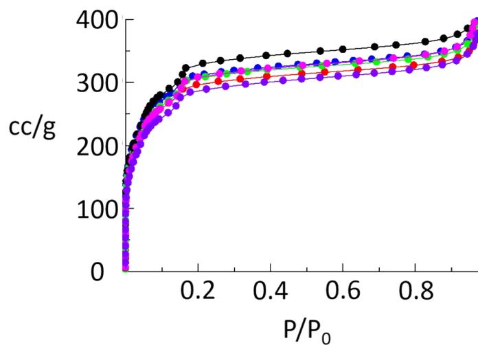
**Fig. S4.** N<sub>2</sub> adsorption isotherms at 77 K of ILs@MIL-101(SO<sub>3</sub>H). black line: MIL-101(SO<sub>3</sub>H); blue line: EMimCl@MIL-101(SO<sub>3</sub>H); red line: BMimCl@MIL-101(SO<sub>3</sub>H); purple line: MOimCl@MIL-101(SO<sub>3</sub>H); pink line: BMimBF<sub>4</sub>@MIL-101(SO<sub>3</sub>H); light green line: BMimBr@MIL-101(SO<sub>3</sub>H).
