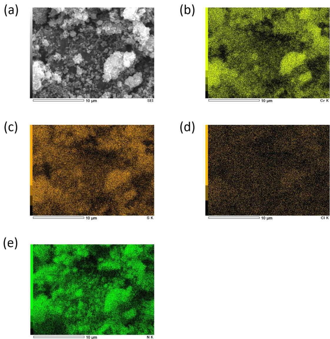
**Fig. S2.** (a) SEM image of BMimCl@MIL-101(SO<sub>3</sub>H), EDX mapping of (b) Cr, (c) S and (d) Cl elements of BMimCl@MIL-101(SO<sub>3</sub>H).
