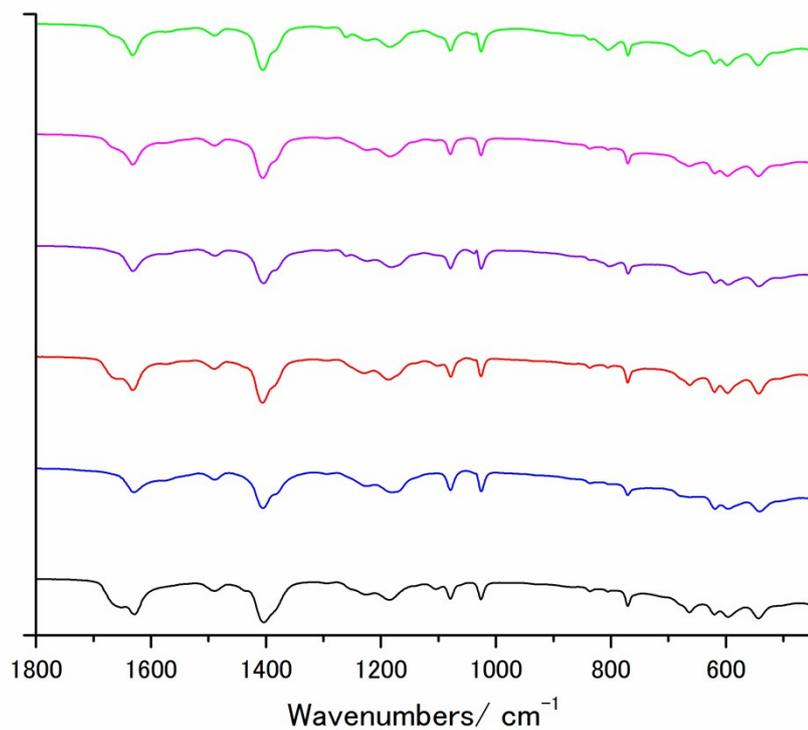
**Fig. S1.** IR spectra of MIL-101(SO<sub>3</sub>H) and ILs@MIL-101(SO<sub>3</sub>H). black line: MIL-101(SO<sub>3</sub>H); blue line: EMimCl@MIL-101(SO<sub>3</sub>H); red line: BMimCl@MIL-101(SO<sub>3</sub>H); purple line: MOimCl@MIL-101(SO<sub>3</sub>H); pink line: BMimBF<sub>4</sub>@MIL-101(SO<sub>3</sub>H); light green line: BMimBr@MIL-101(SO<sub>3</sub>H).
