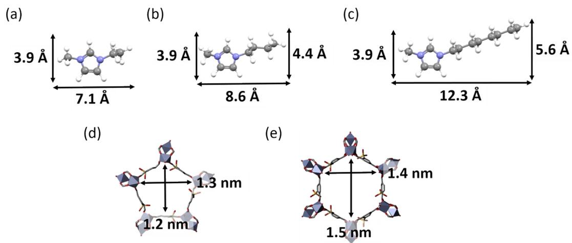
**Fig. S7.** Molecular sizes of (a) EMimCl, (b) BMimCl and (c) MOimCl. (d)(e) Pore window sizes of MIL-101(SO<sub>3</sub>H).
