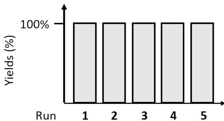
**Fig. S5.** The progress of the reaction yields of poly(propylene oxide) along with the repeated usages of BMimCl@MIL-101(SO<sub>3</sub>H) as catalyst.
