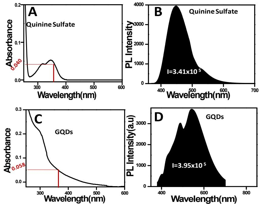
**Figure ESI2** A) UV-Vis spectra of quinine sulfate B) Integrated photoluminescence intensity of quinine sulfate C) UV-Vis spectra of GQDs and D) integrated photoluminescence intensity of GQDs
