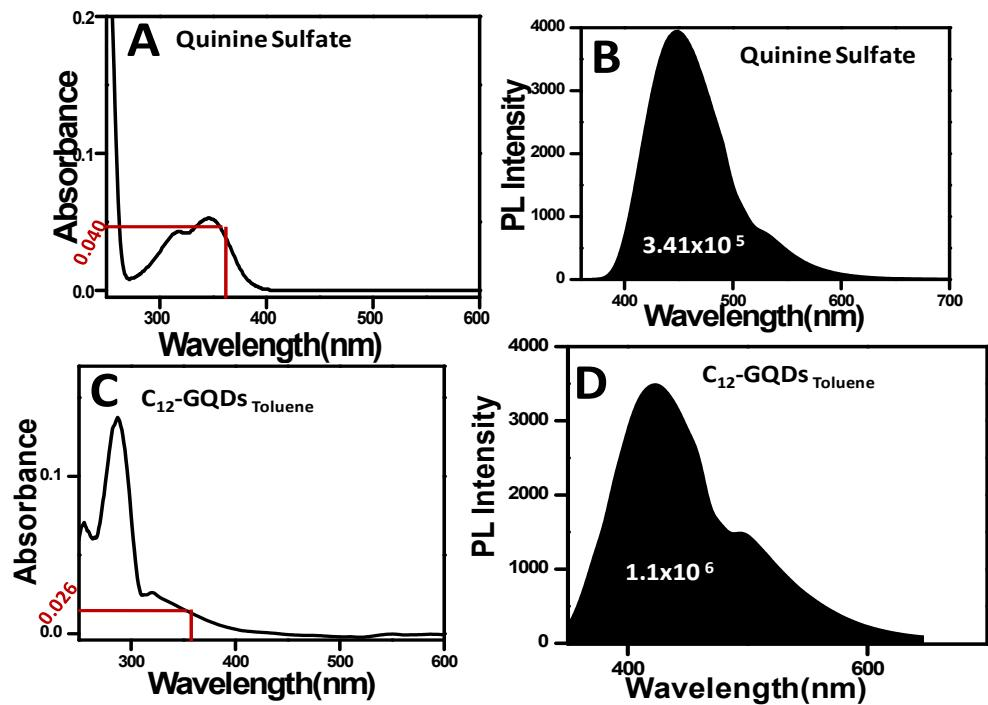
**Figure ESI4** A) UV-Vis spectra of quinine sulfate B) integrated photoluminescence intensity of quinine sulfate C) UV-Vis spectra of  $C_{12}$ -GQDs <sub>Toluene</sub> and D) integrated photoluminescence intensity of  $C_{12}$ -GQDs <sub>Toluene</sub>
