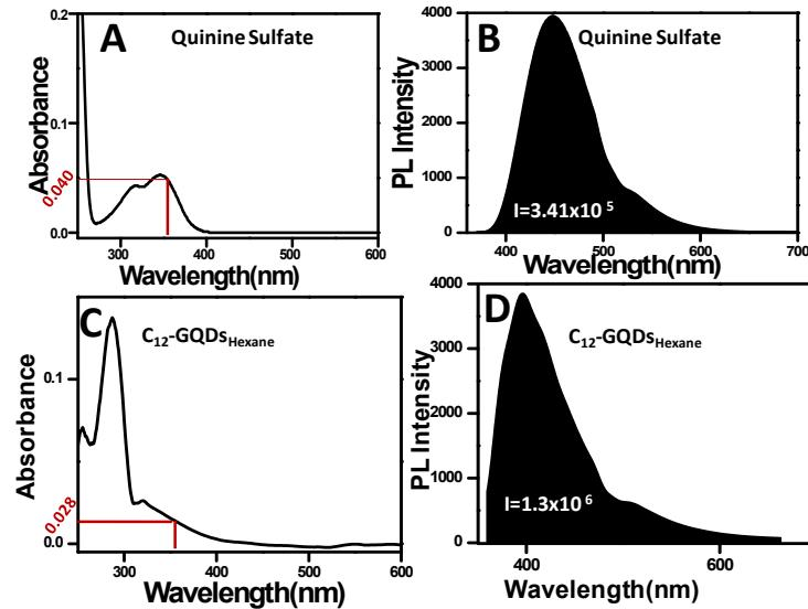
**Figure ESI3** A) UV-Vis spectra of quinine Sulfate B) integrated photoluminescence intensity of quinine sulfate C) UV-Vis spectra of  $C_{12}$ -GQDs<sub>Hexane</sub> and D) integrated photoluminescence intensity of  $C_{12}$ -GQDs<sub>Hexane</sub>
