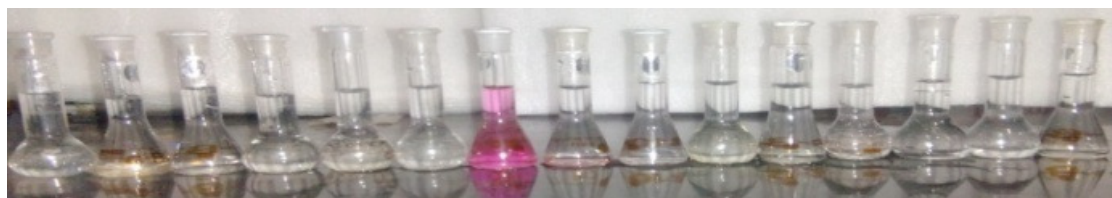
Fig. S2: Photograph of change in colour of the solution of 1 in EtOH–H 2 O (1:1 v/v, 0.1M PBS) medium on addition of various metal ions; added metal ions (from left to right: blank, Na(I), K(I), Ca(II), Mn(II), Fe(II), Fe(III), Co(II), Ni(II), Cu(II), Zn(II), Ag(I), Cd(II), Hg(II) and Pb(II)).
