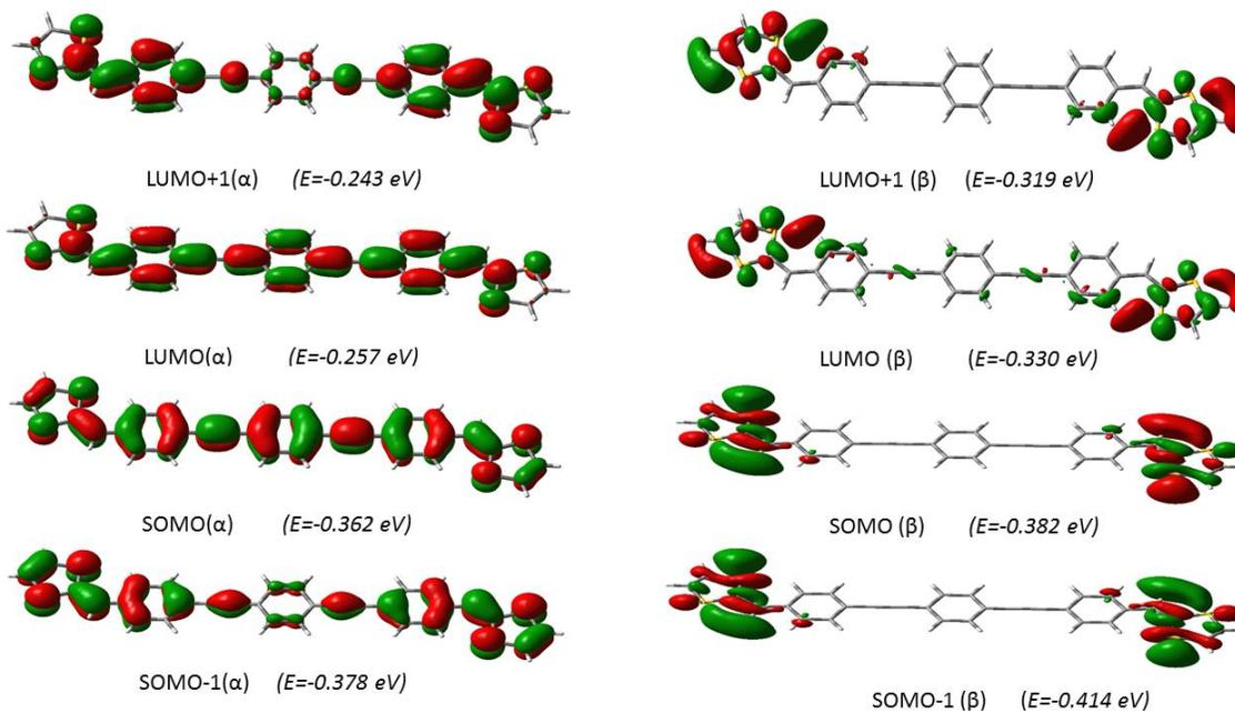
**Fig. S-2.** Contours of frontier MOs for compound **1b** in the triplet dication state and their eigenvalues calculated at the B3LYP/6-31++G (d,p) level.
