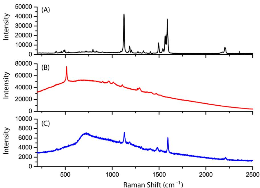
**Fig. S-8.** Raman spectra of the solid thin film of **1a** on a glass substrate measured (A) before exposure to iodine vapour, (B) after exposure to iodine vapour for 65 min, and (C) after being left in open air for two weeks.
