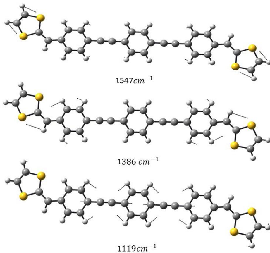
**Figure S-7.** Raman active vibrational vectors for compound **1b** in the dication singlet state calculated at the B3LYP/6-31++G(d,p) level.
