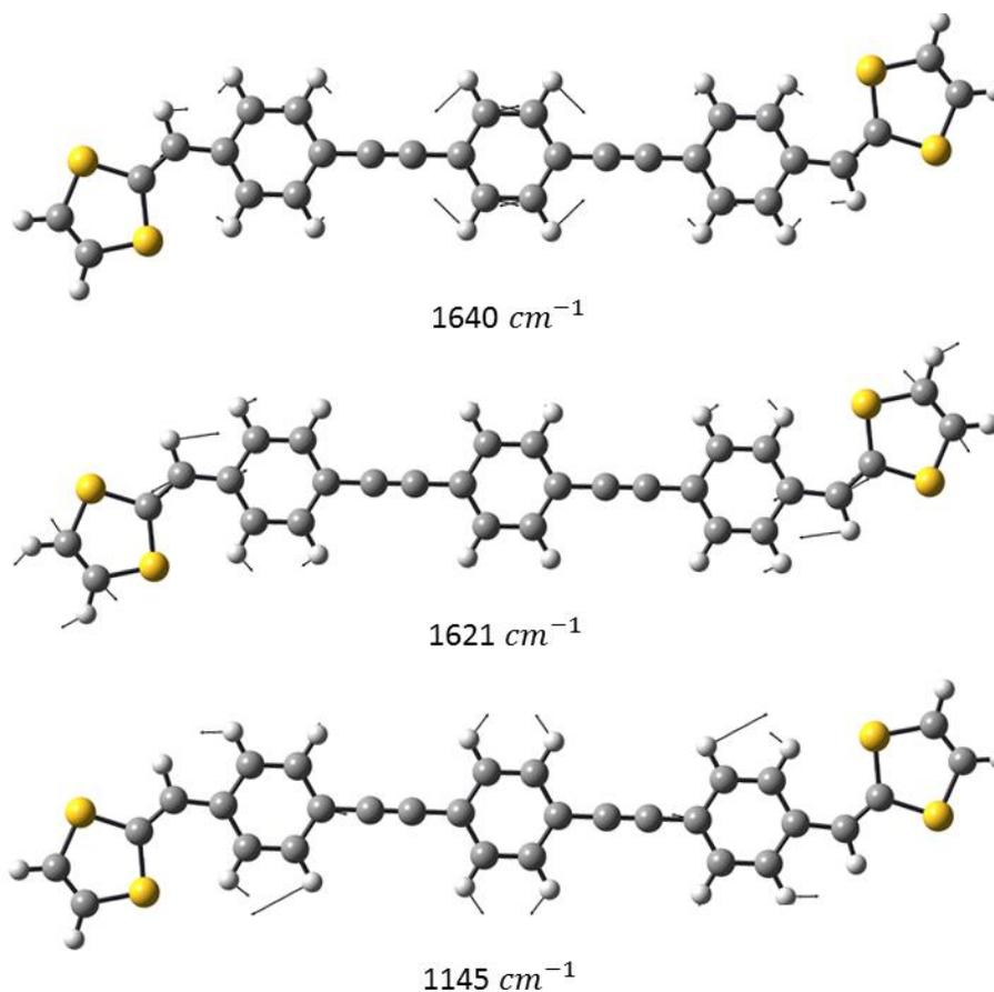
**Fig. S-4.** Raman active vibrational vectors for compound **1b** in the neutral state calculated at the B3LYP/6-31++G(d,p) level.
