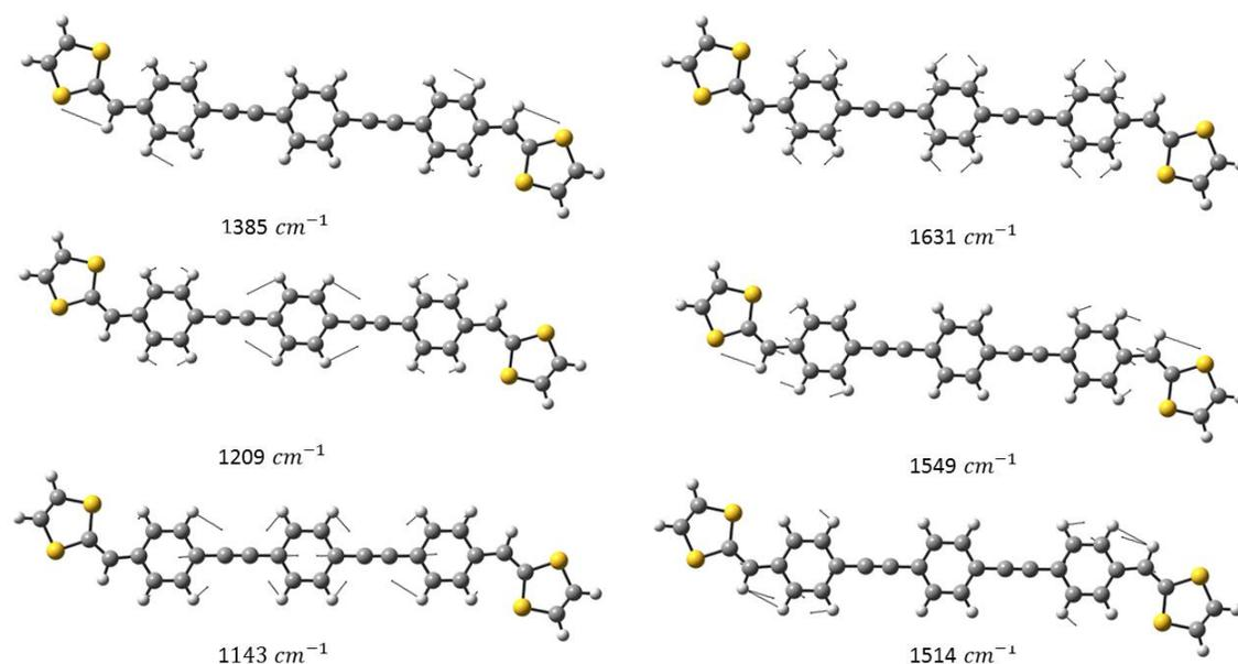
**Fig. S-6.** Raman active vibrational vectors for compound **1b** in the dication triplet state calculated at the B3LYP/6-31++G(d,p) level.
