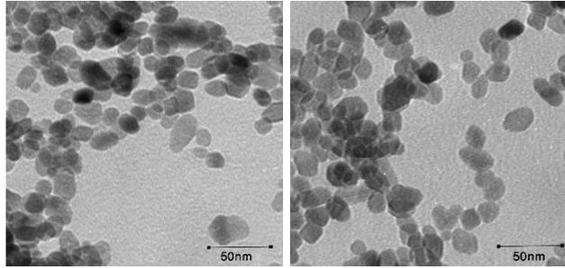
**Figure S3.** TEM images of TiO<sub>2</sub>-AA-Co nanohybrid
