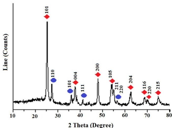
**Figure S1.** XRD pattern of nano TiO<sub>2</sub> ◆ (Anatase) ● (Rutile)
