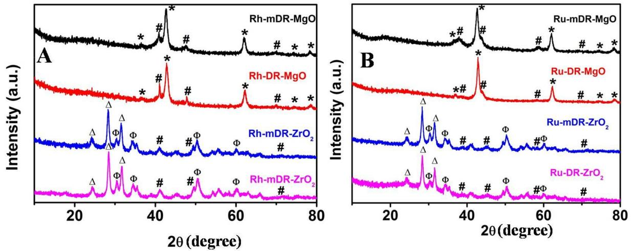
**Figure S1:** XRD pattern for (A) Rh, (B) Ru nanoparticles prepared by traditional and modified digestive ripening and anchored on MgO and ZrO<sub>2</sub> support. JCPs No and Crystallographic phase: Rh (Cubic 88-2334), Ru (Hexagonal 70-0274), MgO (Cubic 78-0430) and ZrO<sub>2</sub> (Monoclinic 89-9066 and Tetragonal 89-9068)
