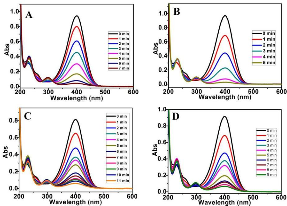
**Figure S5:** UV-vis spectra for PNP reduction reaction catalysed by (A) Rh-MgO-mDR, (B) Rh-MgO-DR, (C) Rh-ZrO-mDR and (D) Rh-ZrO-DR catalysts.
