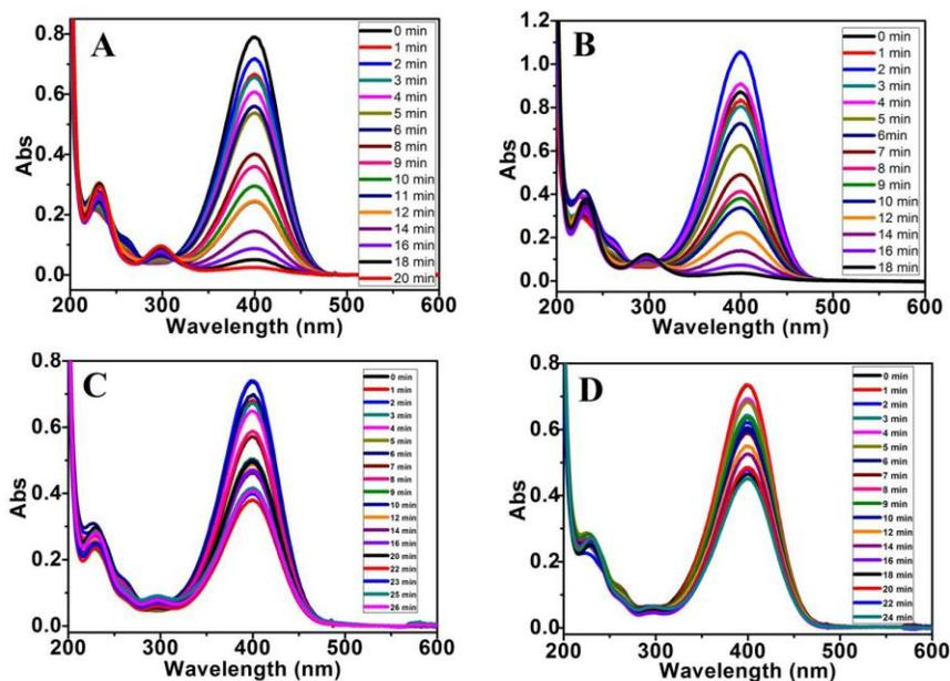
**Figure S6:** UV-vis spectra for PNP reduction reaction catalysed by (A) Ru-MgO-mDR, (B) Ru-MgO-DR, (C) Ru-ZrO-mDR and (D) Ru-ZrO-DR catalysts.
