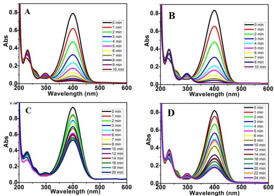
**Figure S4:** UV-vis spectra for PNP reduction reaction catalysed by (A) Pt-MgO-mDR, (B) Pt-MgO-DR, (C) Pt-ZrO-mDR and (D) Pt-ZrO-DR catalysts.
