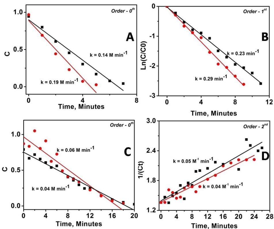
**FigureS9:** Kinetic fitting of p-nitro phenol reduction reaction into various rate law equations. In presence of (A) Rh-mDR-MgO (black), and Rh-DR-MgO (red), (B) Rh-mDR-ZrO<sub>2</sub> (black) and Rh-DR-ZrO<sub>2</sub> (red) catalysts; (C) Ru-mDR-MgO (black), and Ru-DR-MgO (red), and (D) Ru-mDR-ZrO<sub>2</sub> (black) and Ru-DR-ZrO<sub>2</sub> (red) catalysts.
