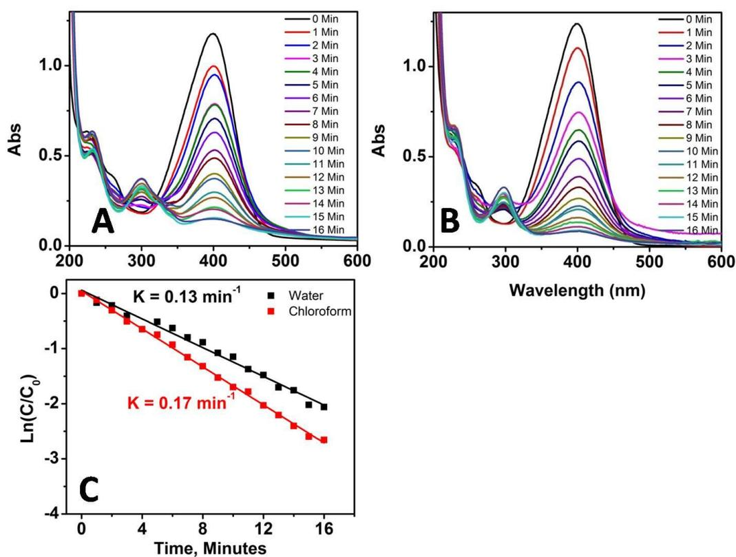
**Figure S8:** UV-Visible spectra of borohydride assisted PNP reduction using Pd-DR-MgO (un-annealed) as catalyst. (A) in absence and (B) in presence of 1 mL chloroform. (C) Fitting of concentration data (obtained from A and B) into first order rate constant equation.
