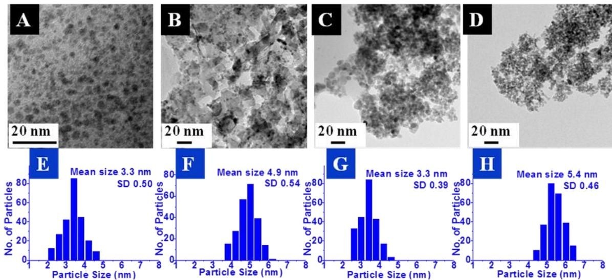
**Figure S2:** upper panel: TEM images for (A) Rh-MgO-mDR, (B) Rh-MgO-DR, (C) Rh-ZrO-mDR and (D) Rh-ZrO-DR particles; lower panel: particle size distribution histogram for (E) Rh-MgO-mDR, (F) Rh-MgO-DR, (G) Rh-ZrO-mDR and (H) Rh-ZrO-DR particles.
