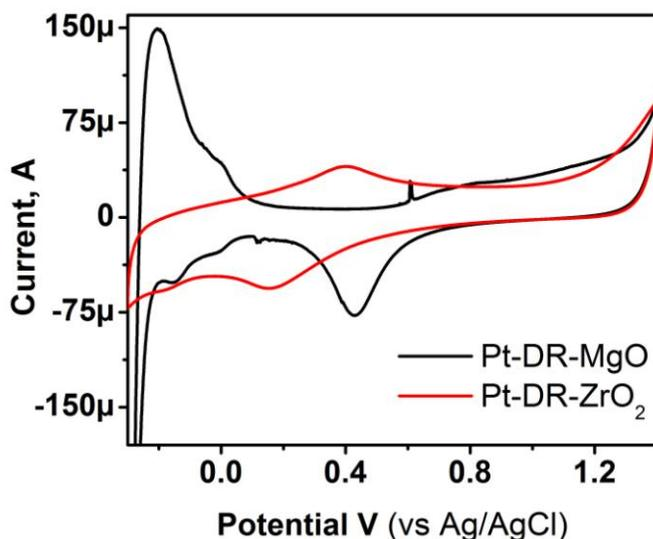
*Figure S11: CVs recorded for MgO (Black) and ZrO<sub>2</sub> (Red) supported Pt nanoparticles prepared by traditional digestive ripening (DR). Material was deposited on glassy Carbon electrode and CVs were recorded in 0.5 M H<sub>2</sub>SO<sub>4</sub> solution. Scan rate: 50 mV/s.*
