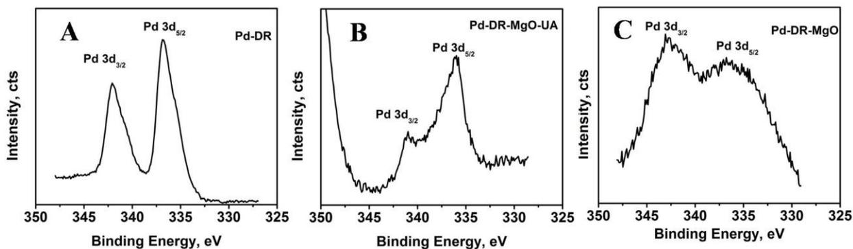
*Figure S10: Pd 3d XPS spectra of (A) unsupported and (B) MgO supported un-annealed and (C) MgO supported (Pd-DR-MgO) Pd nanoparticles.*
