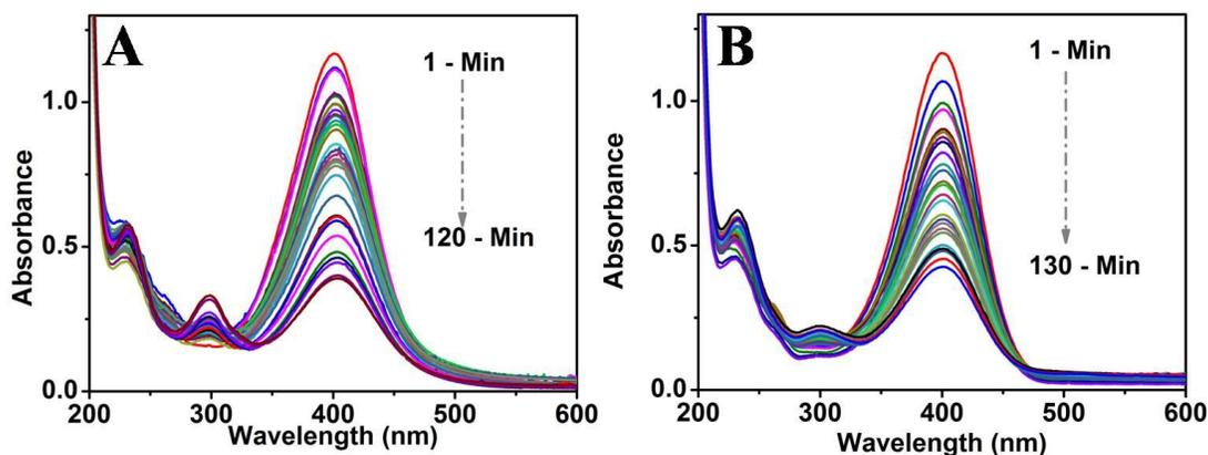
*Figure S7: UV-vis spectra for recorded NaBH<sub>4</sub> assisted PNP reduction in presence (A) and absence (B) of MgO.*
