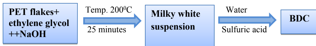
Scheme S1: Depolymerization of PET to BDC via alkaline hydrolysis
