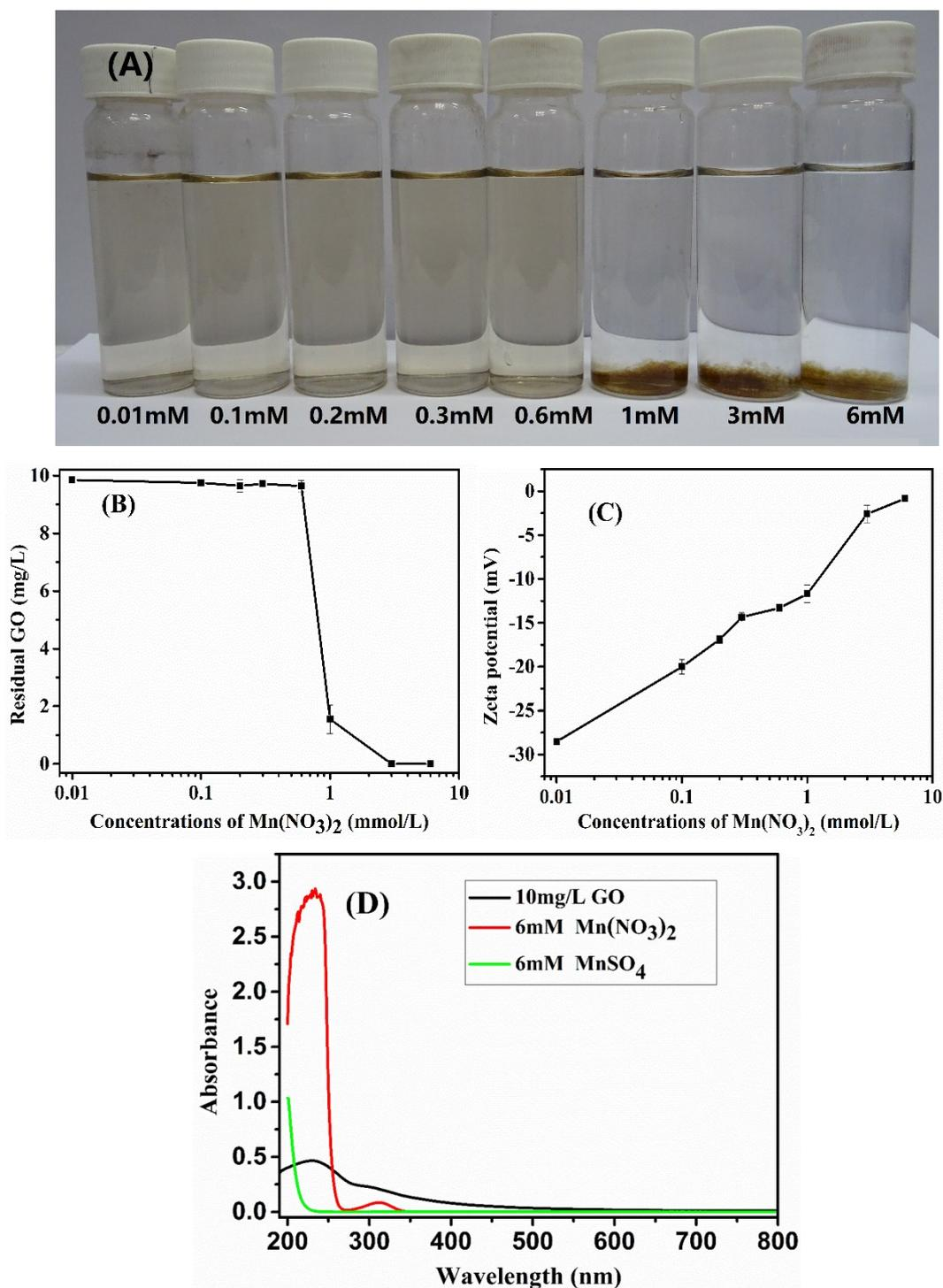
**Fig. S3** (A) Optical images of GO in the presence of different  $\text{Mn}(\text{NO}_3)_2$  concentration. (B) Concentrations of the residual of GO in the supernatant as a function of  $\text{Mn}(\text{NO}_3)_2$  concentration. (C) Zeta potentials of GO as a function of  $\text{Mn}(\text{NO}_3)_2$  concentration. (D) Wavelength scanning spectra of GO,  $\text{Mn}(\text{NO}_3)_2$  and  $\text{MnSO}_4$ ,  $\text{pH}=7.0\pm 0.1$ ,  $C_{(\text{GO})\text{initial}}=10 \text{ mg/L}$ .
