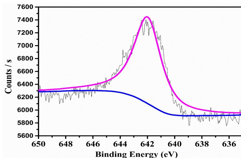
Fig. S7 XPS pattern of GO /manganese aggregates at pH
