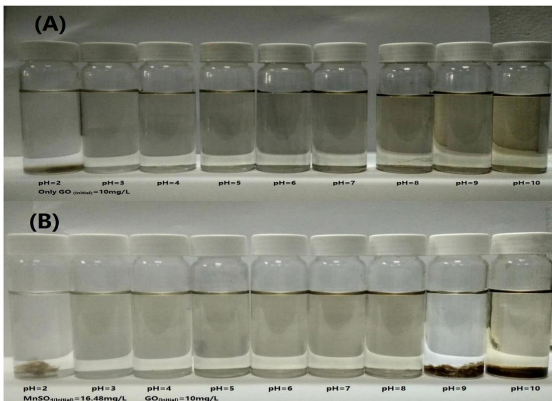
**Fig. S4** (A) Optical images of only GO at different pH conditions. (B) Optical images of GO with addition 0.3 mM Mn(II) at different pH conditions,  $I=0.005$  mol/L NaCl (NaCl was served as an electrolyte in order to adjusting pH of solution)
