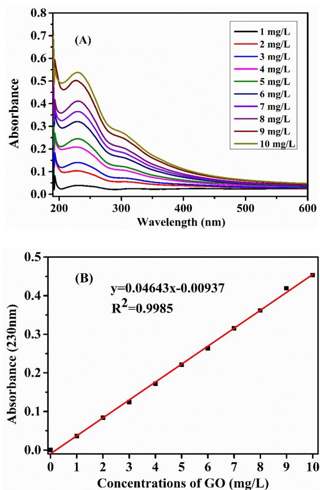
**Fig. S2** UV-Vis absorption spectra of GO and standard curve at absorbance of 230 nm.
