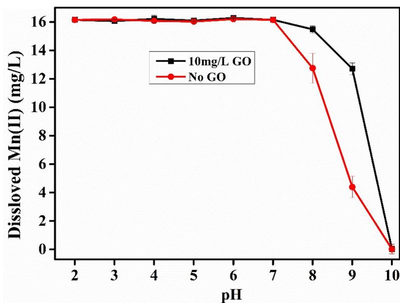
**Fig. S5** Dissolved manganese in the presence and absence of GO in the supernatant.  $C_{(GO)initial}=10$  mg/L,  $C_{(Mn)initial}=0.3$  mmol/L,  $DO=8.0 \pm 0.3$  mg/L.
