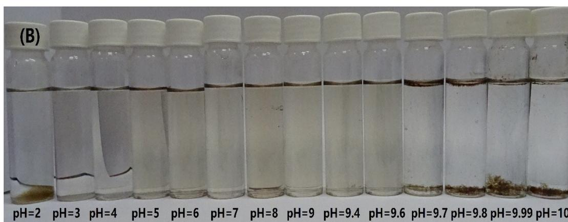
**Fig. S6** (A) Dissolved manganese at different pH conditions. (B) Optical images of residual GO at different pH conditions in anoxic conditions.  $C_{(\text{GO})\text{initial}}=10$  mg/L,  $C_{(\text{Mn})\text{initial}}=0.3$  mM. Reactions were carried out under anoxic conditions ( $\text{DO}= 0.12 \pm 0.03\text{mg/L}$ ).
