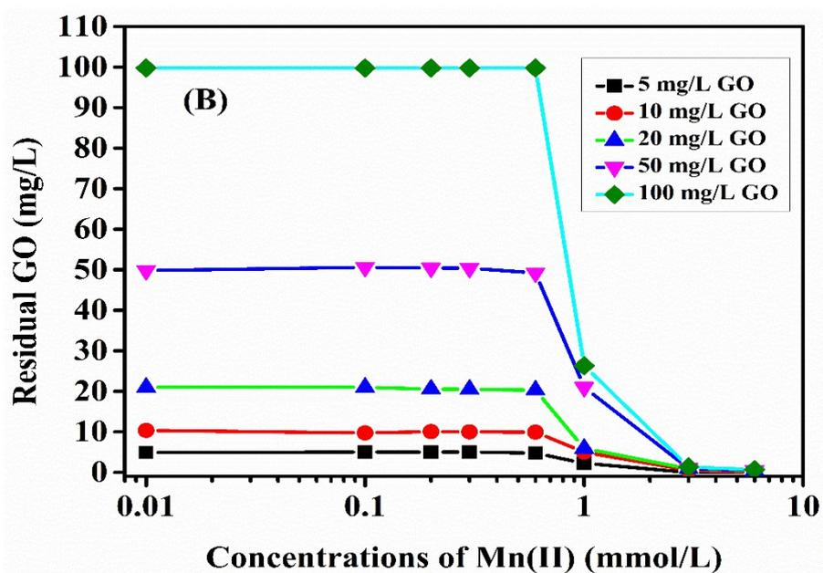
**Fig. S1** (A) Optical images of GO aggregation tests with GO concentration from 5 to 100 mg/L in the presence of different Mn(II) concentration. (B) Concentrations of residual GO flakes in the supernatant as a function of Mn(II) concentration. pH of solution was fixed  $7 \pm 0.1$ .
