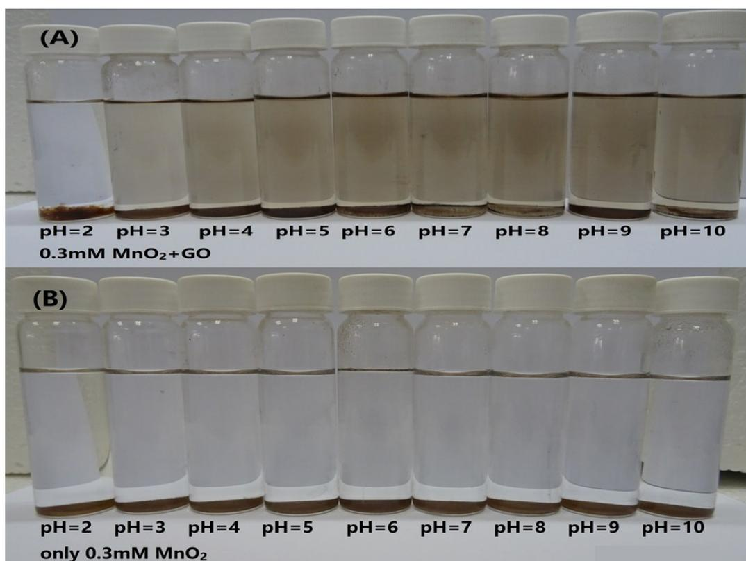
Fig. S8 (A) Optical images of GO with 0.3 mM  $\text{MnO}_2$  in various pH conditions. (B) Only 0.3 mM  $\text{MnO}_2$  at different pH values  $C_{(\text{GO})\text{initial}}=10 \text{ mg/L}$ ,  $C_{(\text{MnO}_2)\text{initial}}=0.3 \text{ mM}$   $I=0.005 \text{ mol/L NaCl}$ . (NaCl was served as an electrolyte in order to adjusting pH of the solutions.)
