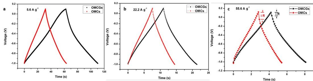
**Fig. S6** Galvanostatic charge/discharge curves of OMCGs (black line) and OMCs (red line) electrodes at current density of (a)  $5.6 \text{ A g}^{-1}$ , (b)  $22.2 \text{ A g}^{-1}$  and (c)  $55.6 \text{ A g}^{-1}$ .
