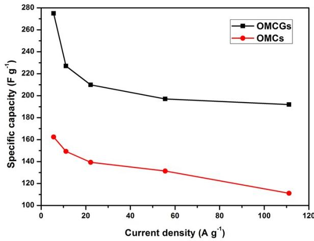
**Fig. S8** Galvanostatic specific capacitance of OMCGs (black line) and OMCs (red line) aganist current density.
