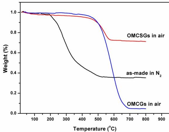
**Fig. S4** TGA curves of OMCSGs in air, as-made in N<sub>2</sub> and OMCGs in air
