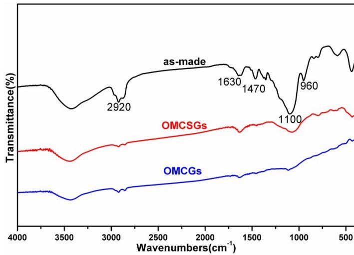
**Fig. S3** FT-IR spectra of (a) as-made, (b) OMCSGs and (c) OMCGs
