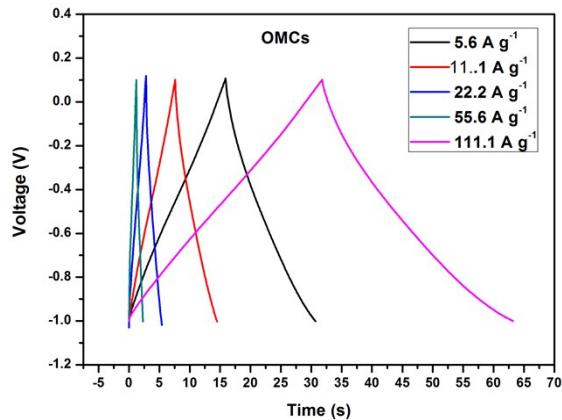
**Fig. S7** Galvanostatic charge/discharge curves of OMCs electrodes at different current density.
