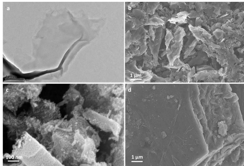
**Fig. S1** (a) TEM image of GO, (b,c) SEM images of OMCGs at different magnifications and (d) SEM image of OMCs.
