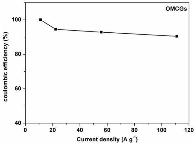
**Fig. S9.** Coulombic efficiency of OMCGs under different current densities.
