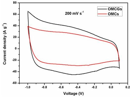
**Fig. S5** Cyclic voltammograms of OMCGs (black line) and OMCs (red line) electrodes at a scan rate of  $200 \text{ mV s}^{-1}$  in  $6.0 \text{ M KOH}$ .
