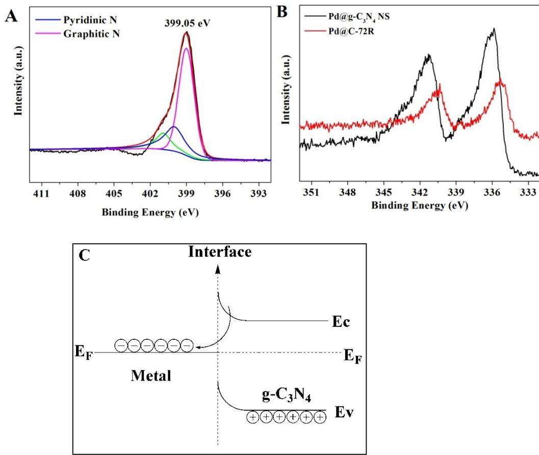
**Fig. S1 Mott-Schottky effect on the catalytic performance of the Pd@g-C<sub>3</sub>N<sub>4</sub> NS catalysts.** (A) N 1s of Pd@g-C<sub>3</sub>N<sub>4</sub> NS, (B) Pd XPS spectra of Pd@g-C<sub>3</sub>N<sub>4</sub> NS and Pd@C-72R and (C) Schematic illustration of Mott-Schottky-type contact of Pd@g-C<sub>3</sub>N<sub>4</sub> NS.
