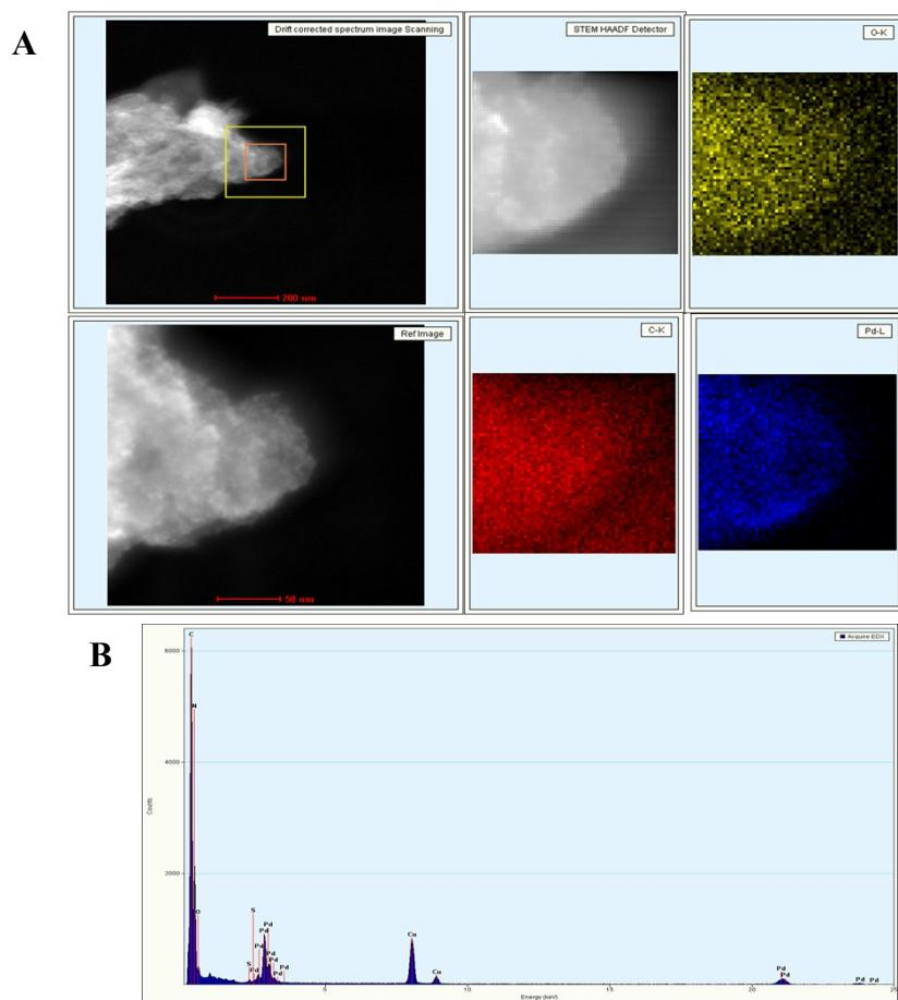
**Fig. S2** The EDX mapping of the synthesized Pd@g-C<sub>3</sub>N<sub>4</sub> NS (A) and EDX image of Pd@g-C<sub>3</sub>N<sub>4</sub> NS (B).
