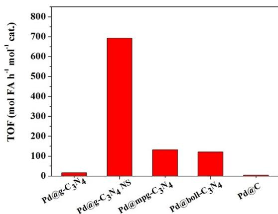
**Fig. S4** TOF values of FA for transfer hydrogenation of nitrobenzene over Pd@g-C<sub>3</sub>N<sub>4</sub>, Pd@g-C<sub>3</sub>N<sub>4</sub> NS, Pd@mpg-C<sub>3</sub>N<sub>4</sub>, Pd@boll-C<sub>3</sub>N<sub>4</sub> and Pd@C (commercially available). Reaction condition: water (5 mL), nitrobenzene (1 mmol), FA (5 mmol), catalyst (2 mg), 25 °C.
