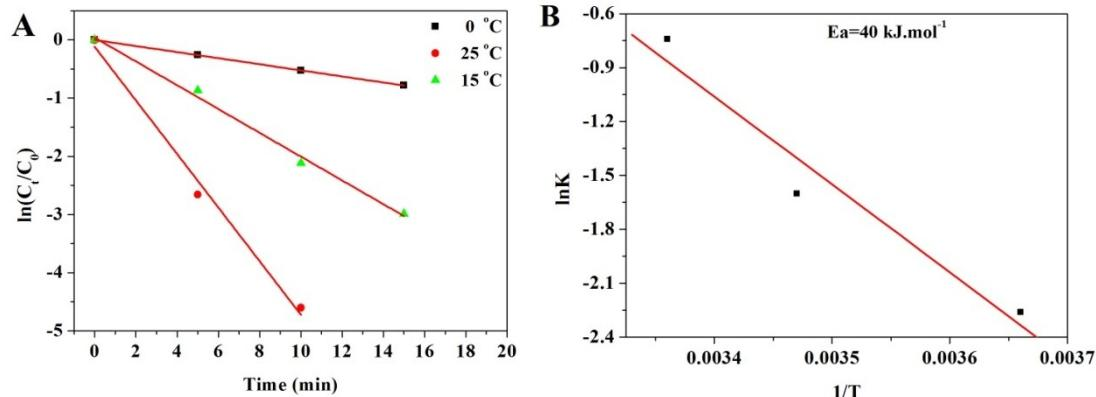
**Fig. S5** The kinetic curves of the catalytic transfer hydrogenation of nitrobenzene at different reaction temperatures. Reaction conditions: nitrobenzene (1 mmol), Pd@g-C<sub>3</sub>N<sub>4</sub> NS (0.155 mol%), water (5 mL), FA (5 mmol).
