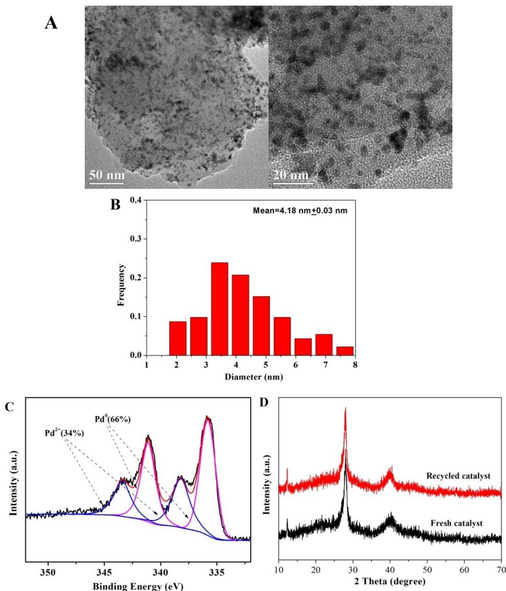
**Fig. S3** TEM images (A), Pd particle-size distribution (B), Pd XPS spectra (C), XRD pattern (D) of recycled catalyst.
