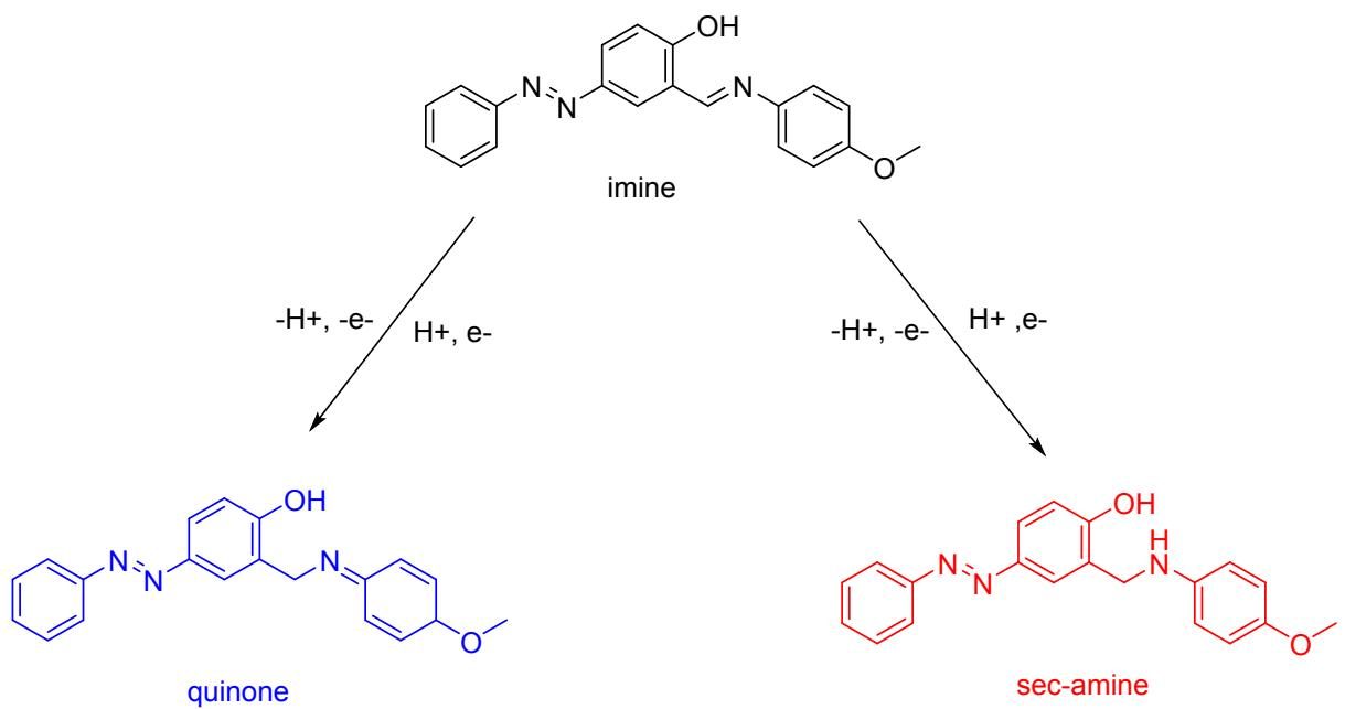
**Fig. S22.** Reversible reduction–oxidation processes of the new azo Schiff base ligands in DMF solution.
