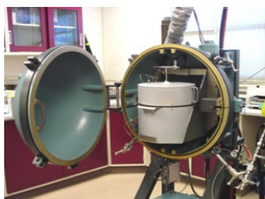
Figure 1. The ARC adiabatic calorimeters used to perform safety experiments using Magpie resins and silver electrolyte effluents.
