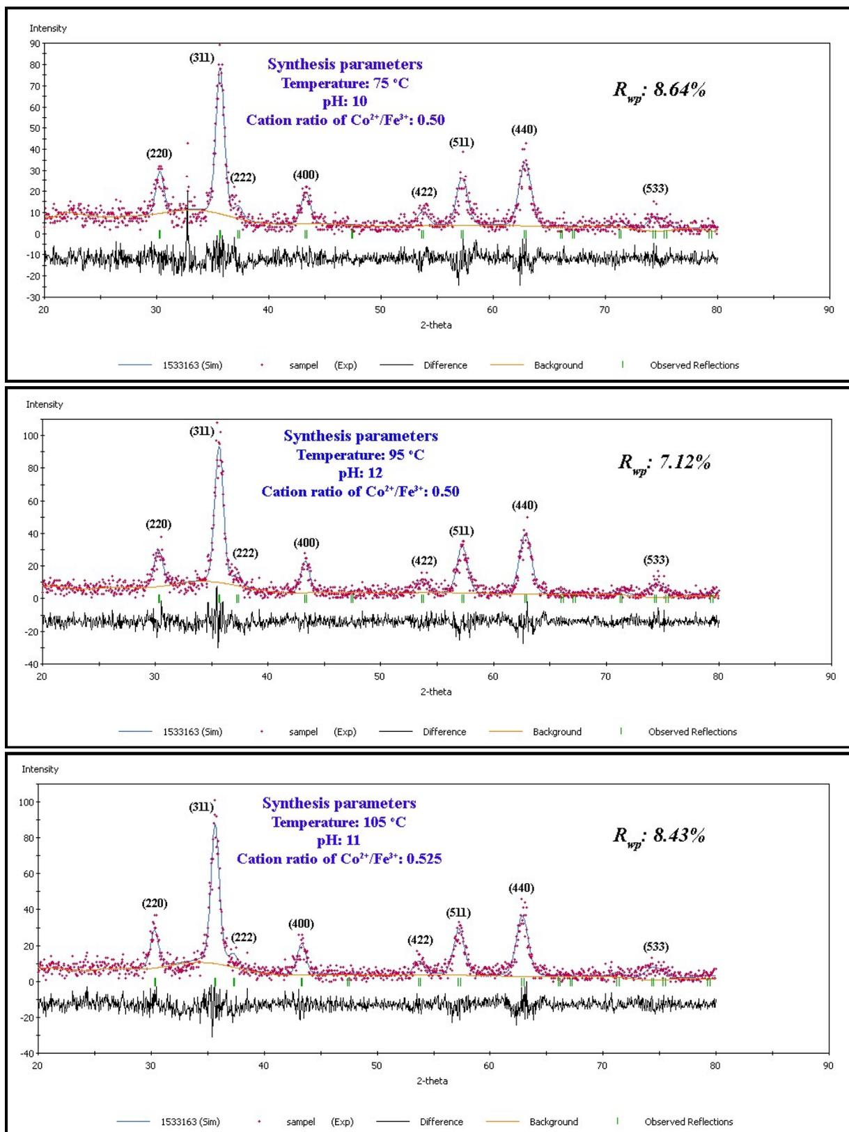
**Fig. S1.** The XRD patterns and corresponding Rietveld structure refinement details of some typical samples with different parameters of synthesis process fitting by Reflex program (CIF#1533163). The values of  $R_{wp}$  factor and synthesis parameters of each sample are presented above of each pattern.
