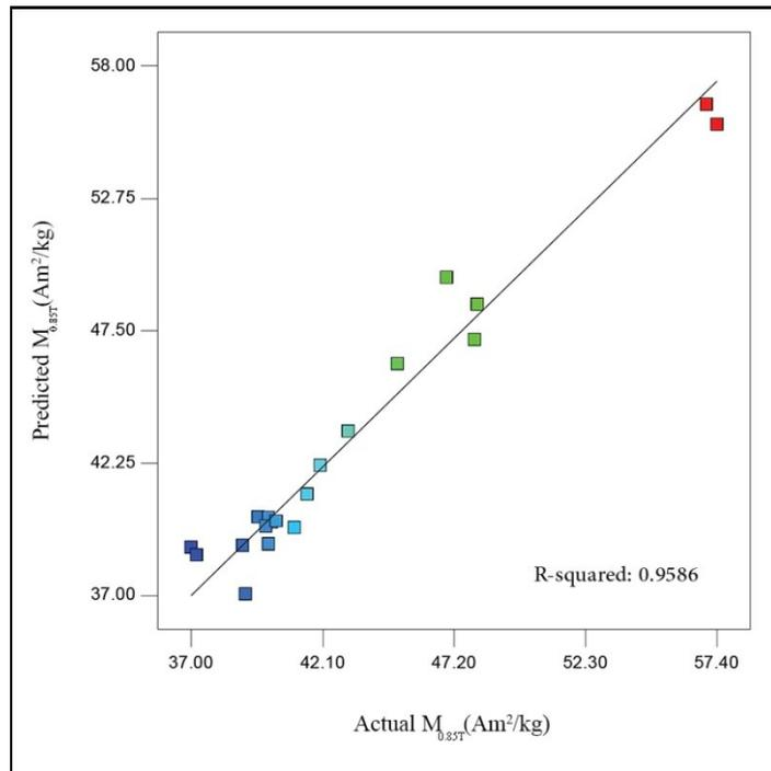
**Fig. S5.** The  $R^2$  graphs for the response of saturation magnetization amount ( $M_{0.85T}$ ).
