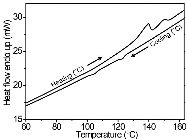
**Figure S5** The DSC trace of compound **5e** on heating and cooling (scan rate 5 °C/min).
