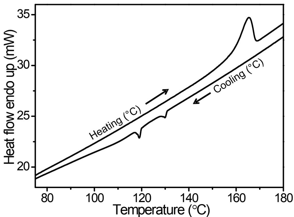
**Figure S4** The DSC trace of compound **5d** on heating and cooling (scan rate 5 °C/min).
