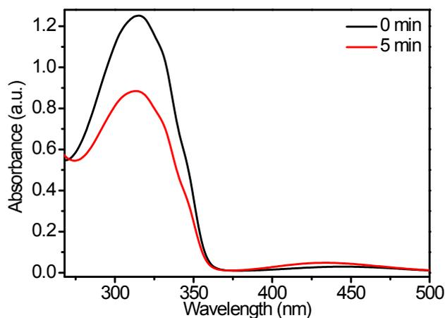
**Figure S7** UV-vis absorption spectra of azobenzenetetracarboxylic acid obtained with respect to time on irradiation at 365 nm wavelength.
