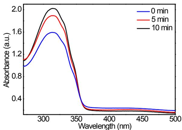
**Figure S6** The UV-vis absorption spectra of compound **5a** obtained with respect to time on exposure to visible light.
