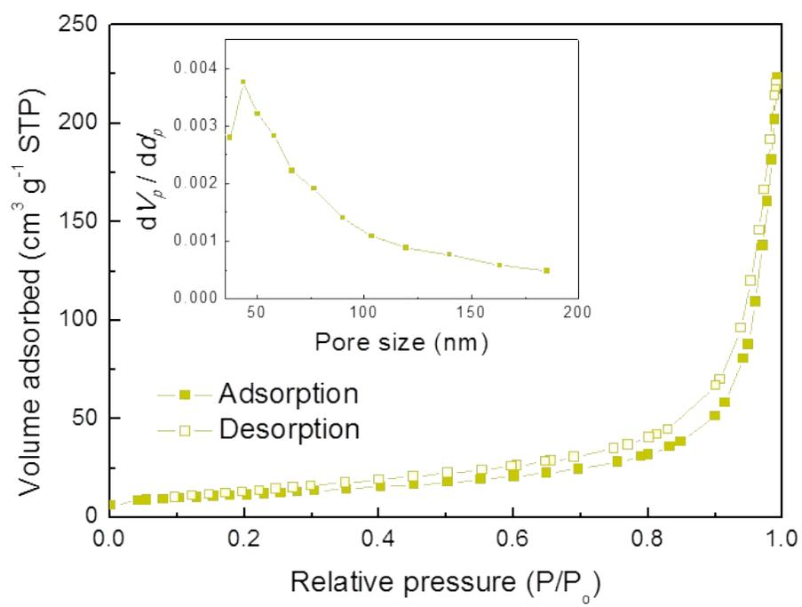
**Fig. S1** Nitrogen adsorption isotherms of 3DOM CFO@60. Inset shows pore size distribution of 3DOM CFO@60.
