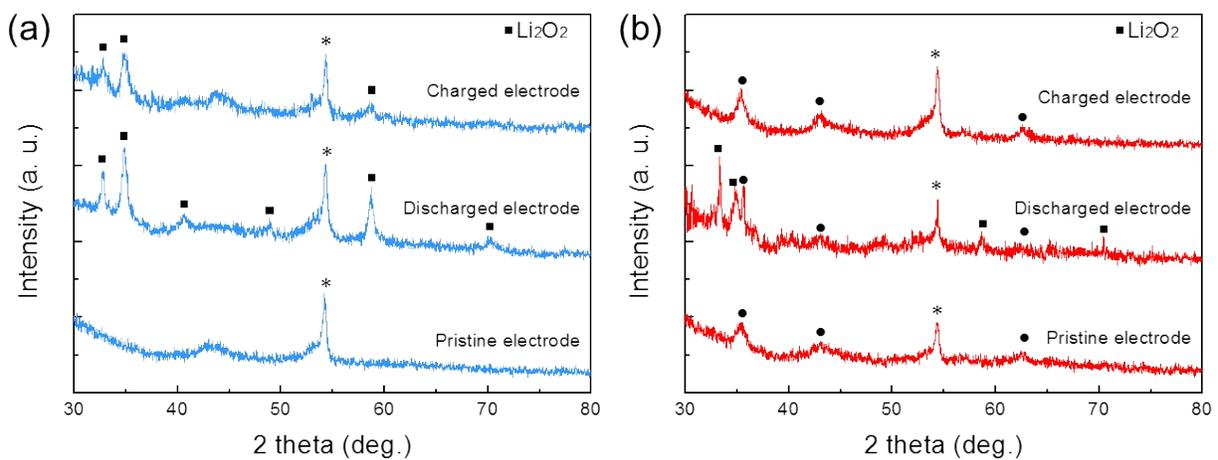
**Fig. S9** XRD patterns of the O<sub>2</sub>-electrodes with (a) KB and (b) CFO@140 at different discharge/charge stages. Peaks marked with asterisks are originated from the carbon paper.
