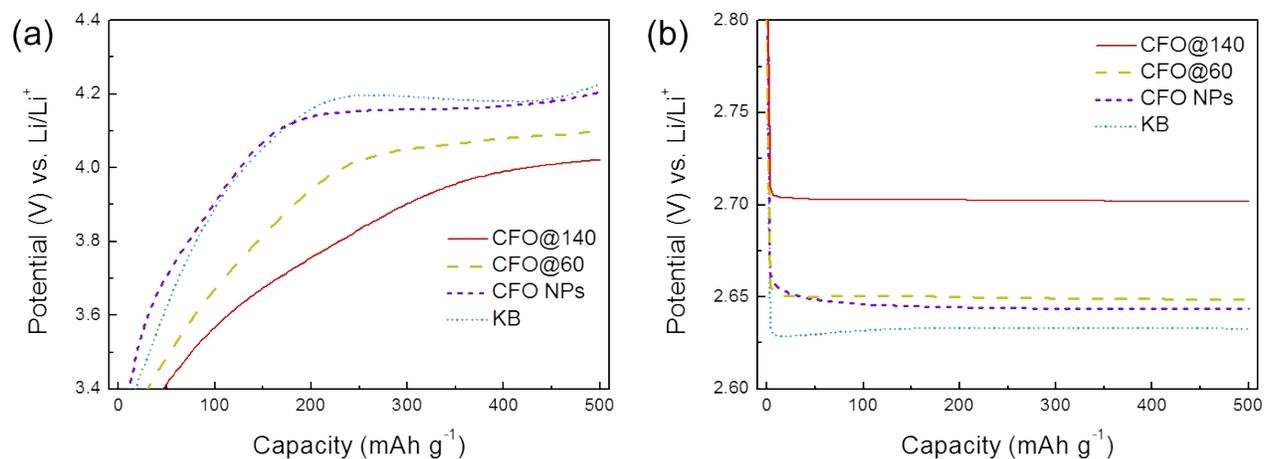
**Fig. S7** Magnified potential-capacity curves for (a) initial charging and (b) initial discharging of the Li-O<sub>2</sub> cells with KB, CFO NPs, CFO@60, and CFO@140 at a current density of 200 mA g<sup>-1</sup> with the limited capacity depth of 500 mAh g<sup>-1</sup>.
