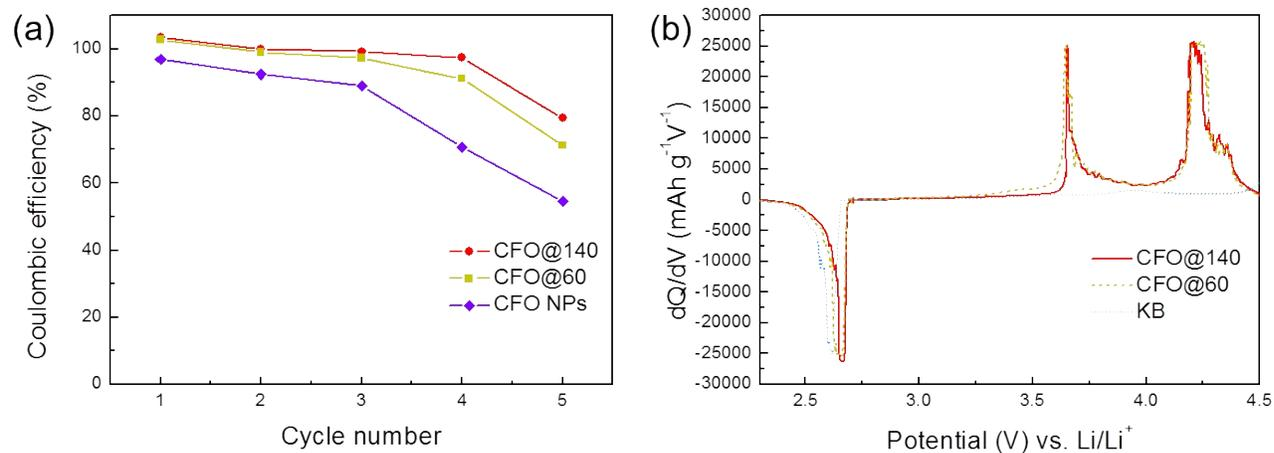
**Fig. S4** (a) Coulombic efficiency-cycle number curves for Li-O<sub>2</sub> cells with CFO NPs, 3DOM CFO@60, and CFO@140 catalysts for five cycles. (b) Plots of the differential capacity *versus* the voltage at a current density of 200 mA g<sup>-1</sup>.
