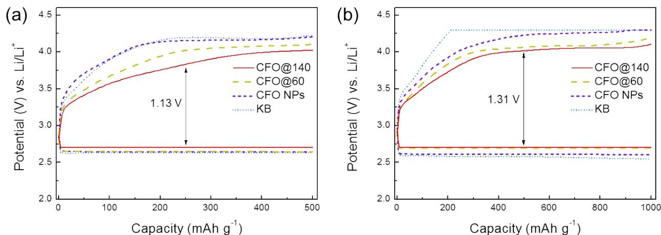
**Fig. S6** Discharge-charge curves of Li-O<sub>2</sub> cells with KB, CFO NPs, 3DOM CFO@60, and CFO@140 catalysts at a current rate of 200 mA g<sup>-1</sup> with the limited capacity depth of (a) 500 and (b) 1000 mAh g<sup>-1</sup>. KB in Fig. S6b was studied in our previous work [5].
