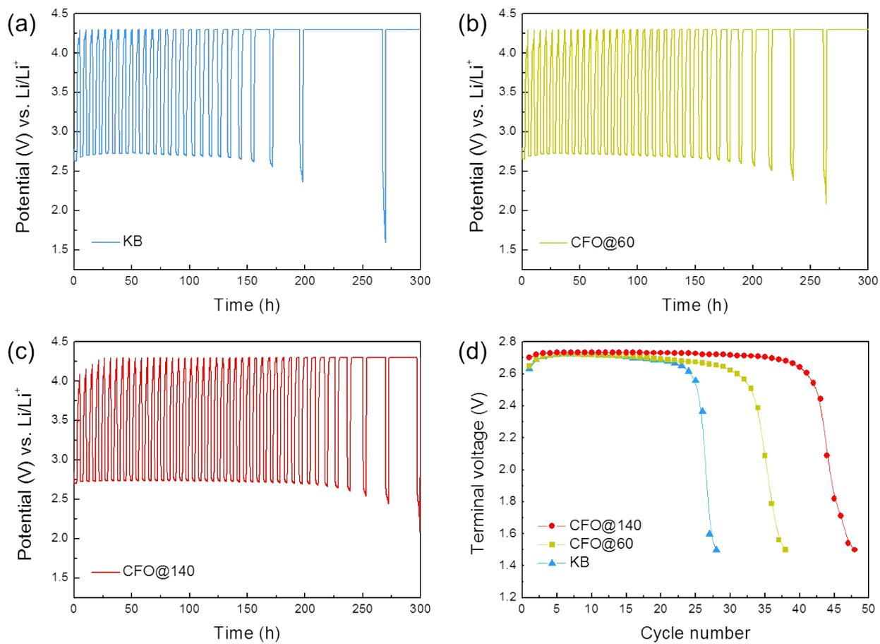
**Fig. S8** Potential-time curves of Li-O<sub>2</sub> cells with (a) KB, (b) CFO@60, and (c) CFO@140 catalysts. (d) Terminal voltage-cycle number curves with KB, CFO@60, and CFO@140.
