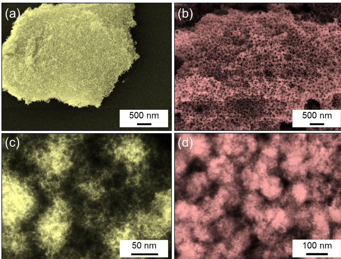
**Fig. S2** SEM images (a and b) of CFO@60 and CFO@140. TEM images (c and d) of CFO@60 and CFO@140.
