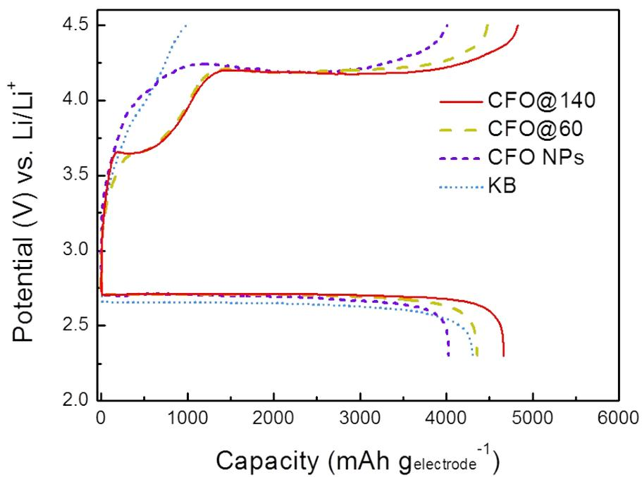
**Fig. S5** The discharge-charge profiles of Li-O<sub>2</sub> cells with KB, CFO NPs, 3DOM CFO@60, and CFO@140 at the first cycle. The capacities are normalized by the total mass of electrode (catalyst, carbon, and binder).
