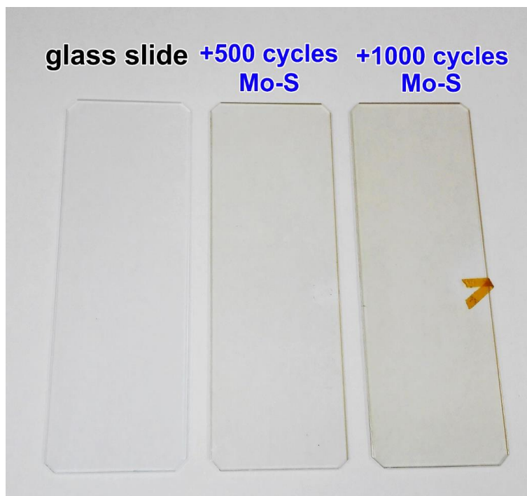
Fig. S5 Digital photograph showing the appearance of glass slides before and after ALD of MoS 2 .
