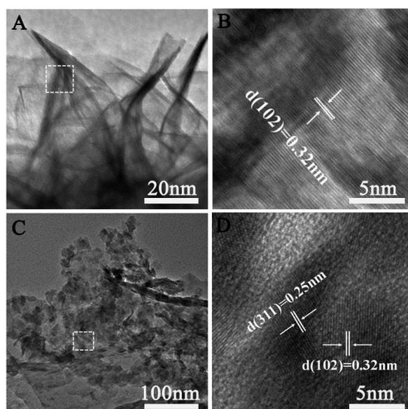
**Fig. S1.** (A) and (B) are the TEM and HRTEM images of ZnIn<sub>2</sub>S<sub>4</sub>, respectively; (C) and (D) are the TEM and HRTEM images of the ZnFe<sub>2</sub>O<sub>4</sub>/ZnIn<sub>2</sub>S<sub>4</sub> composite, respectively.
