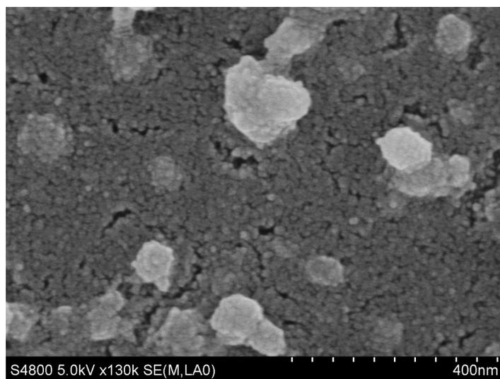
**Fig. S2.** SEM image of the ZnFe<sub>2</sub>O<sub>4</sub> film.
