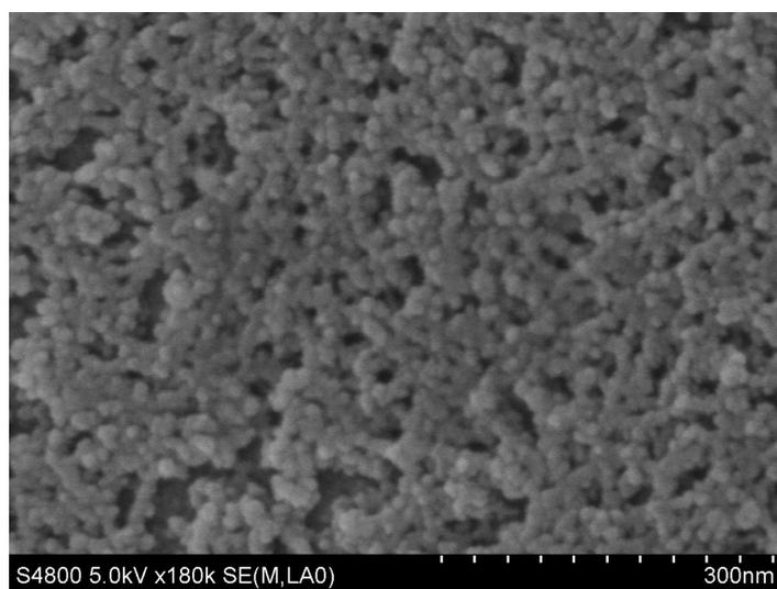
**Fig. S3.** SEM image of the CdS film.
