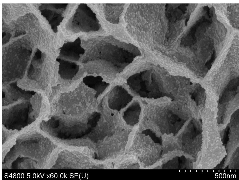
**Fig. S7.** SEM image of the 1-CdS/ZnFe<sub>2</sub>O<sub>4</sub>/ZnIn<sub>2</sub>S<sub>4</sub> film after five times consecutive recycling of photoreaction.
