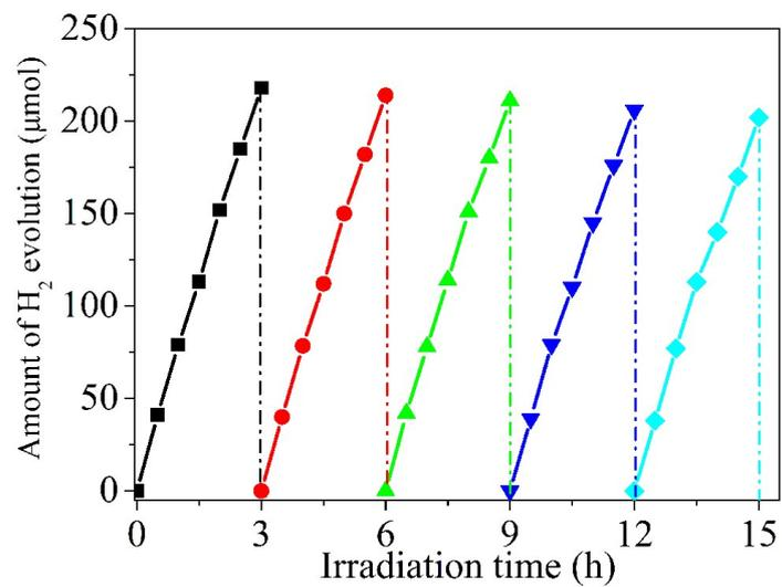
**Fig. S6.** Recycling test of the 1-CdS/ZnFe<sub>2</sub>O<sub>4</sub>/ZnIn<sub>2</sub>S<sub>4</sub> film for the visible light ( $\lambda \geq 420$  nm) H<sub>2</sub> evolution in aqueous solution.
