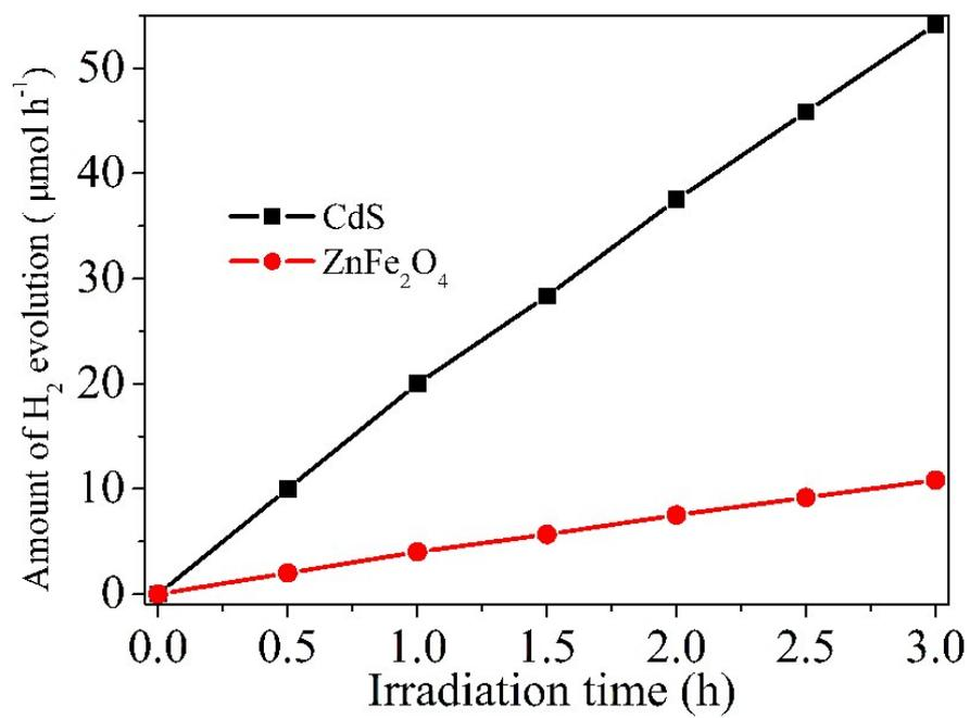
**Fig. S4.** Time-dependent photocatalytic H<sub>2</sub> evolution for the CdS and ZnFe<sub>2</sub>O<sub>4</sub> film catalysts.
