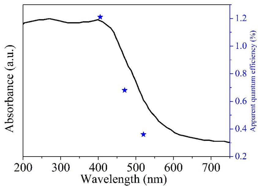
**Fig. S5** The apparent quantum efficiencies of the 1-CdS/ZnFe<sub>2</sub>O<sub>4</sub>/ZnIn<sub>2</sub>S<sub>4</sub> film against wavelength of monochromatic light.
