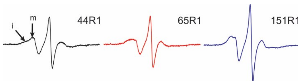
Figure S1. The CW-EPR spectra of three representative spin-labeled protein in buffer with 30% sucrose. These data are consistent with the literature. 2,5,6 The arrows labeled with “i” and “m” indicate the spectrum of 44R1 contains an immobile and a mobile component, respectively, also consistent with the literature. 5 The scan range is 100 G for each spectrum.
