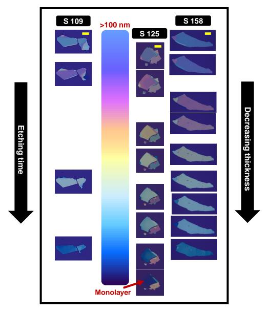
S1: Thickness dependent color profile of MoS<sub>2</sub> flakes
