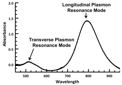
**Fig. S2** –Extinction spectrum of GNRs where absorbance= $-\ln(T)$ , with *T*=transmittance (density is  $\sim 1 \times 10^7$  GNRs/µL in a 1 cm thick sample).
