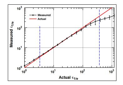
Fig. S5. Results of Monte Carlo Simulations of DS-OCT measurements showing how the measured decay constant ( $\tau_{1/e}$ ) varies with the true decay constant. All times are reported relative to the sampling time ( $\Delta t$ =1). Blue dashed lines indicate the minimum and maximum  $\tau_{1/e}$  accepted by the test in Eq. (8). (Mean ± standard deviation over 10 simulated measurements).
