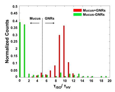
**Fig. S3** – Normalized histogram of the ratio of the isotropic and cross-polarized decorrelation times, showing that the ratio is around 1 (with 0 indicating no real decay constant) for only mucus and centering around 9-10 for mucus with GNRs. We therefore chose to use 5 as the cut-off point for the DS-OCT signal test.
