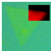
Fig. S3 Raman mapping image of the WSe 2 nanosheet at the peak of 250 cm -1 (corresponding to the A 1g and E 2g 1 )
