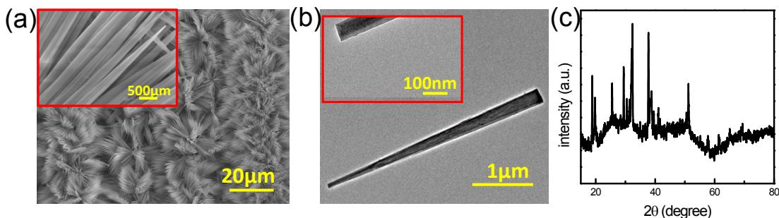
**Fig. S1.** SEM (a) and TEM (b) images of  $\text{Co}(\text{OH})_2$ , XRD pattern of  $\text{Co}(\text{OH})_2$  (c).
