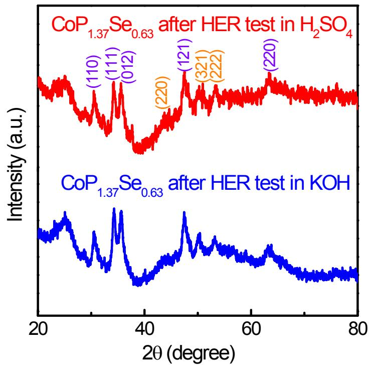
**Fig. S7.** XRD patterns of  $\text{CoP}_{1.37}\text{Se}_{0.63}$  NWs after HER test in both 0.5 M  $\text{H}_2\text{SO}_4$  and 1.0 M KOH solution.
