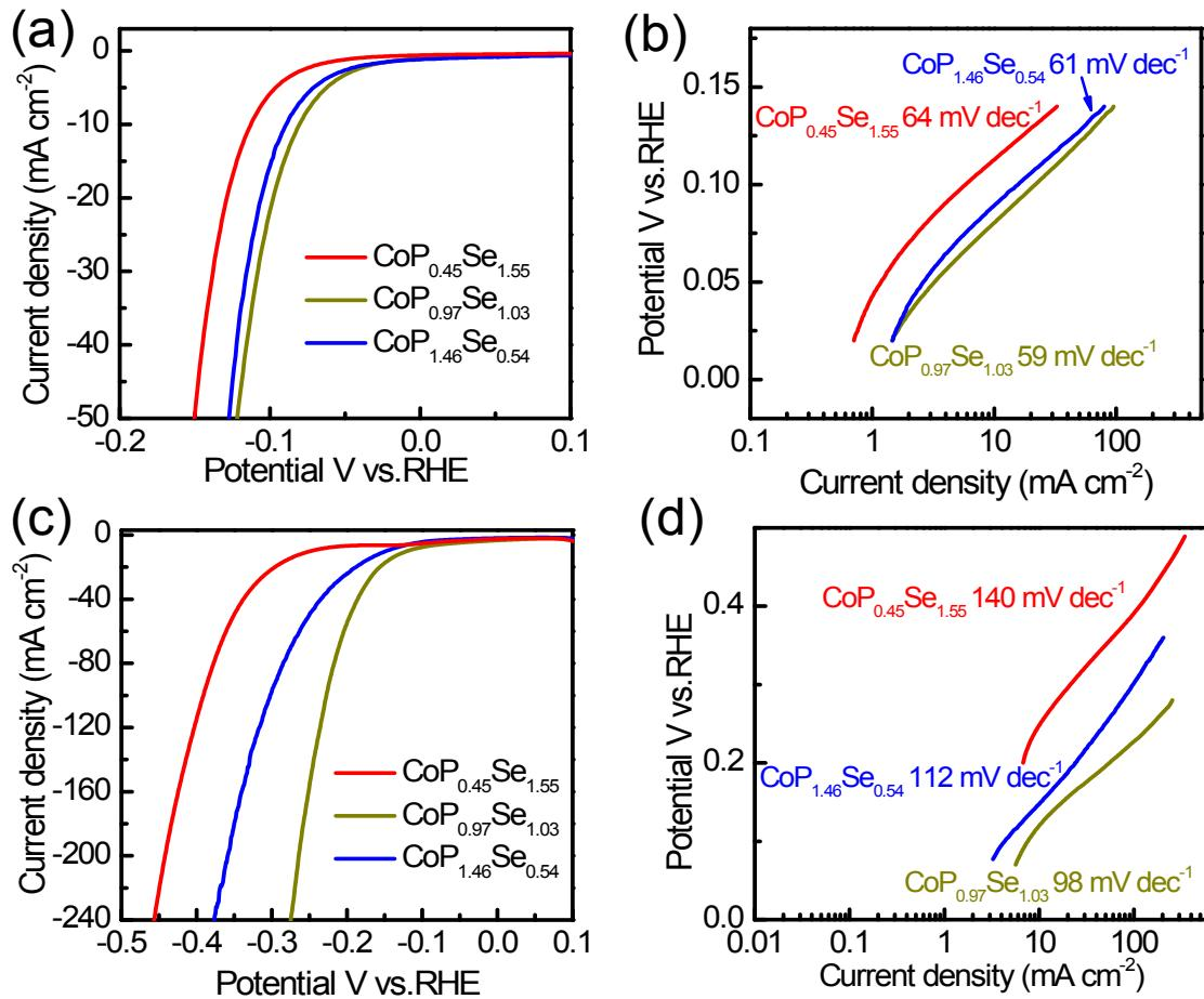
**Fig. S4.** Polarization curves of  $\text{CoP}_{0.45}\text{Se}_{1.55}$ ,  $\text{CoP}_{0.97}\text{Se}_{1.03}$  and  $\text{CoP}_{1.46}\text{Se}_{0.54}$  NWs for HER in both 0.5 M  $\text{H}_2\text{SO}_4$  and 1.0 M KOH solution (a and c). The corresponding Tafel plots for these ternary samples (b and d).
