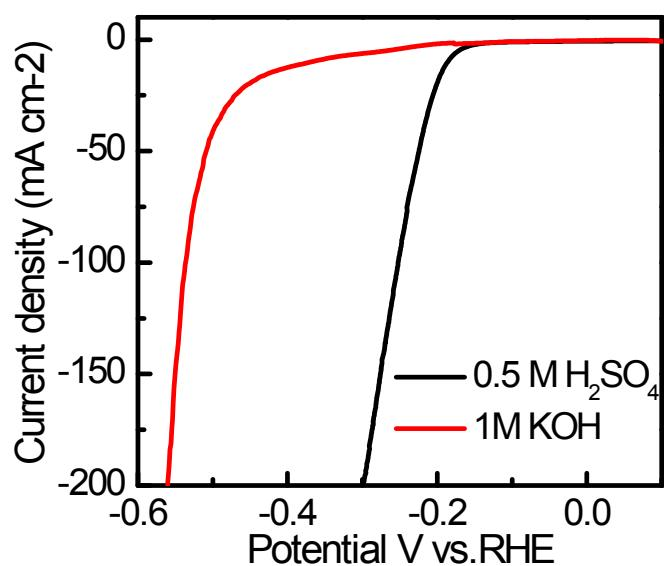
**Fig. S3** Polarization curves of  $\text{CoSe}_2$ NWs for HER in both 0.5 M  $\text{H}_2\text{SO}_4$  and 1.0 M KOH solution.
