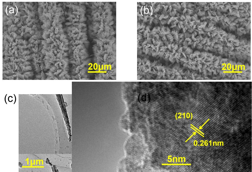
**Fig. S6.** SEM image of  $\text{CoP}_{1.37}\text{Se}_{0.63}$  NWs after HER test in 0.5 M  $\text{H}_2\text{SO}_4$ . SEM (b), TEM (c) and HRTEM (d) of  $\text{CoP}_{1.37}\text{Se}_{0.63}$  NWs after HER test in 1.0 M KOH.
