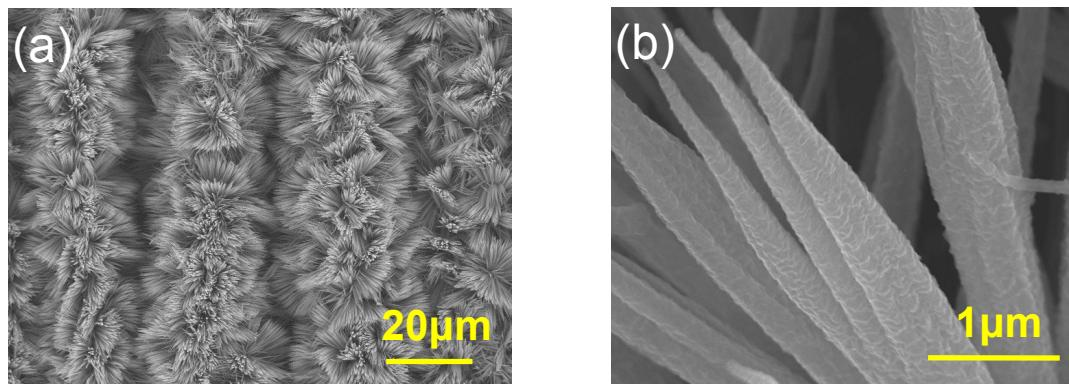
**Fig. S2.** Low-magnification SEM (a) and high-magnification SEM (b) of  $\text{CoP}_{2x}\text{Se}_{2(1-x)}$  NWs.
