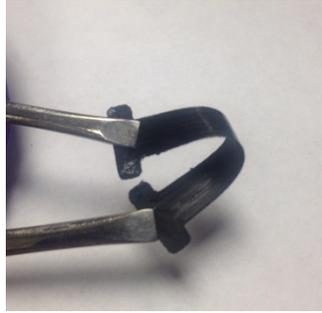
**Figure S2:** A two-layer (10:90)-MWCNT/PVDF dogbone sensor held between two sets of tweezers demonstrating the high flexibility of the printed composite materials.
