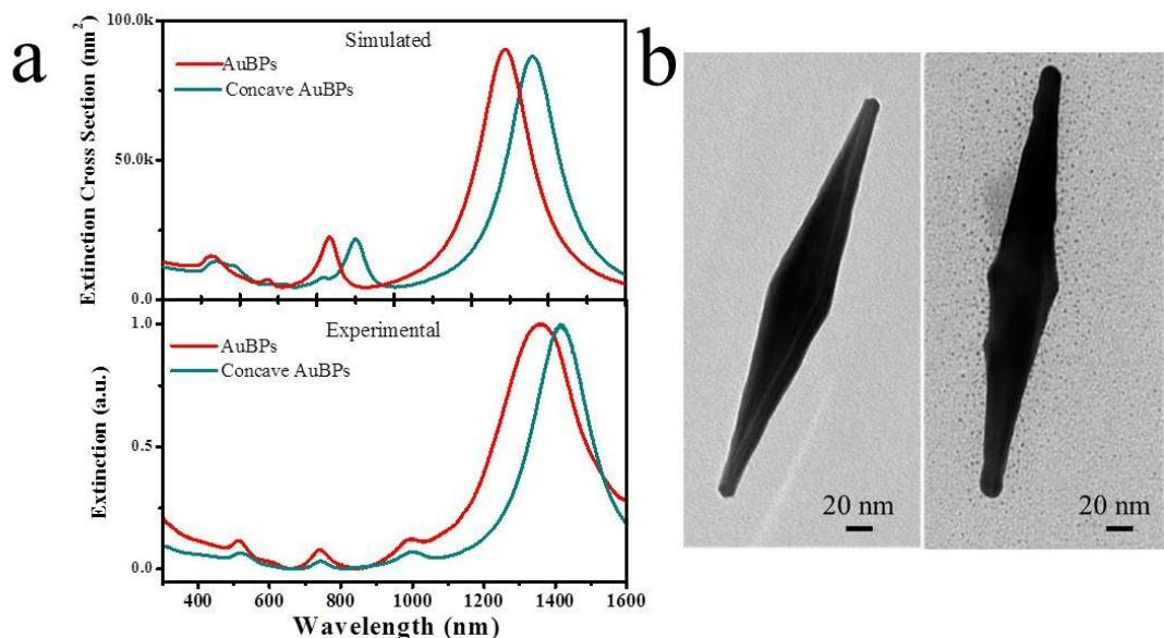
Fig. S10 a)The simulated and experimental extinction spectra of AuBPs and Concave AuBPs with similar sizes. b) TEM images of AuBPs (left, length =  $282 \pm 5$  nm, width =  $52 \pm 2$ ) and Concave AuBPs (right, length =  $281 \pm 6$  nm, width =  $51 \pm 3$ ) for experimental extinction spectra.
