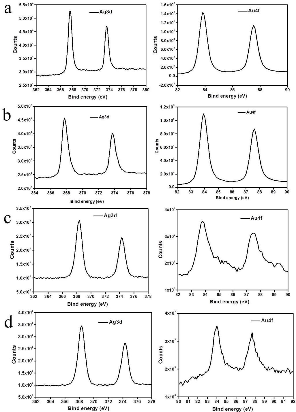
Fig. S8 XPS spectra of the samples overgrowth with different  $\text{Ag}^+$  concentration.a) AuBPs as seeds. b) overgrowth with 10  $\mu\text{l}$   $\text{AgNO}_3$ . c) overgrowth with 20  $\mu\text{l}$   $\text{AgNO}_3$ . d) overgrowth with 40  $\mu\text{l}$   $\text{AgNO}_3$ .
