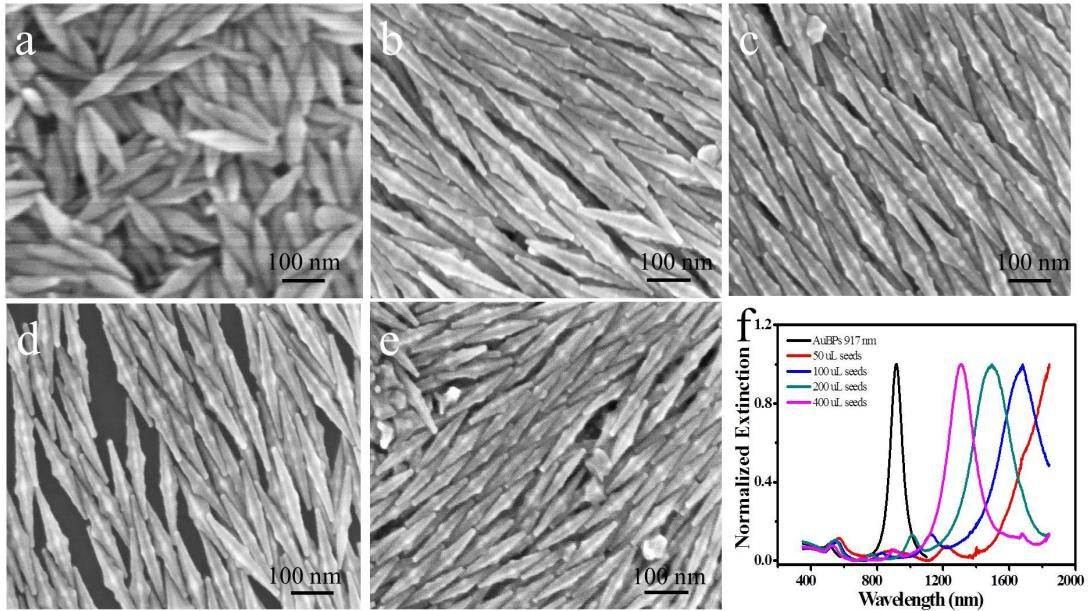
Fig. S3 SEM images of AuBPs with a LPW of 917 nm (a) and corresponding CAuBPs regrown from different amount of AuBPs as seeds (b-e): (b) 50  $\mu\text{L}$ . (c) 100  $\mu\text{L}$ . (d) 200  $\mu\text{L}$ . (e) 400  $\mu\text{L}$ . (f) The corresponding extinction spectra of the AuBPs and CAuBPs.
