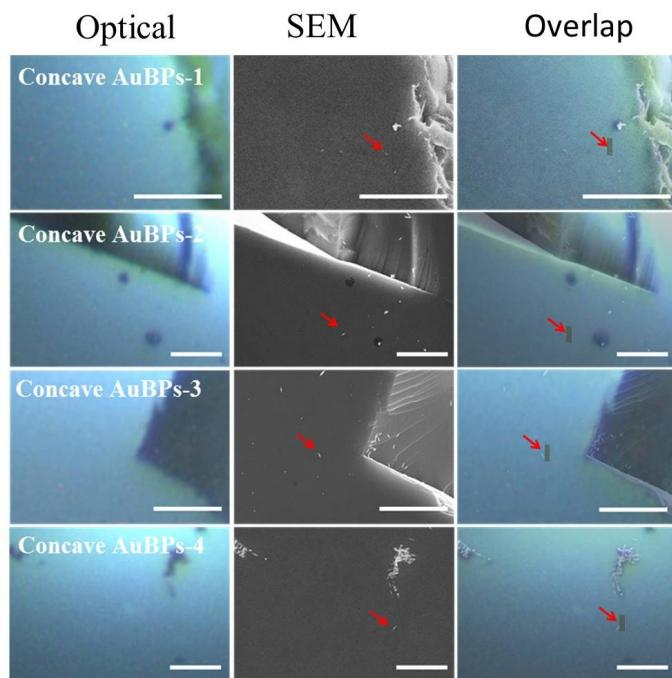
Fig. S12 Optical, SEM and corresponding overlap images of different concave AuBPs at the length of  $285 \pm 13$  nm,  $410 \pm 10$  nm,  $577 \pm 13$  nm and  $748 \pm 14$  nm, respectively. Scale bar = 500 nm.
