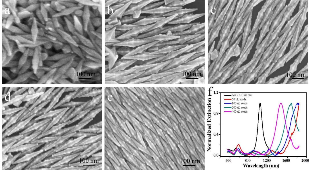
Fig. S4 SEM images of AuBPs with a LPW of 1045 nm (a) and corresponding CAuBPs regrown from different amount of AuBPs as seeds (b-e): (b) 50  $\mu\text{L}$ . (c) 100  $\mu\text{L}$ . (d) 200  $\mu\text{L}$ . (e) 400  $\mu\text{L}$ . (f) The corresponding extinction spectra of the AuBPs and CAuBPs.
