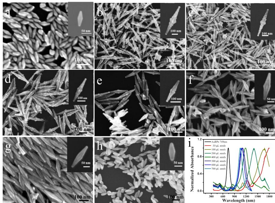
Fig. S2 SEM images of AuBPs with a LPW of 749 nm (a) and corresponding CAuBPs regrown from different amount of AuBPs as seeds (b-h): (b) 50  $\mu$ L. (c) 100  $\mu$ L. (d) 200  $\mu$ L. (e) 400  $\mu$ L. (f) 500  $\mu$ L. (g) 600  $\mu$ L. (h) 700  $\mu$ L. (i)The corresponding extinction spectra of the AuBPs and CAuBPs.
