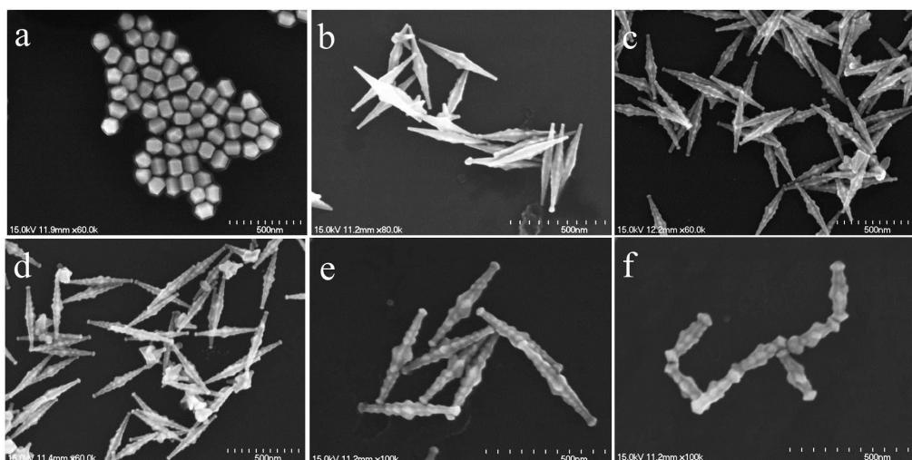
Fig. S7 SEM images of as-synthesized nanoparticles with different amount of  $\text{AgNO}_3$ .
