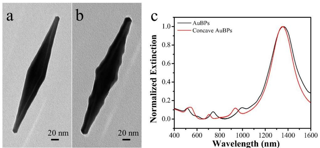
Fig. S11 (a) TEM images of AuBPs (length =  $282 \pm 5$  nm, width =  $52 \pm 2$  nm) and CAuBPs (length =  $285 \pm 13$  nm, width =  $59 \pm 3$ ). (b) The corresponding extinction spectra.
