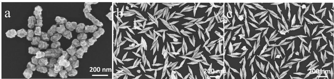
Fig. S9 SEM images of as-synthesized nanoparticles with different surfactants. (a) CTAC. (b) CTAB+CTBAB. (c) CTAC+CTBAB.
