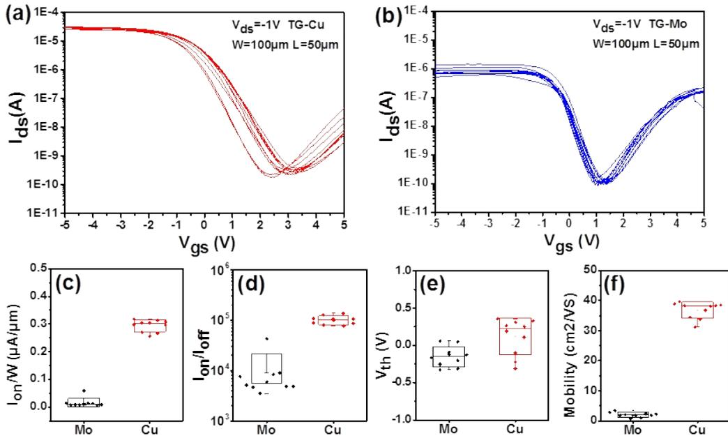
Ten devices were measured for both Cu- and Mo-contacted devices with the same designed geometry ( $W = 100 \mu m$ ,  $L = 50 \mu m$ ). The Cu contacted devices show higher performances obviously.
