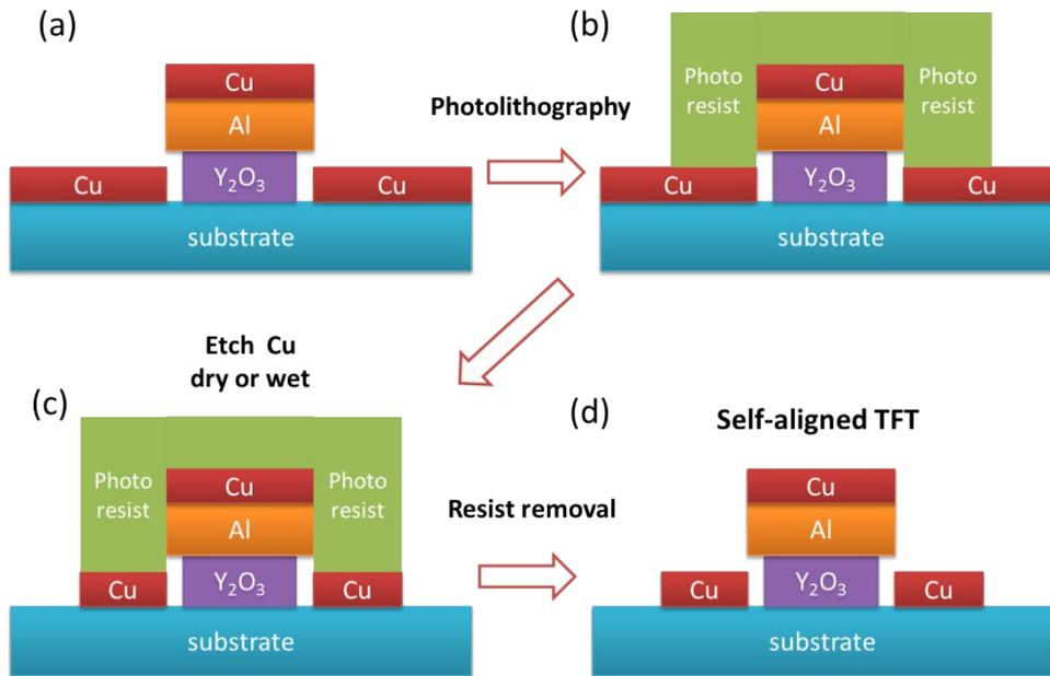
The suggested fabrication process for small channel length device is similar to the TG device fabrication in Fig. 1a of the main text. After the Al/ $Y_2O_3$  gate stack etching, Cu was deposited to the substrate entirely as shown in Fig. S10(a). Then S/D were patterned as shown in (b)-(d). The gap between the gate and S/D electrode (as shown in Fig. 7a of the main text) was minimized by a self-align deposition due to the undercut profile of the gate stack.
