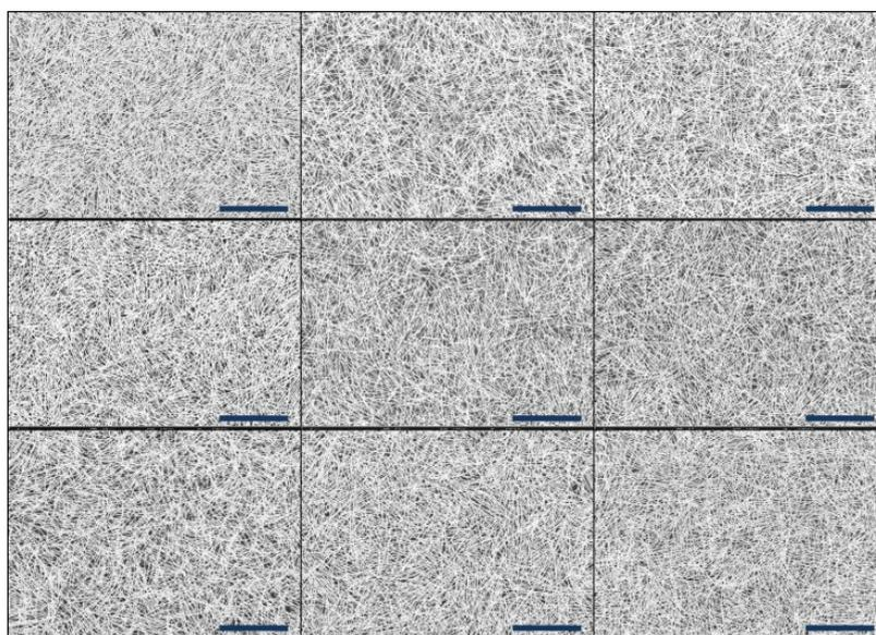
The SEM image below shows the density of CNT deposited in the TG and BG devices are similar. Scale bar: 2  $\mu\text{m}$ .
