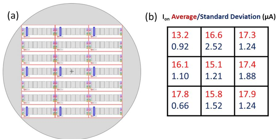
There are 21 dies, 7 rows by 3 columns, in the wafer. Each die includes four groups of devices. Each group has 100 units, 10 columns  $\times$  10 rows, and 3 devices in each unit. The devices have the same geometry, channel length ( $L$ ), and width ( $W$ ), in the same column, but different geometries for different columns. There are 10 designed
