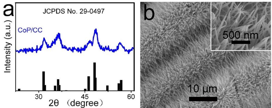
**Fig. S5.** (a) XRD pattern for CoP scratched down from CC. (b) SEM images for CoP/CC.
