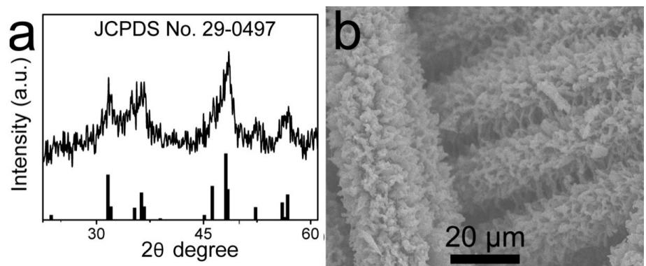
**Fig. S8.** (a) XRD pattern for Al-CoP and (b) SEM image for Al-CoP/CC after HER hydrolysis.
