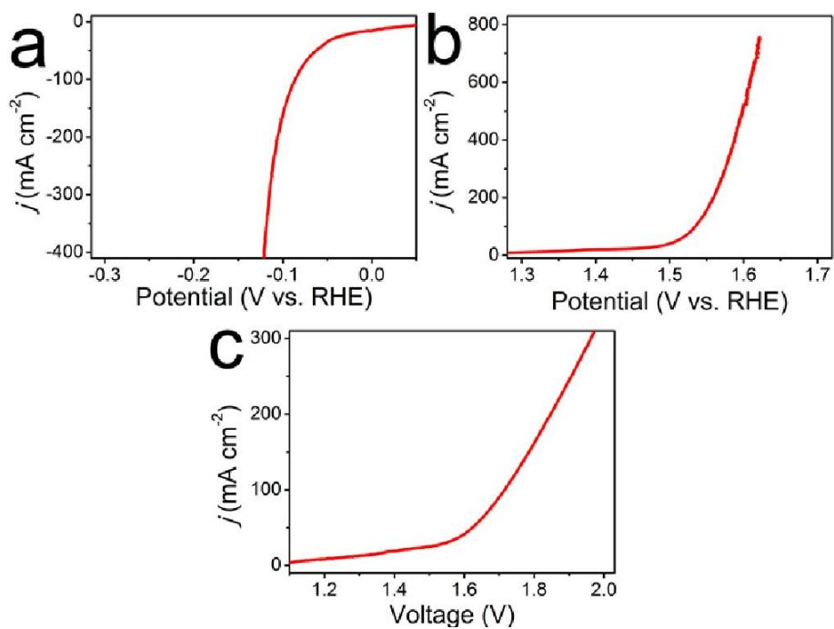
**Fig. S16.** Polarization curves for (a) HER and (b) OER with a scan rate of  $5 \text{ mV s}^{-1}$ . (c) Polarization curve of Al-CoP/NF||Al-CoP/NF in a two-electrode setup for full water splitting with a scan rate of  $5 \text{ mV s}^{-1}$ . All experiments were performed in  $1.0 \text{ M KOH}$ .
