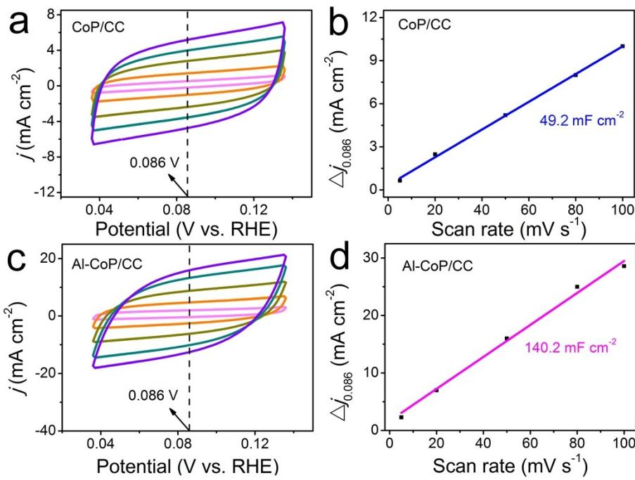
**Fig. S10.** CVs of (a) CoP/CC and (c) Al-CoP/CC after electrolysis with various scan rates ( $5\text{--}100\text{ mV s}^{-1}$ ) in the region of 0.036 to 0.136 V. The capacitive current densities at 0.086 V as a function of scan rate for (b) CoP/CC and (d) Al-CoP/CC. All experiments were performed in 0.5 M  $\text{H}_2\text{SO}_4$ .
