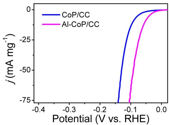
**Fig. S6.** Mass-normalized polarization curves for Al-CoP/CC and CoP/CC in 0.5 M  $\text{H}_2\text{SO}_4$ .
