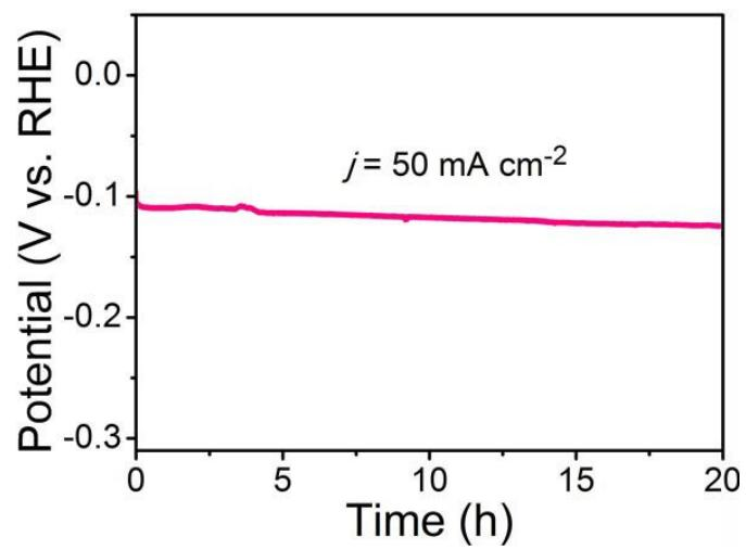
**Fig. S13.** Chronopotentiometric curve of Al-CoP/CC with constant current density of  $50 \text{ mA cm}^{-2}$  for HER in 1.0 M KOH (without iR correction).
