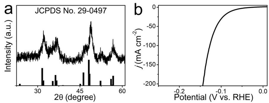
**Fig. S12.** (a) XRD pattern and (b) polarization curve for HER of Al-doped CoP nanoarray on CC with Al doping degree: 35%.
