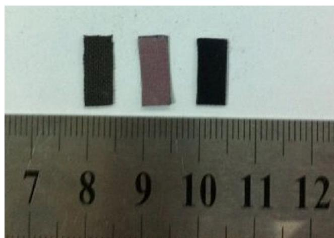
**Fig. S1.** Optical photograph for CC, CoAl-LDH/CC, and Al-CoP/CC (from left to right).
