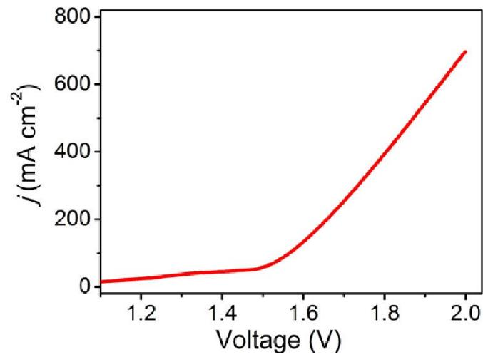
**Fig. S17.** (a) Polarization curve of Al-CoP/NF||Al-CoP/NF in a two-electrode setup for full water splitting with a scan rate of  $5 \text{ mV s}^{-1}$  in  $1.0 \text{ M KOH}$  at  $65^\circ\text{C}$ .
