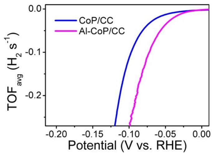
**Fig. S7.** TOF<sub>avg</sub> calculation of Al-CoP/CC and CoP/CC.
