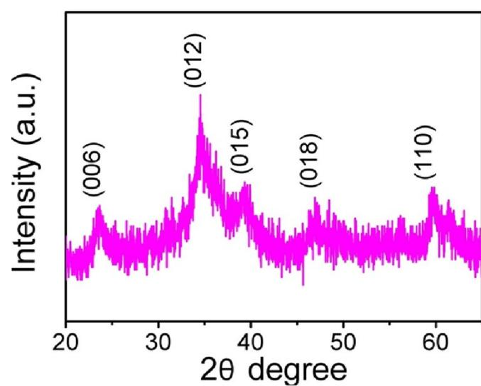
**Fig. S2.** XRD pattern of CoAl-LDH scratched down from CC.
