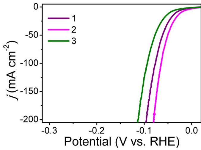
**Fig. S11.** Polarization curves for HER of Al-doped CoP nanoarray on CC with different Al doping degree: 4% (curve 1), 10 % (curve 2), and 16 % (curve 3). All experiments were performed in 0.5 M H<sub>2</sub>SO<sub>4</sub> with a scan rate of 5 mV s<sup>-1</sup>.
