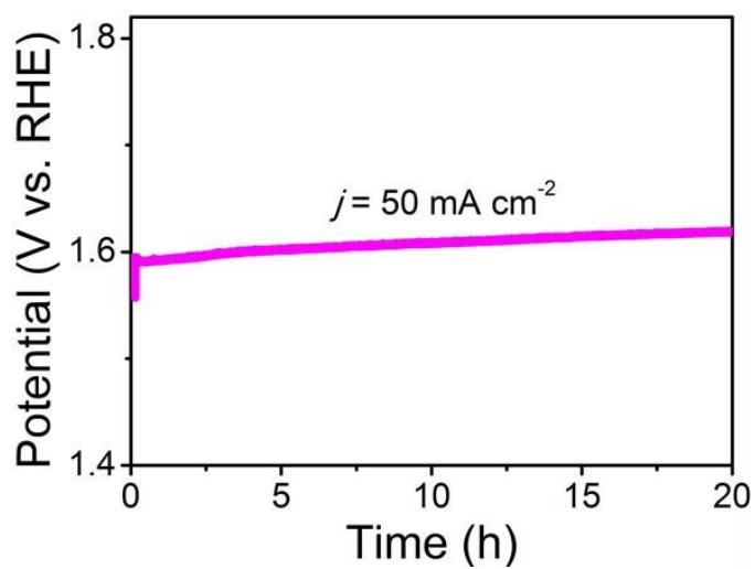
**Fig. S14.** Chronopotentiometric curve of Al-CoP/CC with constant current density of  $50 \text{ mA cm}^{-2}$  for OER in  $1.0 \text{ M KOH}$  (without iR correction).
