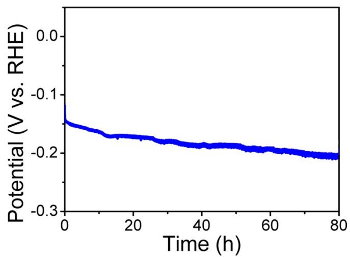
**Fig. S9.** Chronopotentiometric curve of CoP/CC with constant current density of  $50 \text{ mA cm}^{-2}$  for 80 h (without iR correction).
