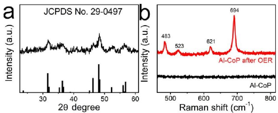
**Fig. S15.** (a)XRD pattern for Al-CoP after OER electrolysis and (b) Raman spectra for Al-CoP before and after OER electrolysis in 1.0 M KOH.
