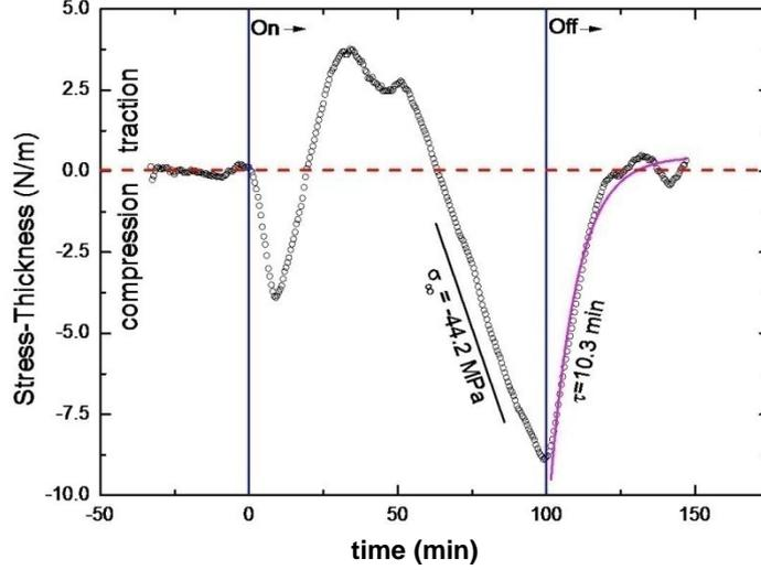
**Fig. 2s.** Stress-thickness evolution of an Au film deposited on (100)Si at a rate of  $F = 0.1$  nm/s. Vertical lines denotes the flux-on and flux-off transients. The solid curve corresponds to the fitting dependences (namely, stress-thickness  $\propto F\sigma_{\infty}t$  for a constant flux or  $\propto \exp(\pm t/\tau)$  for flux transients) together their parameters.
