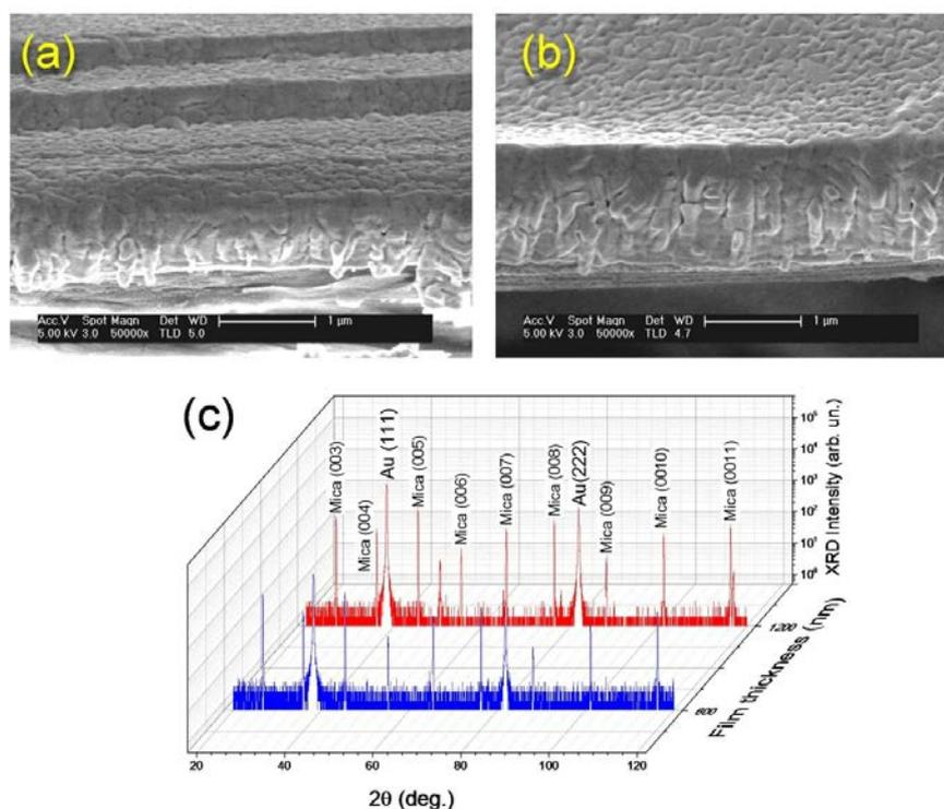
**Fig. 1s** Ex-situ sample characterization. (a, b) Cross-section SEM images of 600 nm and 1200 nm-thick Au films on mica substrates, respectively. (c)  $\theta$ -2 $\theta$  XRD scans of the same films.
