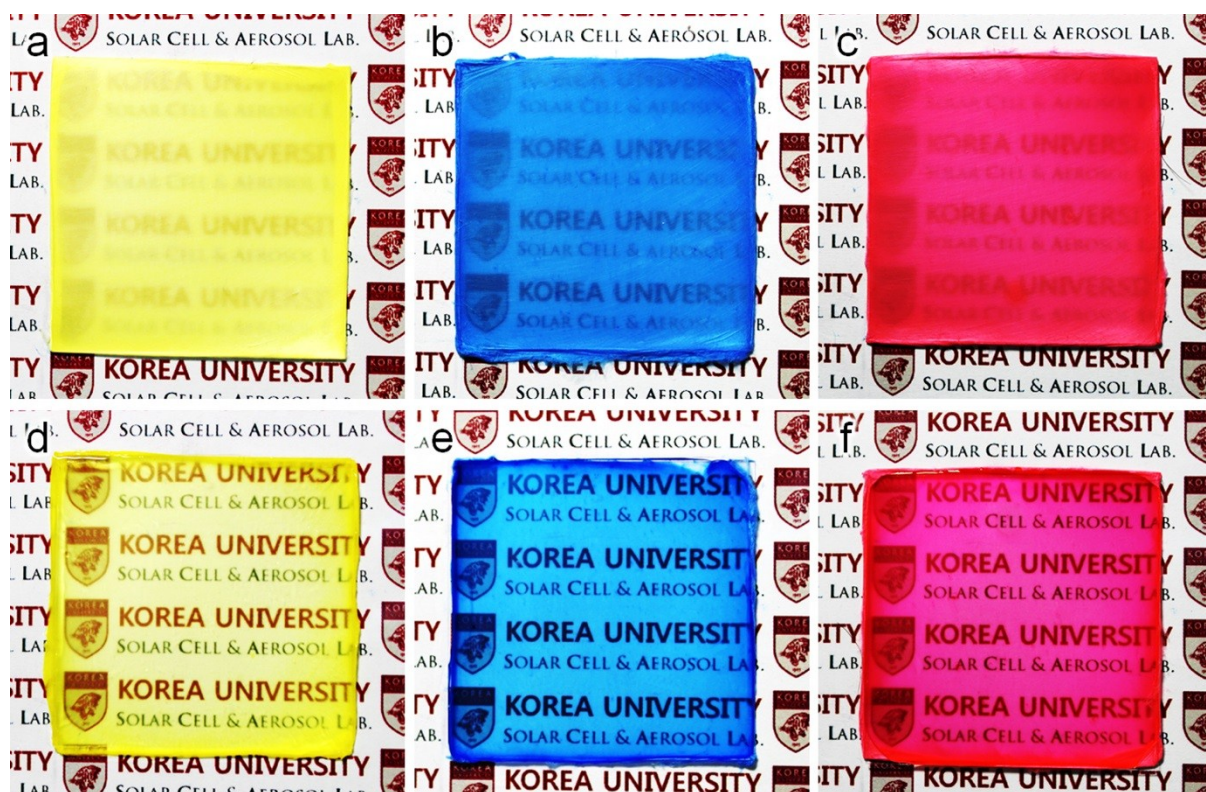
Fig. S7 Photographs of the (a and d) yellow-, (b and e) blue-, and (c and f) red-colored light-scattering layers on glass for t_1 = 120 min (a, b, and c) before applying PDMS, and (d, e, and f) after applying PDMS and the middle glass.
