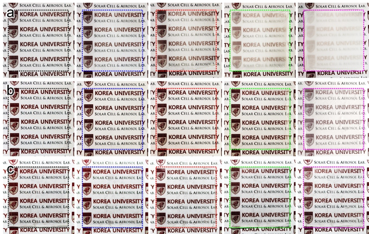
Fig. S2 Photographs of the fabricated films illustrating each step of the fabrication process: (a) light-scattering layers on glass before applying PDMS (cf. Fig. 2b ), (b) light-scattering layers (on glass) after applying PDMS and the middle glass (cf. Fig. 2d ), and (c) the hybrid films (where the defrosting layers and the top glasses were applied, cf. Fig. 2f ). The first electrospinning time t_1 was 5 min, 15 min, 30 min, 60 min, and 120 min from the left to the right columns.
