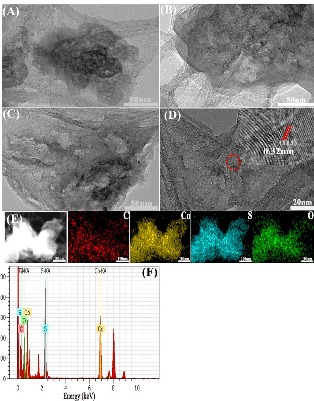
**Figure S2.** TEM images of (A-D) CNT-CoS<sub>2</sub>-60 and (E) STEM and corresponding element mapping. (F) EDS of CNT-CoS<sub>2</sub>-60.
