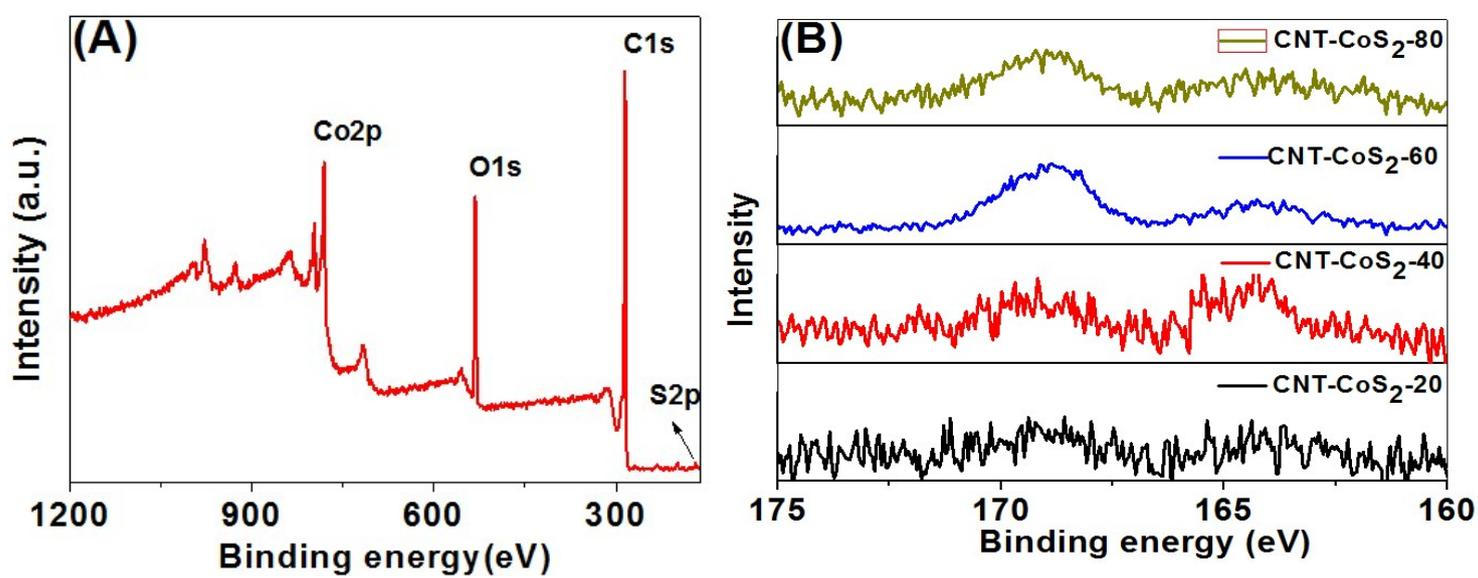
Figure S3. (A) XPS spectra survey of the CNT-CoS<sub>2</sub>-60; (B) S 2p region.
