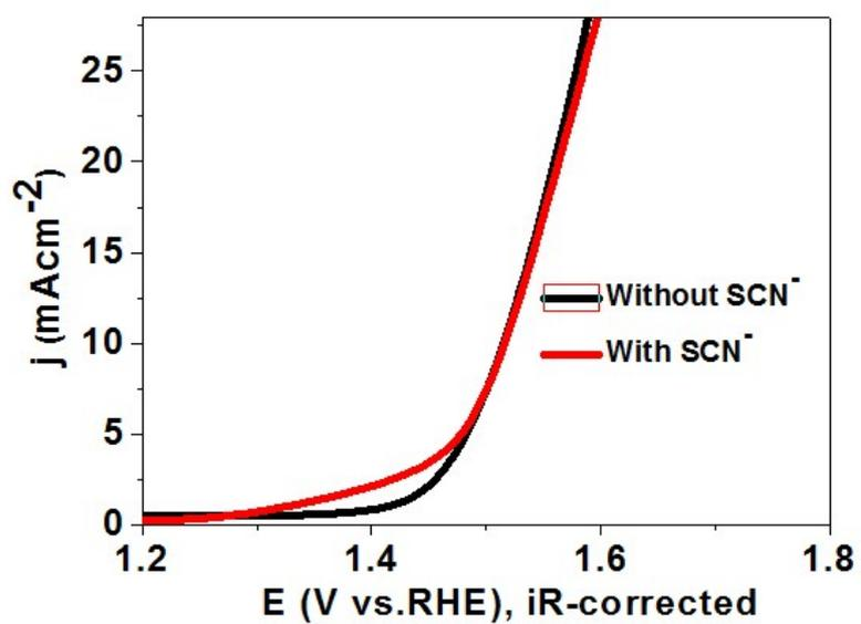
**Figure S11.** OER iR-corrected polarization plots of  $\text{IrO}_2$  in  $0.1\text{M KOH}$  with  $\text{KSCN}$ .
