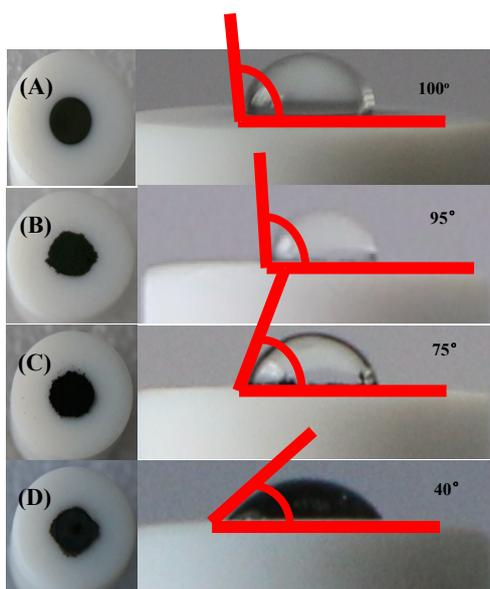
**Figure S6** Contact angle of different electrodes: (A) GCE; (B) Raw CNT; (C) CNT/CoS<sub>2</sub>; (D) CNT-CoS<sub>2</sub>-60.
