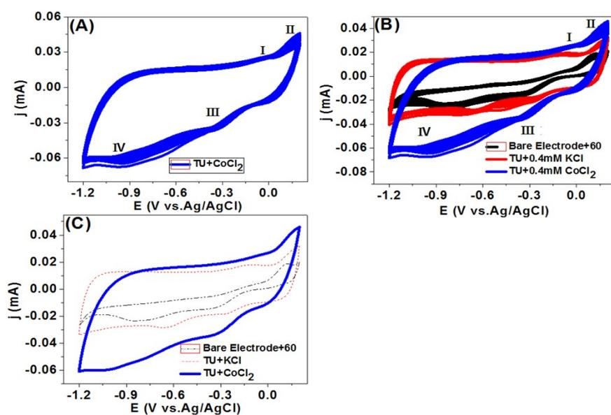
**Figure S1.** Electrodeposition cyclic voltammetry (CVs) of  $\text{CoS}_2$ . (A)  $0.4\text{mM CoCl}_2$  containing  $0.06\text{M}$  thiourea electrolyte on CNT; (B) Deposited on the various substrates: Bare Electrode (Bare glass carbon electrode, black), CNT (red: TU+KCl electrolyte, blue: TU+ $\text{CoCl}_2$  electrolyte). scan rate  $30\text{ mV s}^{-1}$ .
