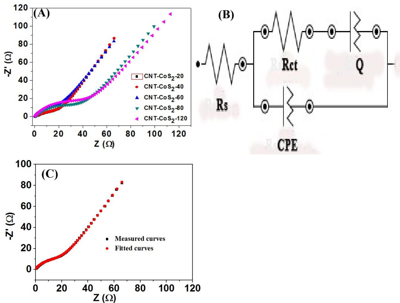
**Figure S8.** (A) Electrochemical impedance spectroscopy (EIS) of different cycles, condition: 0.01MKOH. (B) Equivalent circuit models OH-/O<sub>2</sub> of CNT-CoS<sub>2</sub>-60, (C) The measured and fitted curves of CNT-CoS<sub>2</sub>-60.
