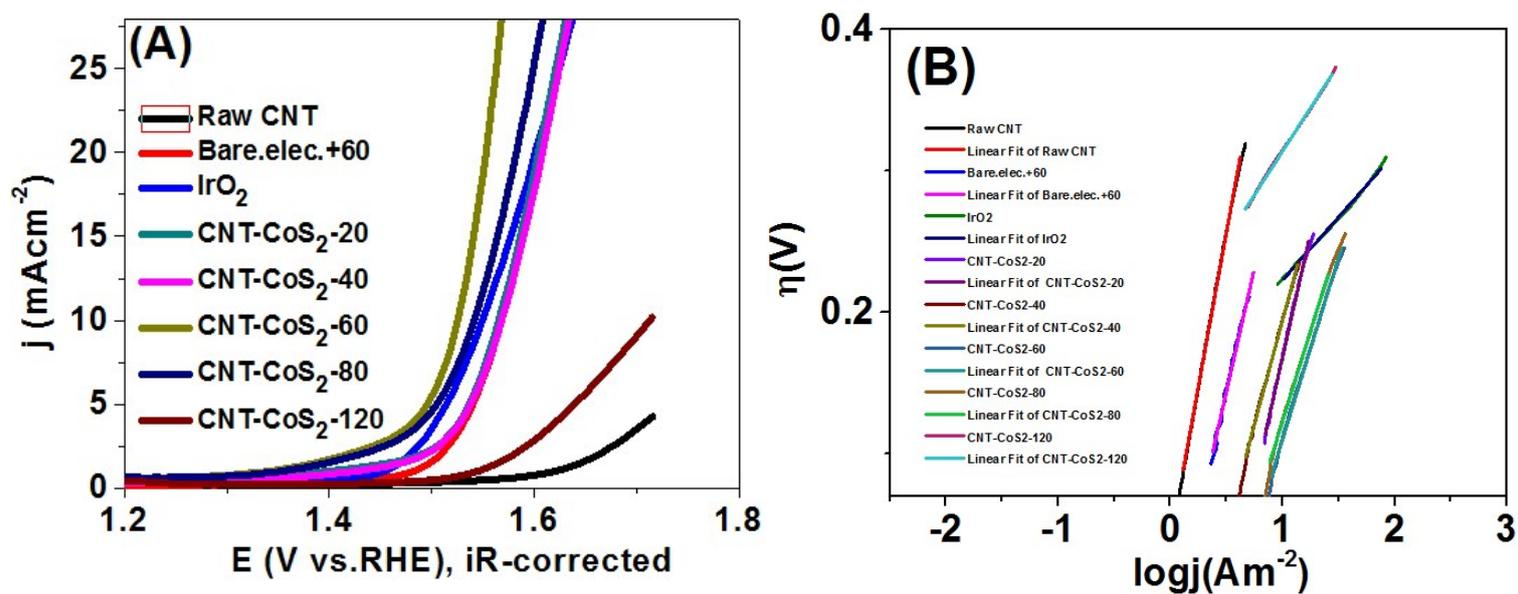
Figure S7. (A) iR-corrected Polarization curves for various CNT-CoS<sub>2</sub>. (B) iR-corrected Tafel Plot of (A).
