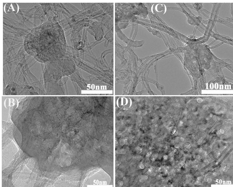
**Figure S10.** TEM images of different magnification: (A) CNT-CoS<sub>2</sub>-40; (B) CNT-CoS<sub>2</sub>-60; (C) CNT-CoS<sub>2</sub>-80; (D) CNT-CoS<sub>2</sub>-120.
