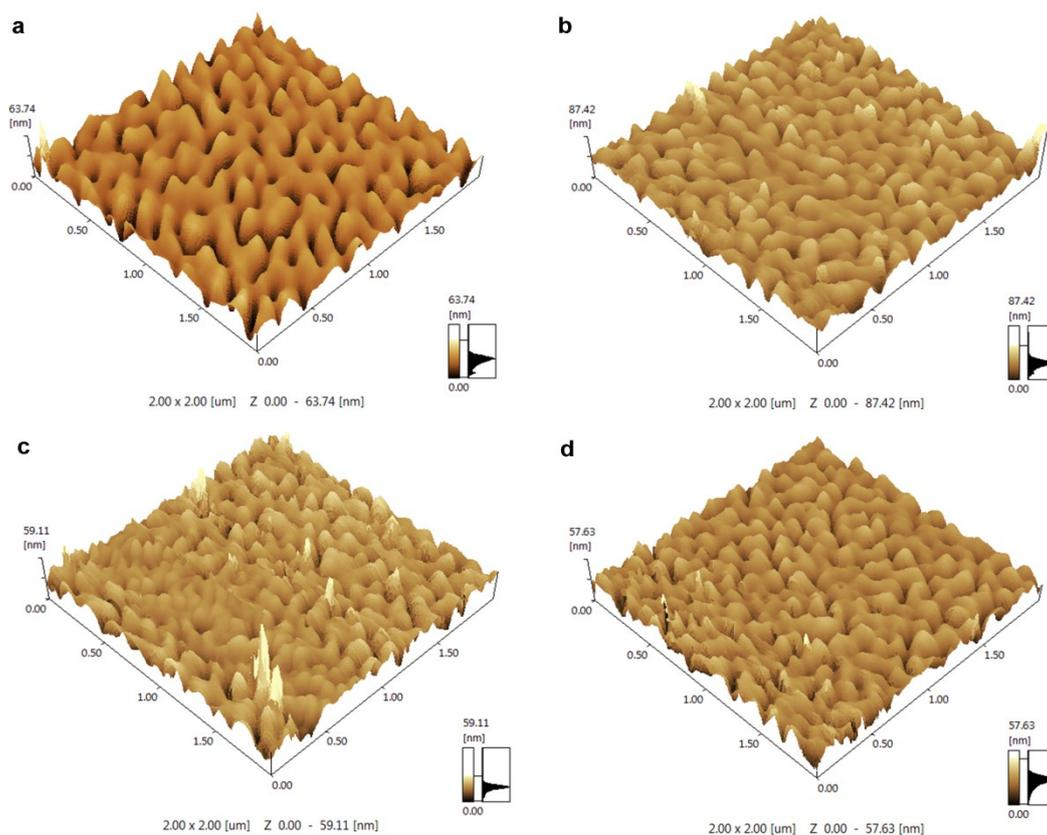
**Fig. S5** Surface morphologies of CBP layer as a function of MoO<sub>3</sub> overlayer thickness of 0–2.5 nm. (a) 0 nm. (b) 0.5 nm. (c) 1.5 nm. (d) 2.5 nm.
