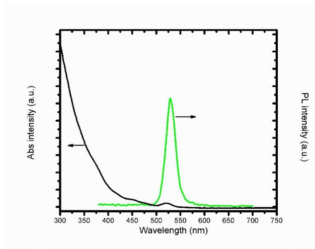
**Fig. S2** Ultraviolet-Visible absorption and PL emission spectra of green QD solution.
