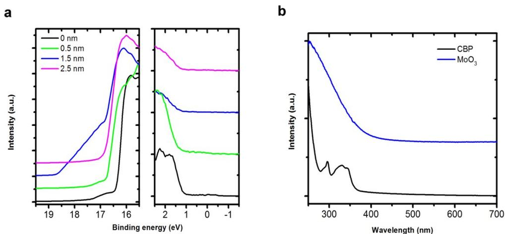
**Fig. S7** (a) UPS spectra of the CBP layer as a function of MoO<sub>3</sub> overlayer thickness of 0–2.5 nm. (b) Ultraviolet-Visible absorption spectra of CBP and MoO<sub>3</sub> layer.
