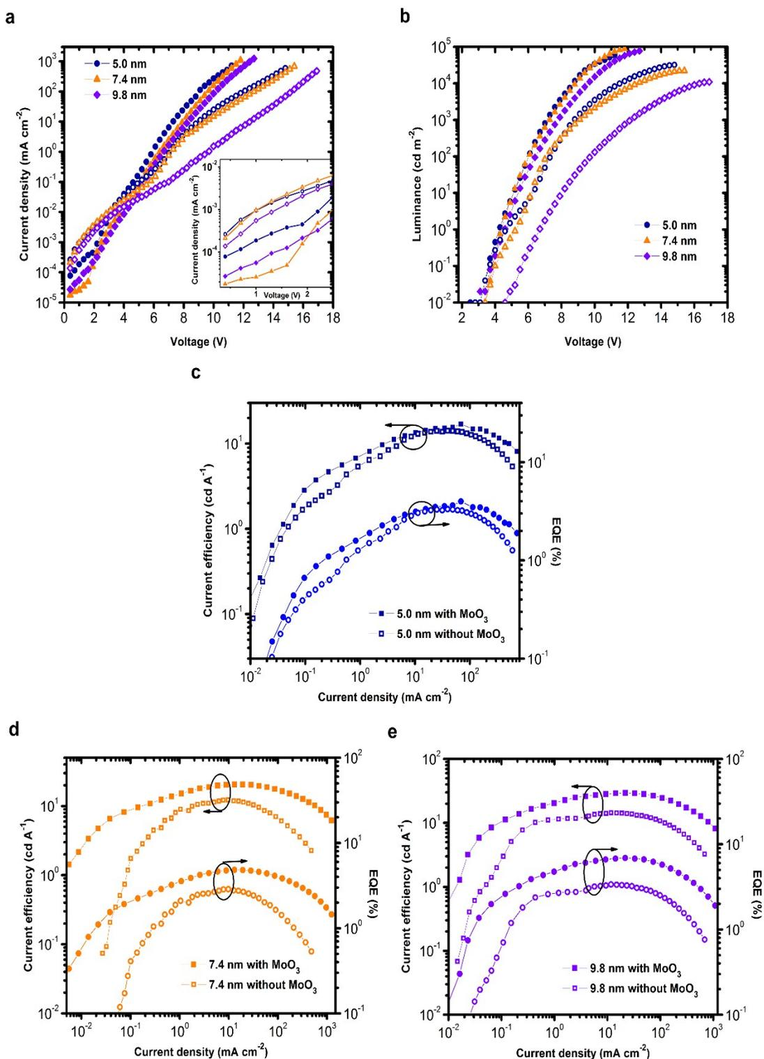
**Fig. 6** EL performance of QLEDs with different thickness HAT-CN layer. Devices that have 1.5 nm MoO<sub>3</sub> layer or not are represented by solid sign and hollow sign, respectively. (a) J-V characteristics. Inset: J-V curves at low bias voltage range. (b)
