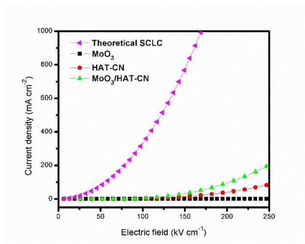
**Fig.S8** Current density-voltage (J-V) characteristics of hole-only device with different HIL.
