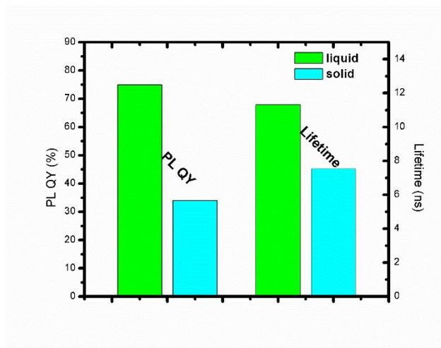
**Fig. S4** Comparison of PL QY and fluorescence lifetime of QDs in liquid and solid (film) states.
