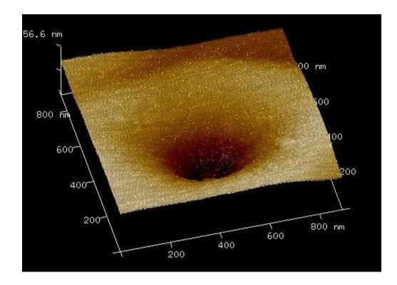
**Figure S2**. The AFM image of the femtosecond laser irradiated area of as-implanted fused silica. When the laser fluence is above  $0.5 \text{ J/cm}^2$ , there is a nanoscale crater in the irradiated area.
