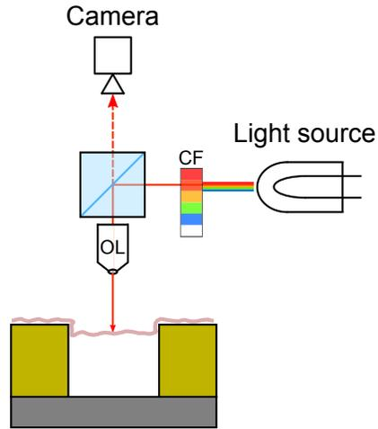
Figure S-1: Colorimetry setup: an optical microscope with Köhler illumination and a 20× objective lens (OL) is used for visualizing the suspended graphene drums. The white light illumination of a halogen lamp goes through a color filter (CF).
