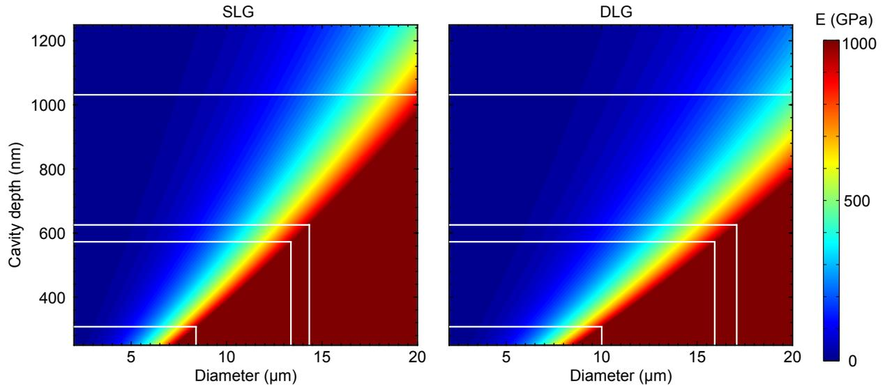
Figure S-5: Minimum Young's modulus of circular SLG (left) and DLG (right) membranes for different diameters and cavity depths for which a pressure difference of 1 bar would induce a deflection equal to the cavity depth.
