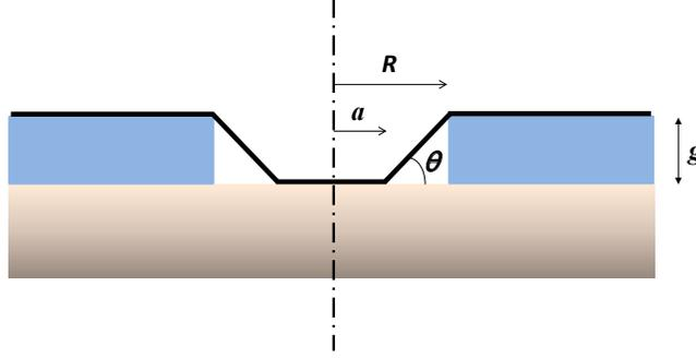
Figure S-3: Model of a stuck circular membrane of radius  $R$ , the stuck area is assumed to be circular with a radius  $a$ , and a cavity depth  $g$ . The tensed suspended part of the membrane forms an angle  $\theta$ .
