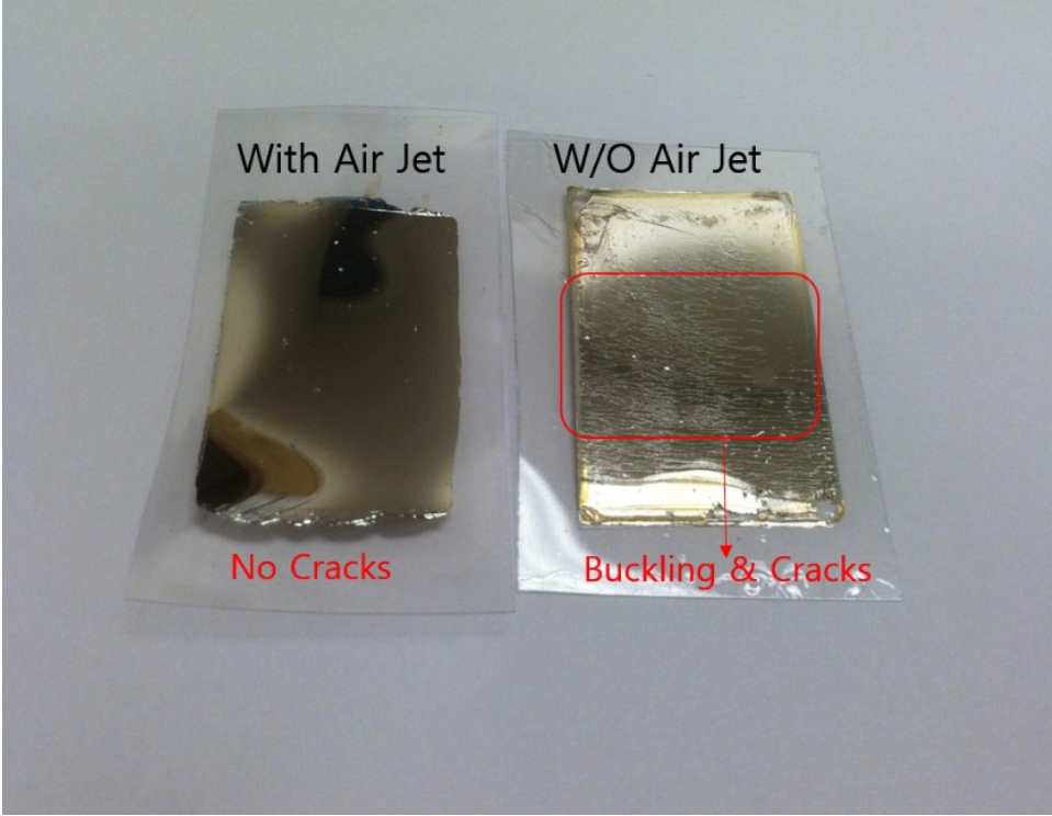
Figure. S2 Single Ag film delamination characteristics by using the air jetting system.
