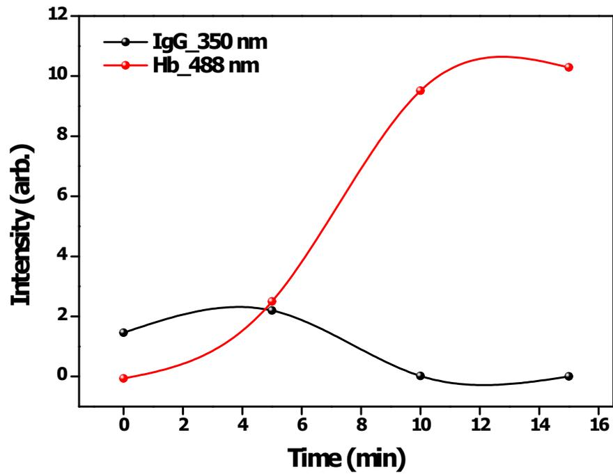
**Figure S4.** Fluorescence intensity as a function of penetration time using a mixture of Hb and IgG proteins in the nanosieve with SiN membrane. The signals were measured at a 50  $\mu\text{m}$ -away from the edge of the supporting membrane (200  $\mu\text{m}$  x 200  $\mu\text{m}$ ).
