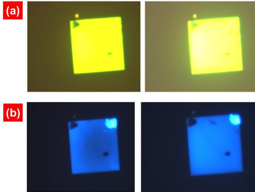
**Figure S3.** Fluorescence photographs showing selective penetration of mixture of Hemoglobin (Hb) (a) and Immunoglobulin G (IgG) (b) at separation-starting time and after 10 min in the nanosieve with SiN membrane, IgG is tagged with Alexa Fluor® 350 and Hb with Alexa Fluor® 488.
