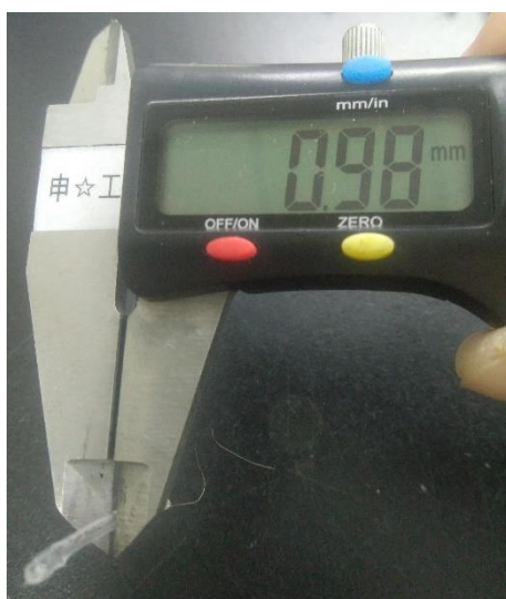
Figure S10. Optical photograph of the LIC's diameter measure with a vernier caliper.
