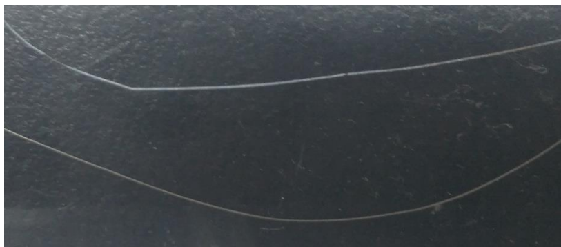
Figure S1. Optical photos of the pristine Ti (down) and LTO-NWA@Ti (up) wires.
