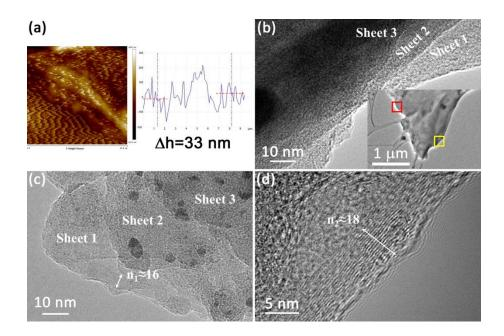
**Figure S3.** Thickness of the  $MoS_2$  nanosheet in Figure 3: (a) AFM image of the nanosheet, (b-d) TEM images of the nanosheet. The inset in (b) shows the low magnification TEM image of the nanosheet, (c) is the high magnification TEM image of the red region and (b,d) are the high magnification TEM images in the yellow region.
