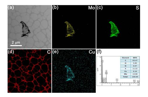
**Figure S1.** EDS of the  $MoS_2$  membrane used in the experiments: (a) the SEM image; (b-e) the Mo, S, C, and Cu in the image; (f) the propagation of the elements in the image.
