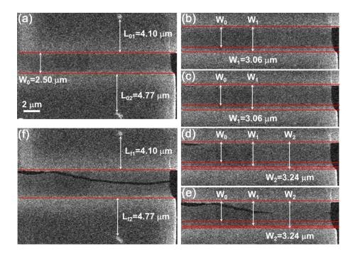
**Figure S2.** The whole process of the *in situ* SEM tensile test of the thicker  $MoS_2$  membrane in Figure 2: (a) before the test, (b) before the initiation of the crack, (c) initiation of a crack, (d) before the sudden expansion of the crack, (e) before fracture, (f) after fracture.
