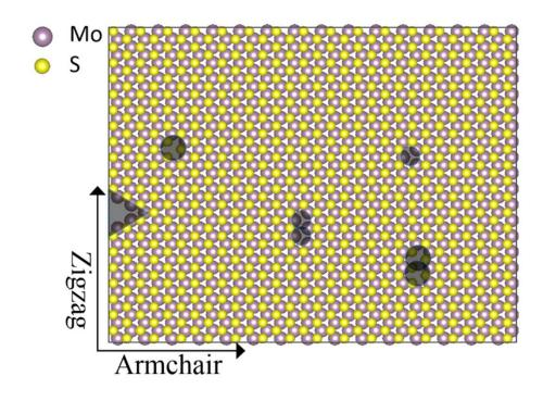
Figure S4. Defect arrangement for  $MoS_2$  nanosheets in MD simulation.
