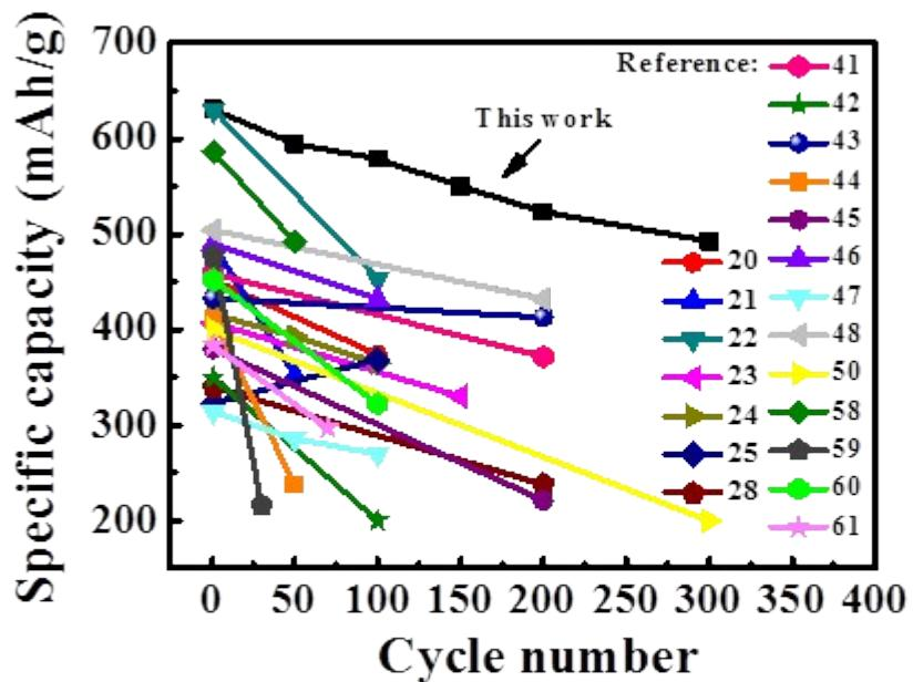
**Figure S9.** Cyclic stability comparison of proposed  $\text{SnO}_2/\text{CMK}-8$  electrode and state-of-the-art  $\text{SnO}_2$ -based NIB anodes reported in the literature.
