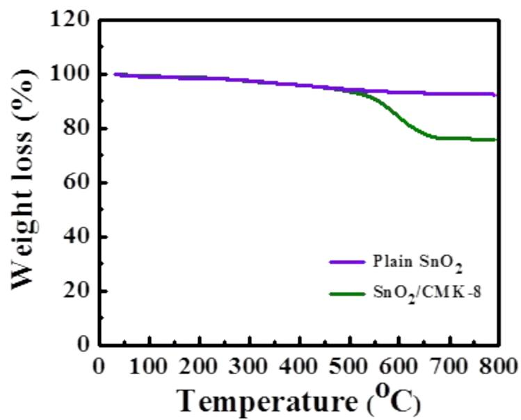
**Figure S6.** TGA data of plain SnO<sub>2</sub> and SnO<sub>2</sub>/CMK-8 samples recorded under air with heating rate of 5 °C min<sup>-1</sup>.
