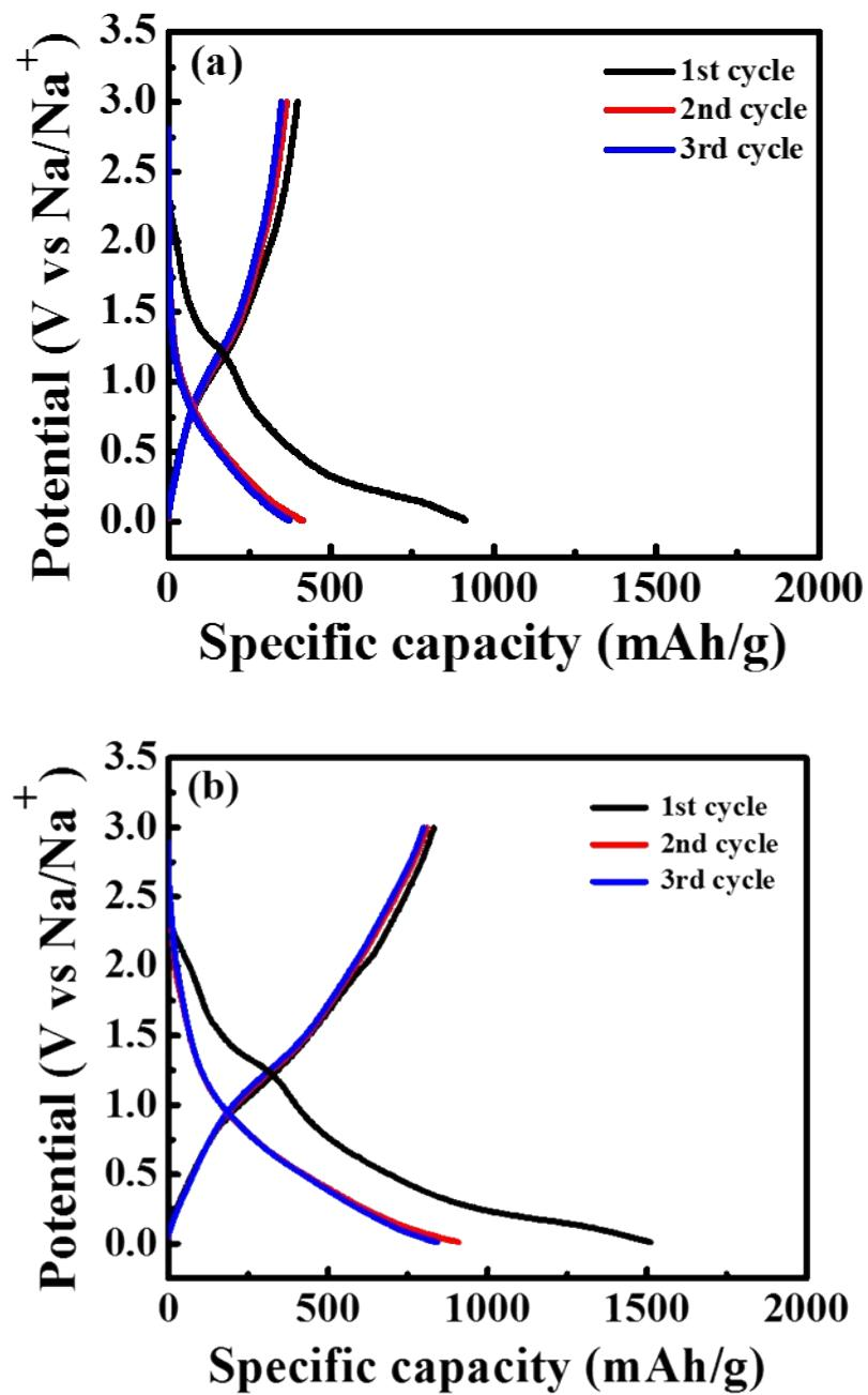
**Figure S4.** Initial three charge–discharge cycles of (a) plain  $\text{SnO}_2$  and (b)  $\text{SnO}_2/\text{CMK-8}$  electrodes measured at rate of  $20 \text{ mA g}^{-1}$ .
