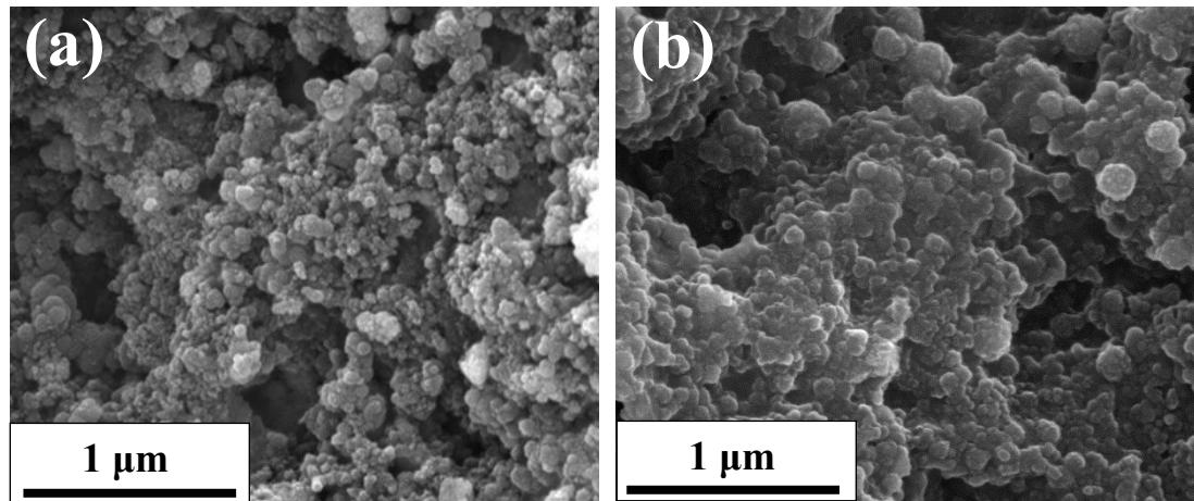
**Figure S11.** SEM images of  $\text{SnO}_2/\text{CMK-8}$  electrode (a) before and (b) after 300 charge–discharge cycles.
