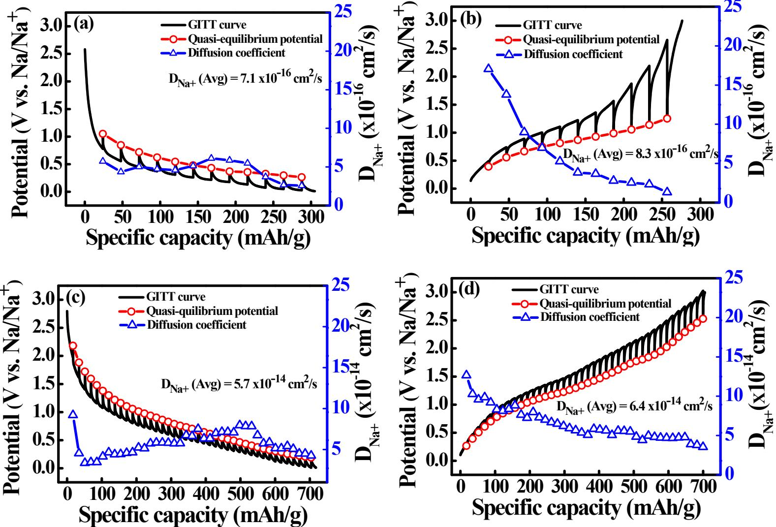
**Figure S8.** Quasi-equilibrium potentials and Na diffusion coefficients measured by GITT for (a, b) plain SnO<sub>2</sub> and (c, d) SnO<sub>2</sub>/CMK-8 electrodes. Data were recorded with a series of current pulses of 50 mA g<sup>-1</sup> for 20 min and 3 h relaxation at each interval.
