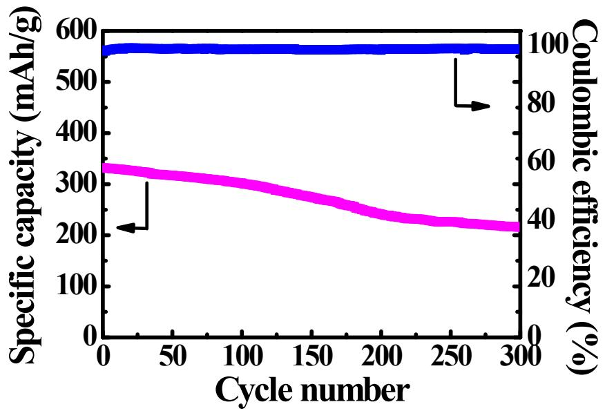
**Figure S10.** Cycling stability data of  $\text{SnO}_2/\text{CMK-8}$  electrode measured at charge–discharge rate of  $2000 \text{ mA g}^{-1}$ .
