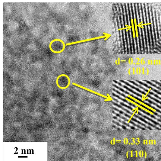
**Figure S1.** High-resolution TEM image of SnO<sub>2</sub>/CMK-8 sample.
