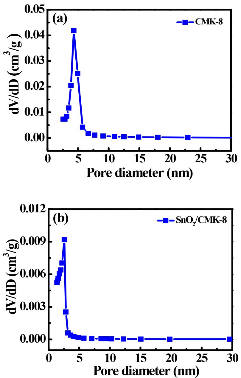
**Figure S2.** Pore size distribution data of (a) CMK and (b)  $\text{SnO}_2/\text{CMK-8}$ .
