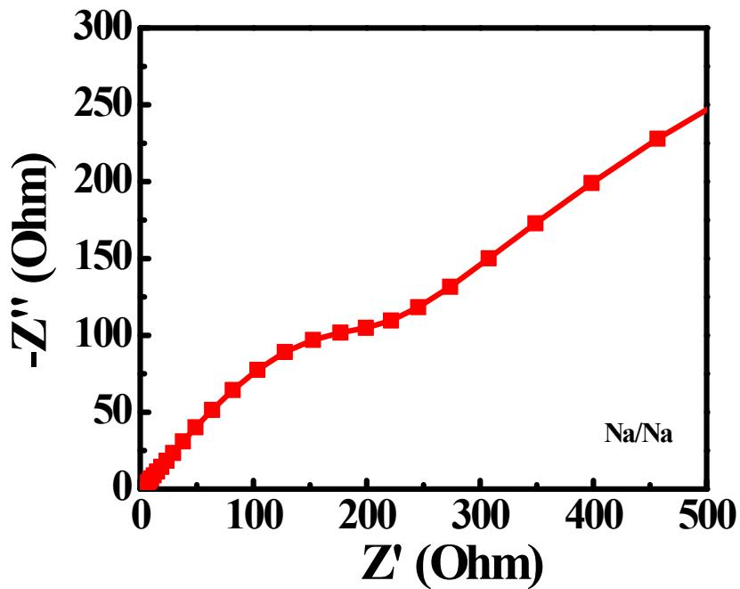
**Figure S7.** EIS data of Na/Na symmetric cell. The fitted  $R_{ct}$  value is  $\sim 400\Omega$ , which is the sum of charge transfer resistances at both Na electrodes. This indicates that resistance at each Na electrode is  $\sim 200 \Omega$ .
