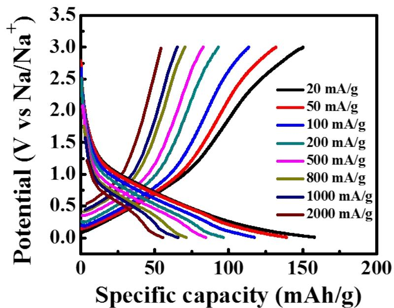
**Figure S5.** Charge–discharge curves of plain CMK-8 electrode recorded at various rates.
