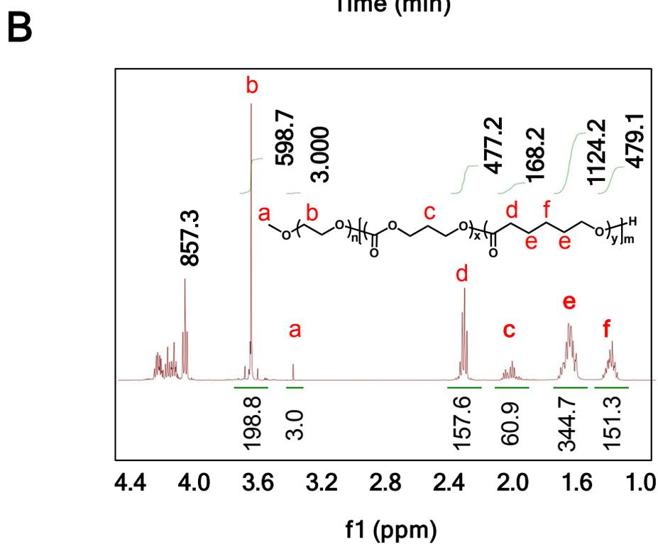
**Figure S1. Characterization of PEG(2k)-*b*-TCL(11.2k) copolymer.** (A) GPC-MALS and (B)  $^1\text{H}$ -NMR spectrum of the copolymer in  $\text{CDCl}_3$ . Distinguishable  $^1\text{H}$  peaks are labeled and assigned to protons in the chemical structure.
