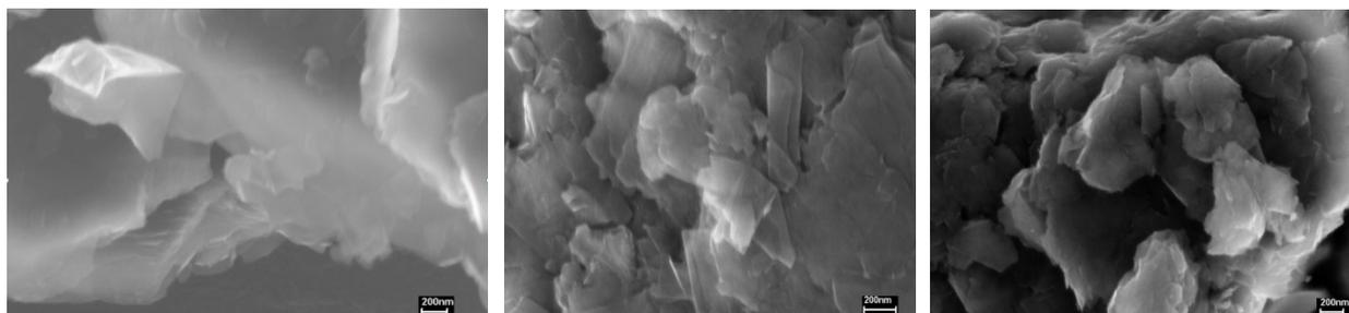
Figure S1: SEM images showing the changes in the dimensions of graphite platelets upon ball-milling. Pristine graphite (left), G5h (center) and G20h (right). The unit of length shown is 200 nm. For images with different zoom refer to<sup>1</sup>.
