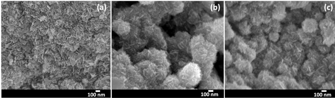
**Fig. S5** FE-SEM images of (a) MnO<sub>2</sub> nanosheet powder, (b) MnO<sub>2</sub> nanosheets on positive electrode after cycling stability, and (c) MnO<sub>2</sub> nanosheets on negative electrode after cycling stability.
