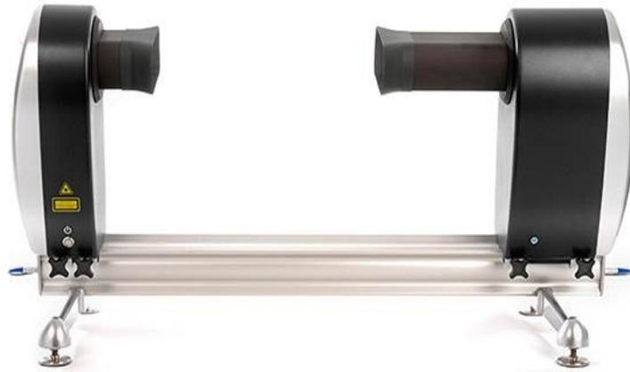
**Figure S3.** Photograph of Spraytec laser diffractometer used for the measurement of droplet sizes.
