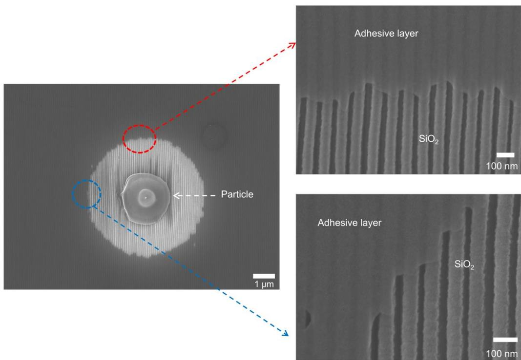
**Fig. S5** SEM images of Au/adhesive/SiO<sub>2</sub> layers after peel-off test.
