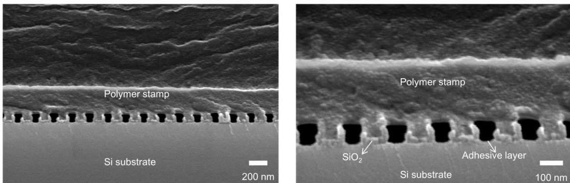
**Fig. S4** SEM images of Si/adhesive/SiO<sub>2</sub> structure after peel-off test at different magnifications.
