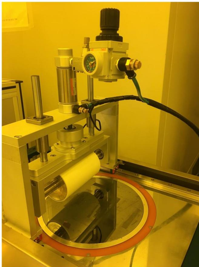
**Fig. S9** Photograph of roll-to-plate transfer system.
