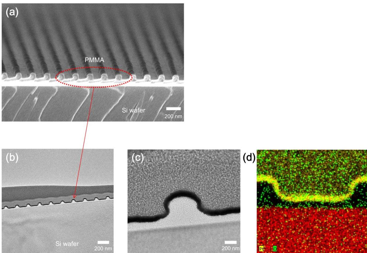
**Fig. S1** Transfer printing using PMMA as adhesive. (a) SEM image of imprinted PMMA after transfer procedure, (b,c) TEM images of imprinted PMMA, (d) EDS image of imprinted PMMA.
