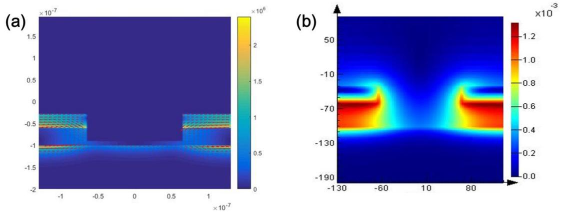
Fig. S7 Simulation results of electromagnetic field for meta-surface with period of 260 nm and diameter of 130 nm (a) current density vector at wavelength of 545 nm (b) magnetic field intensity at wavelength of 545 nm.
