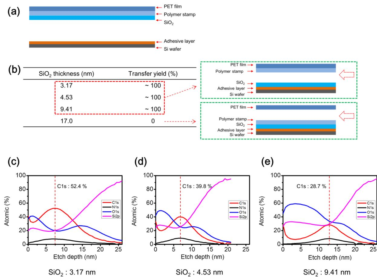
**Fig. S2** Schematic diagrams of nanotransfer process depending on thicknesses of SiO<sub>2</sub> and XPS spectra (a) schematic diagram of prepared sample, (b) measured SiO<sub>2</sub> thickness, transfer yield and schematic diagrams after transfer procedure, based on the SiO<sub>2</sub> thickness (dotted arrow indicates the detached interface), (c, d, e) XPS spectra for different thicknesses of SiO<sub>2</sub>.
