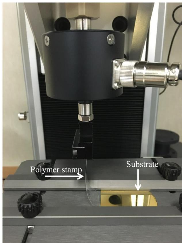
**Fig. S3** A photograph of peel test set-up and peel force measurement.
