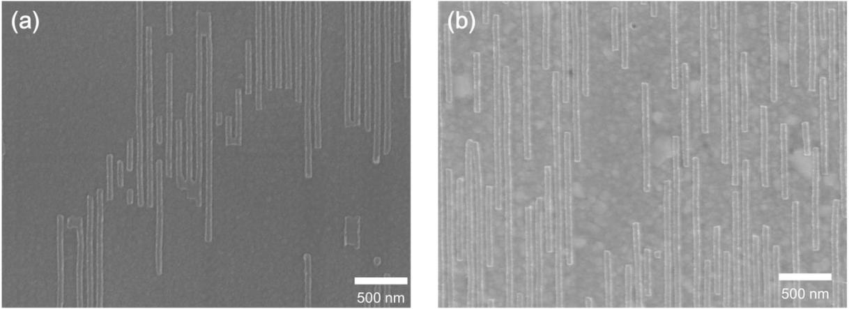
**Fig. S6** SEM images of samples with transferred SiO<sub>2</sub> lines on the (a) Al substrate and (b) Ag substrate after peel test.
