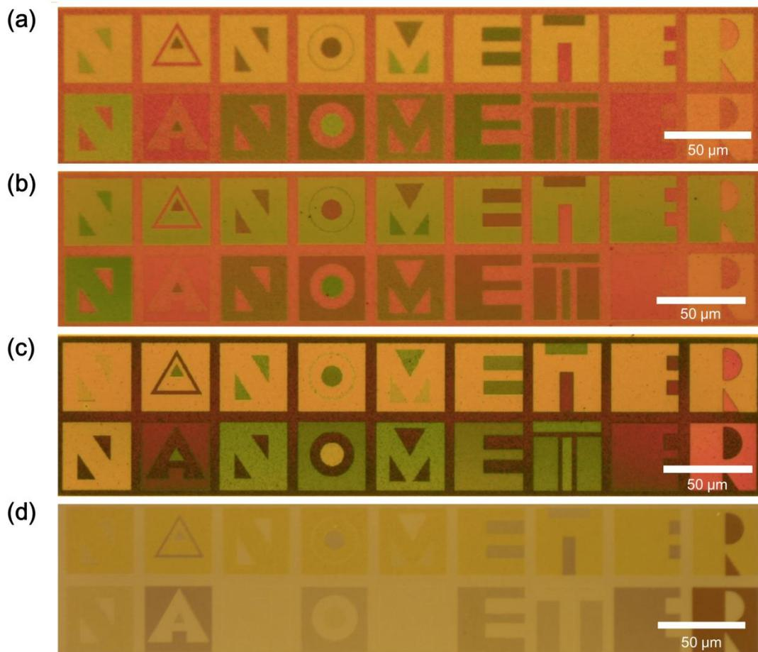
**Fig. S8** Optical microscope images of meta-surfaces illuminated with halogen lamp. Fabricated meta-surface using (a) Ag, (b) Au, (c) Au and PMMA spin coating, and (d) Al.
