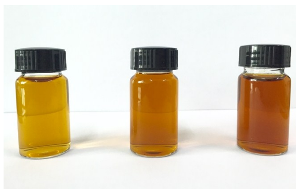
Fig. S2 Photograph of aqueous dispersions GO-FA, GO-FA/Py- \gamma -CD, and GO-FA/Py- \gamma -CD/ \text{C}_{60} (from left to right, 30 \mu\text{g}/\text{mL} )
