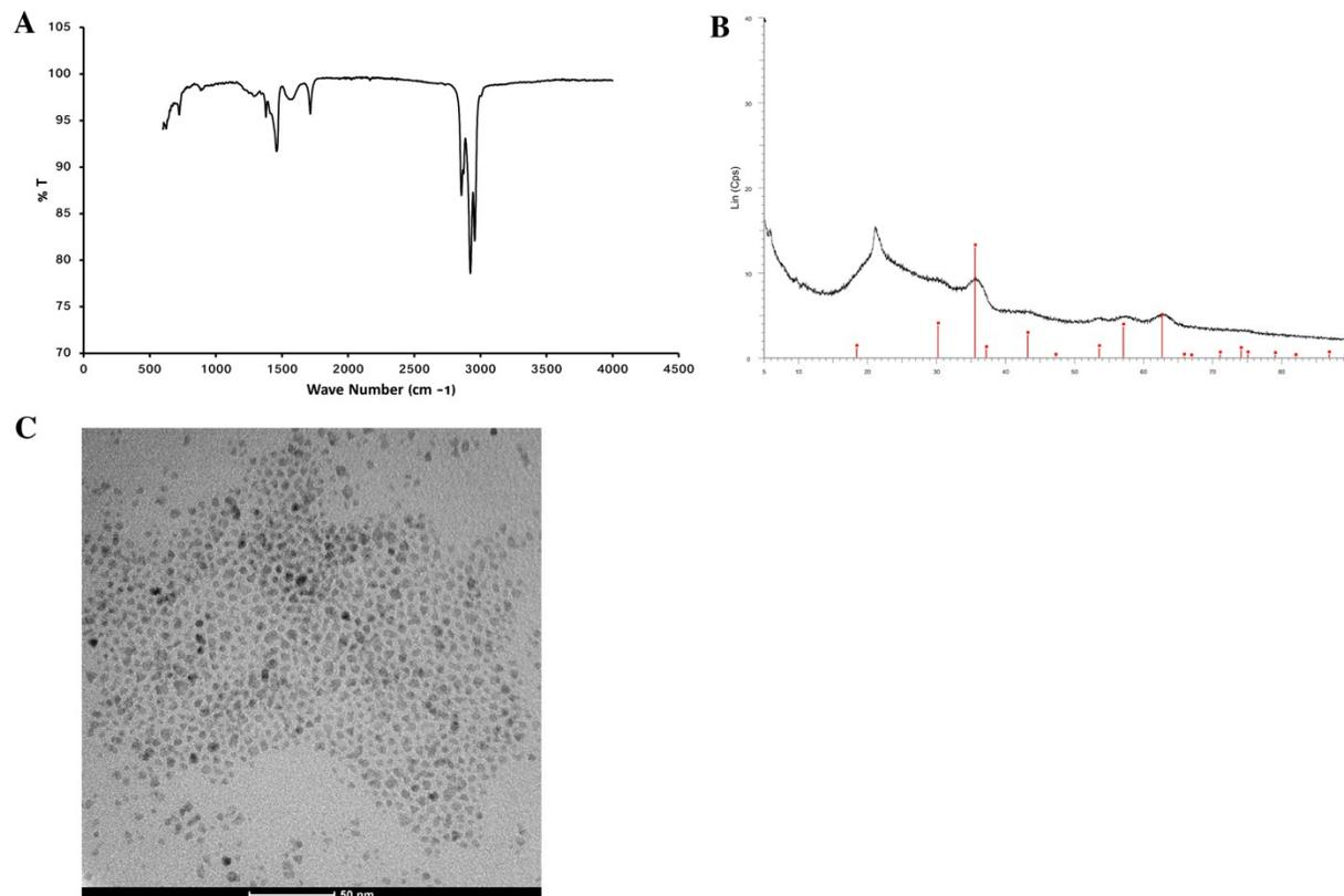
**Supplemental Figure S1. Characterization of IONP.** (A) Fourier Transform Infrared Spectroscopy of oleic-acid coated IONP show characteristics peaks at 2964, 2932, 2874, 1629 and 1469 cm<sup>-1</sup>. (B) X-ray diffraction. (C) A representative TEM image of IONP particles. Scale bar = 50 nm.
