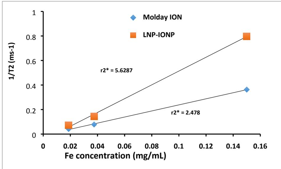
**Supplementary Figure S6.** Spin-spin  $1/T_2^*$  relaxation rates of LNP-IONP (orange) is compared to commercially available T2 contrast agent Molday ION (blue) at different iron (Fe) concentrations. Transverse relaxivity rates  $r_2^*$  of LNP-IONP and Molday ION were obtained by measuring calculating the slopes.
