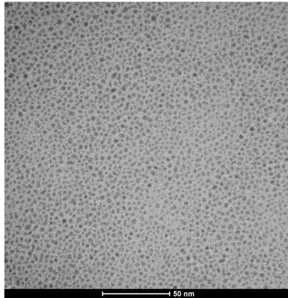
**Supplemental Figure S2. Representative TEM image of gold nanoparticles.** 10 $\mu$ L of GNP solution was pipetted onto a copper grid and imaged using a TEM at 200 kV acceleration voltage. Images were acquired using a high-speed AMT 2K side mount CCD camera.
