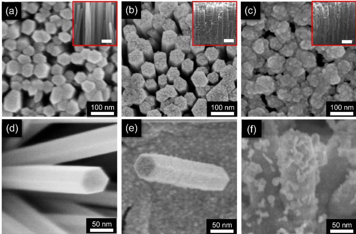
**Figure S1.** SEM images of (a) & (d) ZnO NRs, (b) & (e) binary CuO-ZnO NRs composite, (c) & (f) ternary Ag-CuO-ZnO NRs composite. The insets in (a-c) are the cross-section images of the corresponding products. The scale bars of the insets (a-c) are 50 nm.
