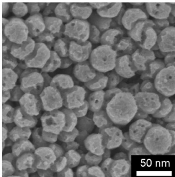
**Figure S10.** The SEM image of ternary Ag-CuO-ZnO NRs after the 20<sup>th</sup> photocatalytic cycle degradation.
