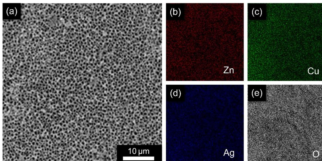
**Figure S3.** Elemental mapping results of the ternary Ag-CuO-ZnO NTs composite.
