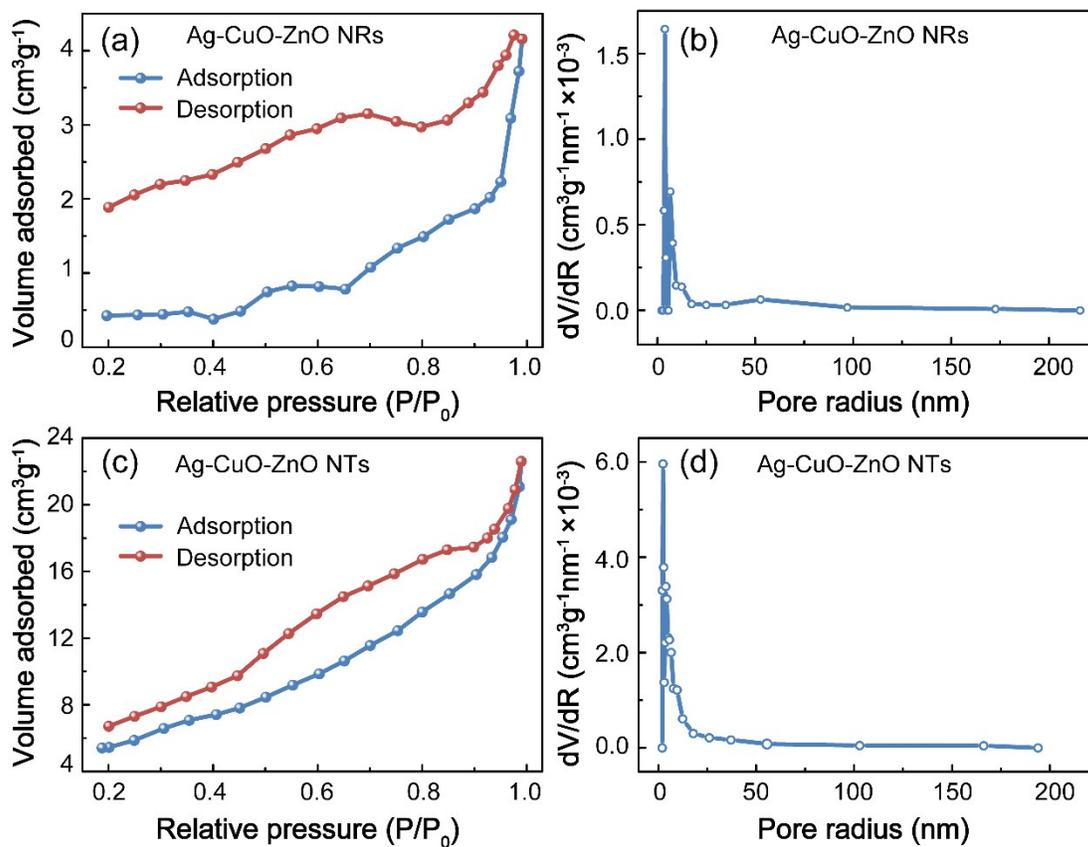
**Figure S7.** BET of (a), (b) Ag-CuO-ZnO NRs, and (c), (d) Ag-CuO-ZnO NTs.
