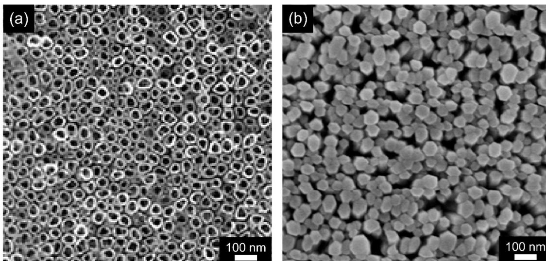
**Figure S2.** SEM images of large-area (a) ZnO NTs and (b) ZnO NRs.
