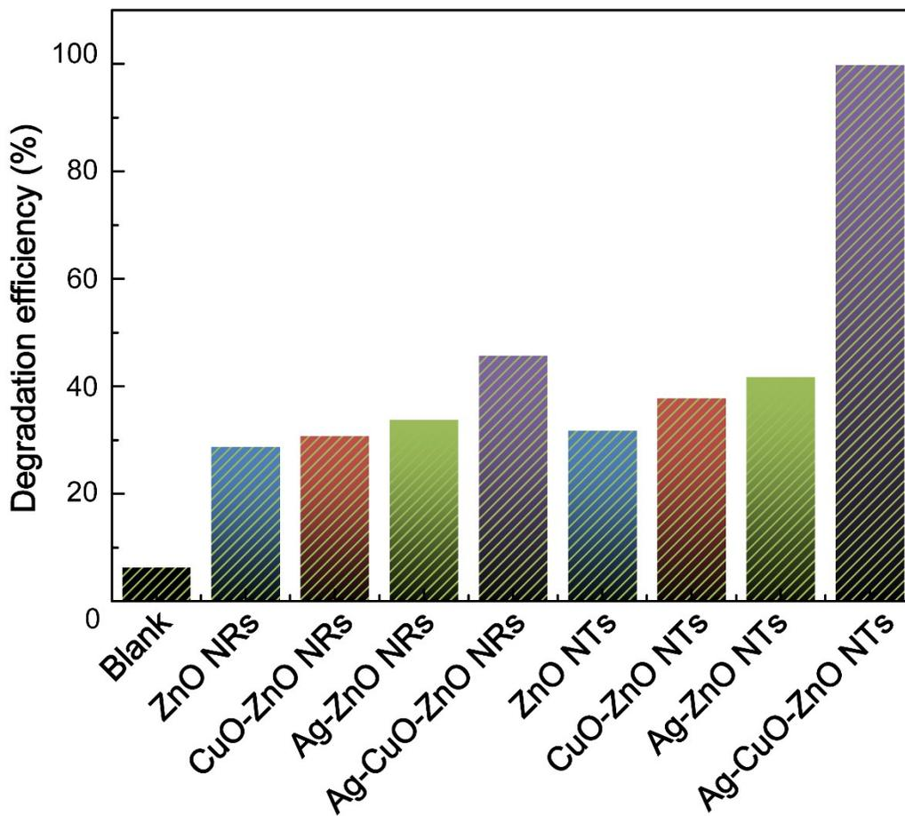
**Figure S4.** Different photocatalysts to degrade MO, including ZnO NRs, CuO-ZnO NRs, Ag-ZnO NRs, Ag-CuO-ZnO NRs, ZnO NTs, CuO-ZnO NTs, Ag-ZnO NTs and Ag-CuO-ZnO NTs.
