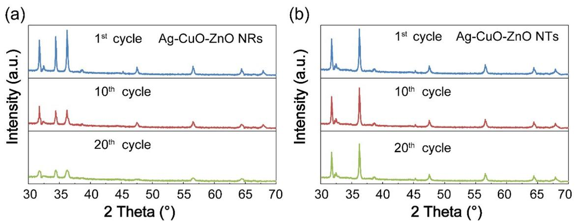
**Figure S11.** XRD patterns of (a) Ag-CuO-ZnO NRs and (b) Ag-CuO-ZnO NTs after the 1<sup>st</sup>, 10<sup>th</sup> and 20<sup>th</sup> photocatalytic cycle degradation.
