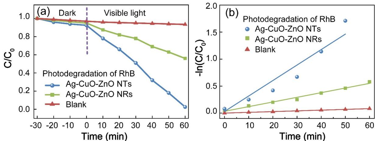
**Figure S6.** (a) Time-dependent photodegradation efficiency of RhB without photocatalysts and in the presence of the ternary composites based on ZnO NTs and NRs. (b) The corresponding plots of  $-\ln(C_t/C_0)$  versus irradiation time.
