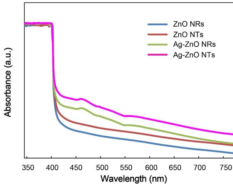
**Figure S9.** Absorption spectra of the bare ZnO NRs, bare ZnO NTs, Ag-ZnO NRs and Ag-ZnO NTs.
