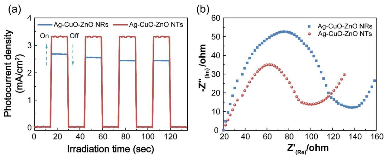
**Figure S8.** (a) Photocurrent density and (b) electrochemical impedance spectroscopy (EIS) Nyquist plots for the ternary ZnO NRs and ZnO NTs-based composites
