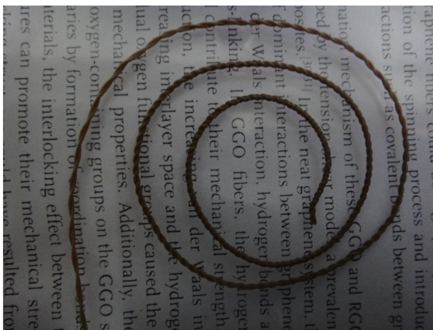
Figure S3. Photograph of double-plyed GO fibers with a continuous alteration of helix angle produced by a double-hole spinneret with a variable rotation speed. The alterable structure of GO fiber indicates the excellent controllability of our fabrication method.
