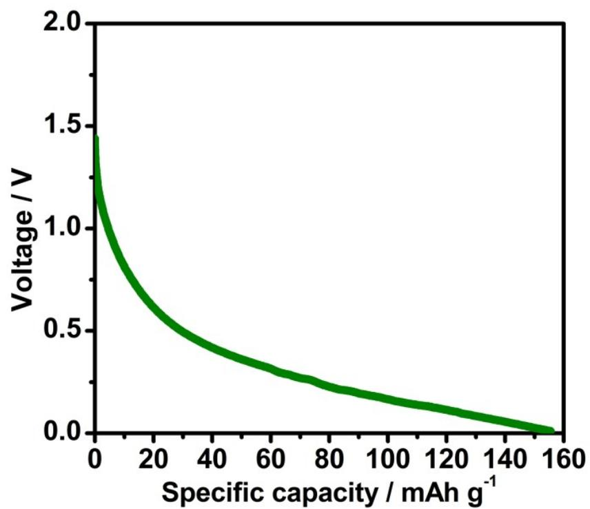
**Figure S13.** First discharge curve of the TiO<sub>2</sub>-B nanowires in Mg ion batteries.
