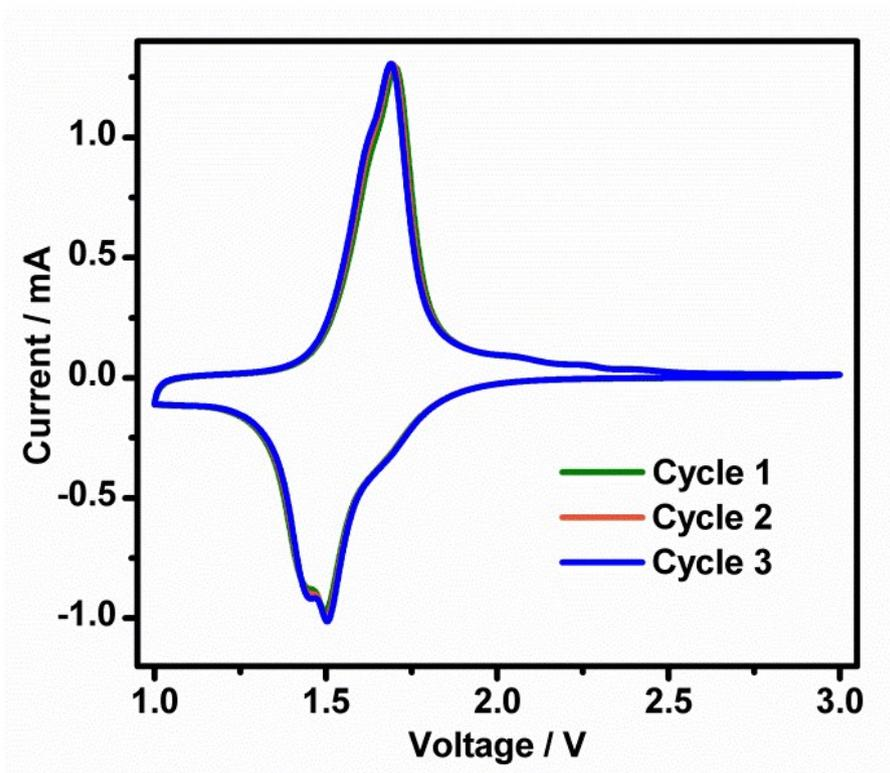
**Figure S7.** CV of the TiO<sub>2</sub>-B nanowires in a 1.0 M LiPF<sub>6</sub> electrolyte dissolved in ethylene carbonate (EC) and dimethyl carbonate (DMC) (EC : DMC = 3 : 7).
