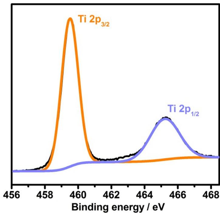
**Figure S11.** Ti 2*p* XPS pattern of the TiO<sub>2</sub>-B nanowires.
