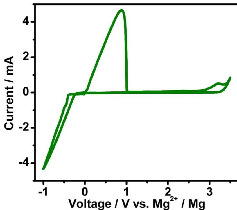
**Figure S2.** CV curve from the three-electrode cell using the APC/THF electrolyte, Pt as the working electrode and Mg as the reference and counter electrodes.
