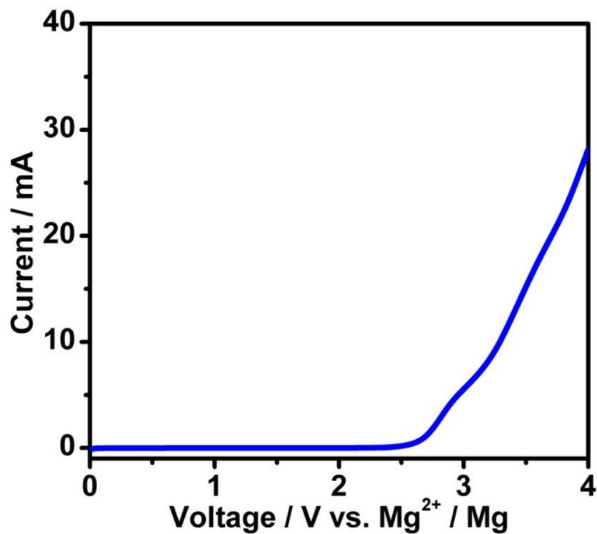
**Figure S3.** LSV curve obtained from a coin cell using the APC/THF electrolyte, SSF as the working electrode and Mg as the counter electrode.
