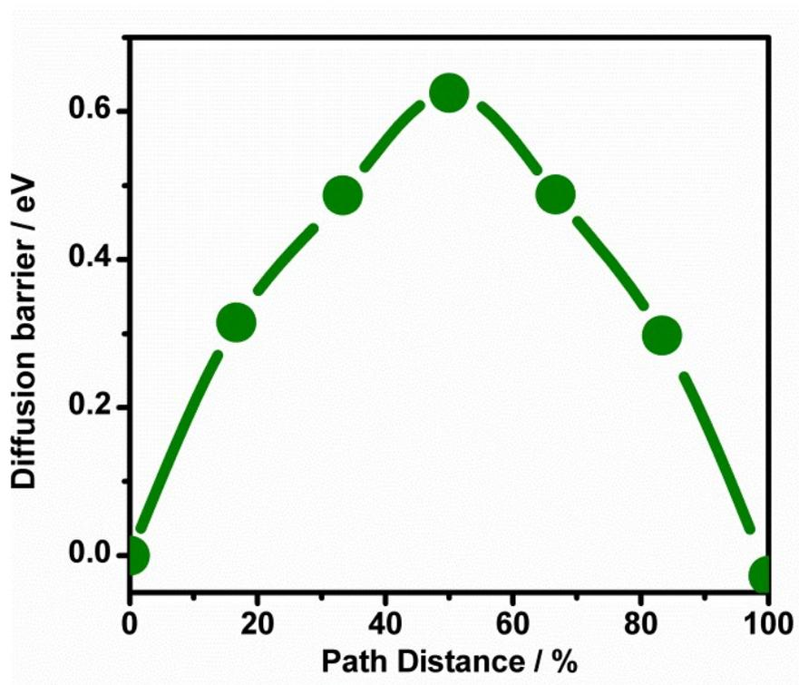
**Figure S8.** Calculated diffusion barrier for Mg<sup>2+</sup> ions in TiO<sub>2</sub>-B.
