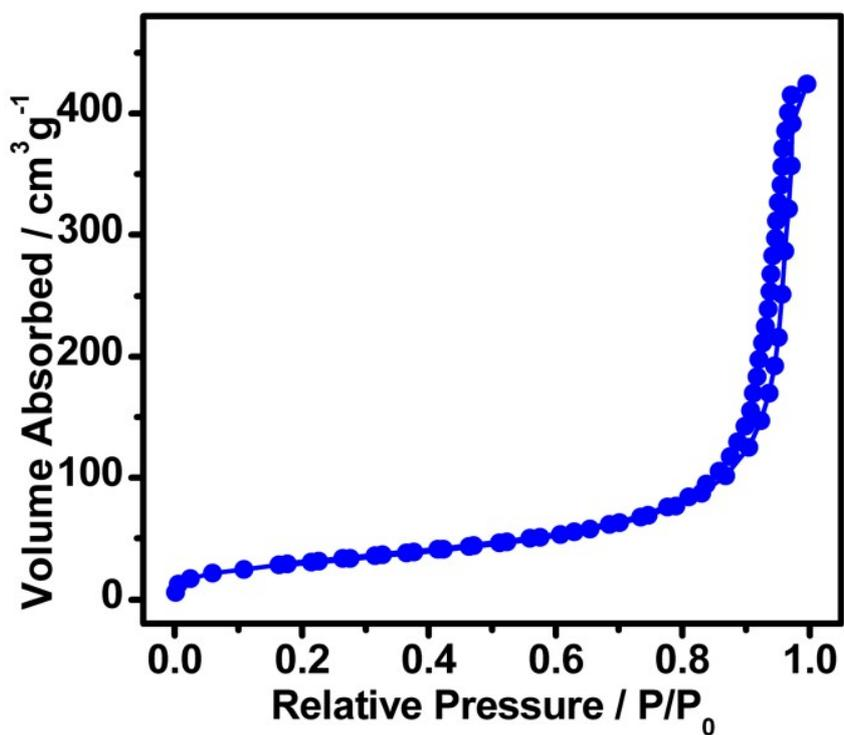
**Figure S1.** Nitrogen adsorption-desorption isotherms of the TiO<sub>2</sub>-B nanowires.
