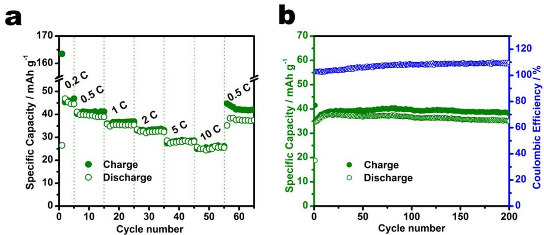
**Figure S5.** Rate performance (a) and charge-discharge cycling performance at 2C rate (b) for the reference TiO<sub>2</sub>-B nanowire sample.
