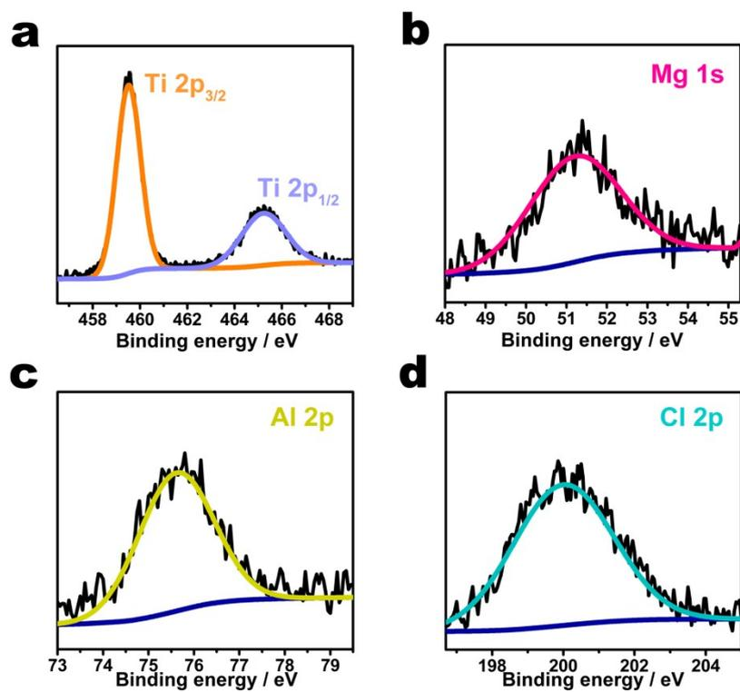
**Figure S12.** (a) Ti 2*p*, (b) Mg 1*s*, (c) Al 2*p*, and (d) Cl 2*p* XPS patterns of the TiO<sub>2</sub>-B electrode held at the open-circuit voltage (OCV) for 36 h.
