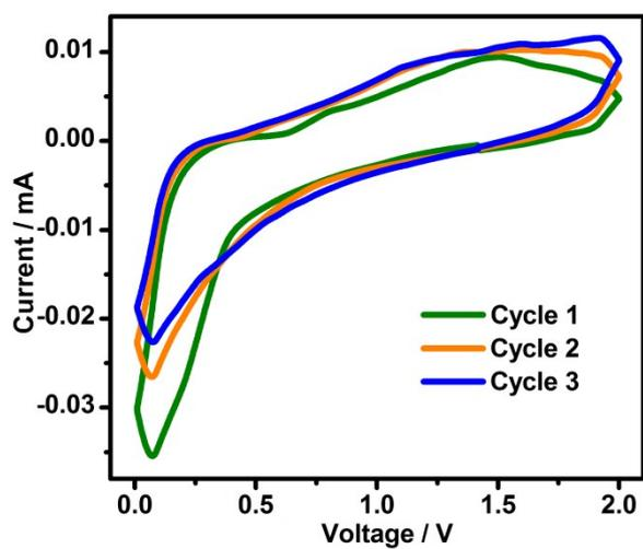
**Figure S6.** CV curves of the TiO<sub>2</sub>-B nanowires at a scanning rate of 0.05 mV·s<sup>-1</sup>.
