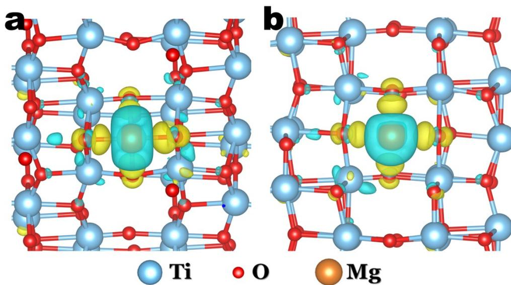
**Figure S10.** The charge difference isosurfaces of Mg<sup>2+</sup> ion adsorption on the site A2 (left) and C (right) sites of TiO<sub>2</sub>-B (-110) surface, respectively; isosurface level is set to 0.005 e/Å<sup>3</sup>.
