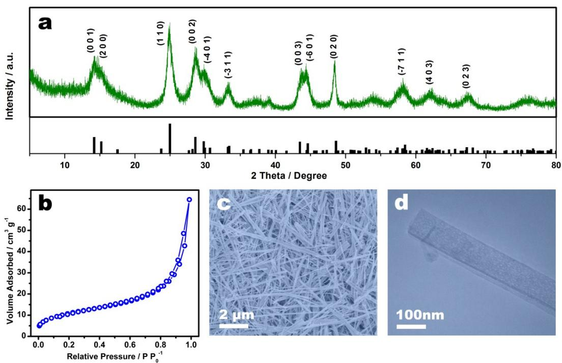
**Figure S4.** XRD (a), N<sub>2</sub> adsorption-desorption isotherms (b), SEM (c) and TEM (d) of the reference TiO<sub>2</sub>-B nanowire sample.
