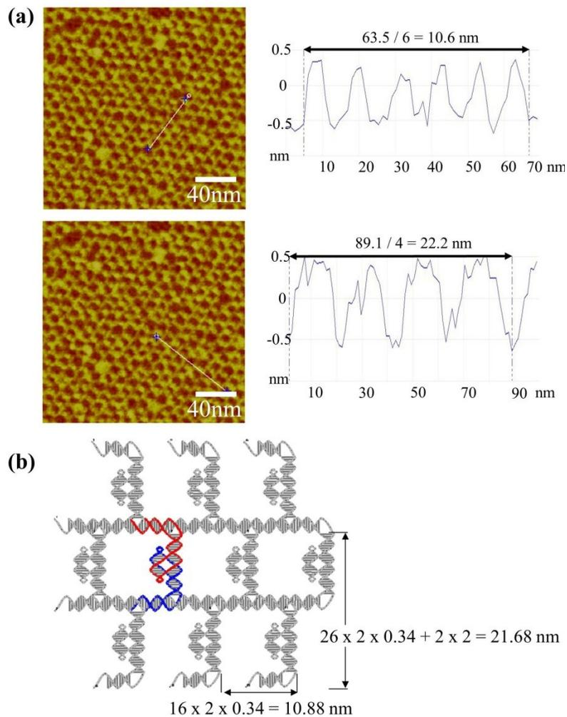
**Figure S2. Section analysis of M2 -- 2D arrays assembled from M1.** (a) The height profiles (right) are along the lines indicated on the AFM images (left). (b) The calculation of the repeating distances.
