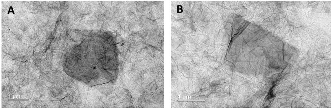
**Fig. S1.** Transmission electron micrograph (TEM) of graphene oxide.
